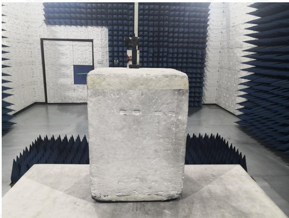
FCC RADIATED EMISSION TEST SETUP ABOVE 1GHZ
