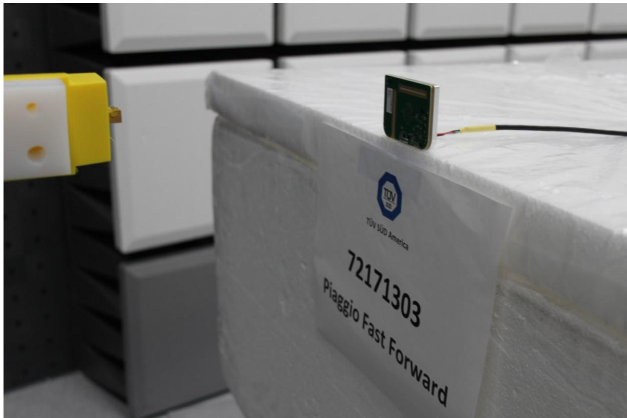
**Radiated Emissions Test Setup (220GHz TO 231GHz)**
