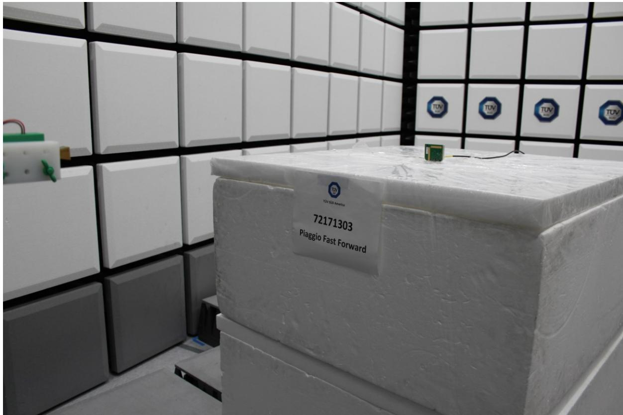
**Radiated Emissions Test Setup (81GHz TO 220GHz)**
