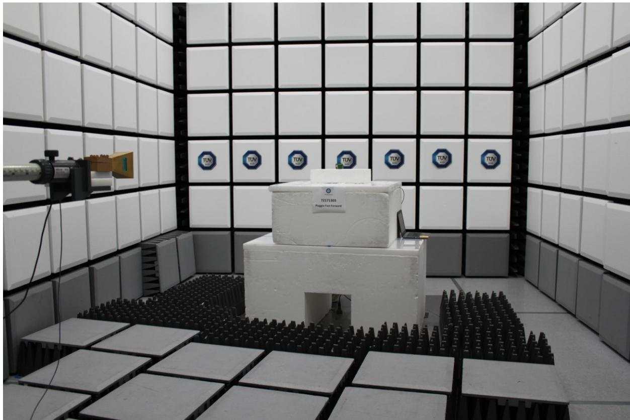
**Radiated Emissions Test Setup (18GHz TO 81GHz)**
