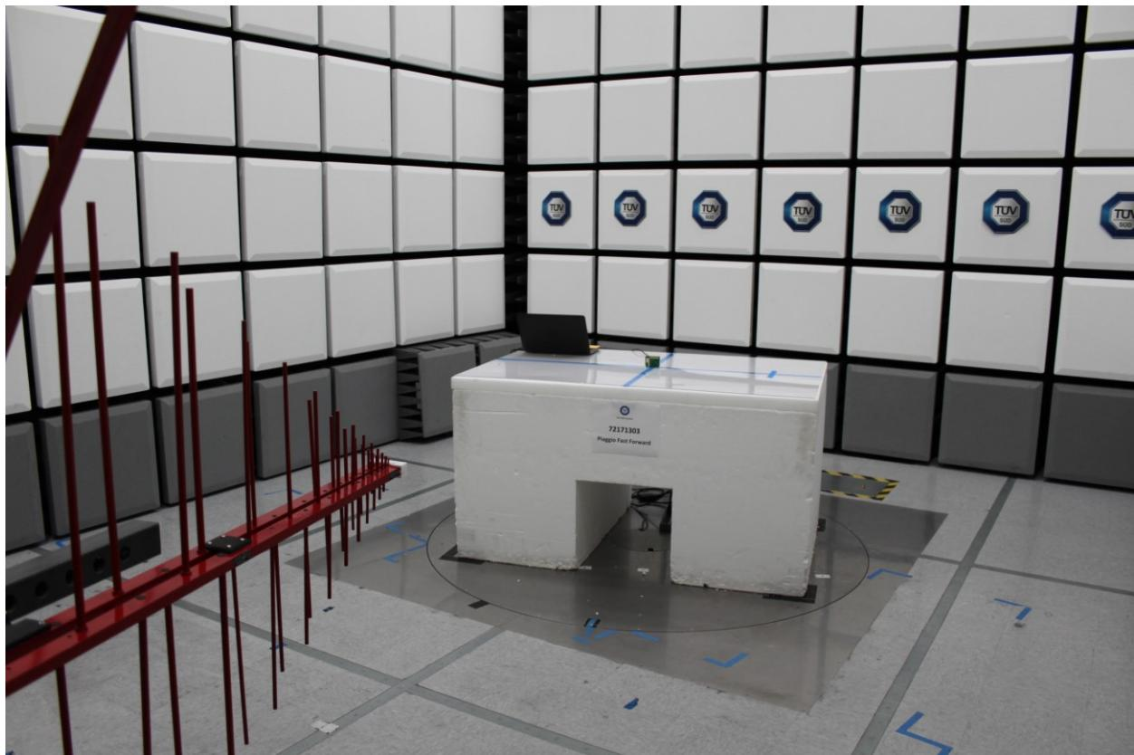
**Radiated Emissions Test Setup (30MHz to 1GHz)**
