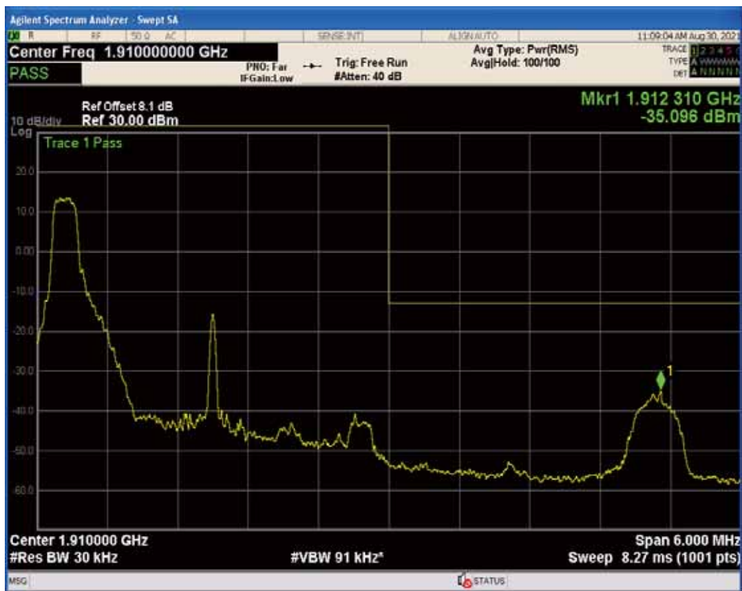
Band2 QAM16 BW=3MHz Channel=19185 RB Size=1 Position=#Max
