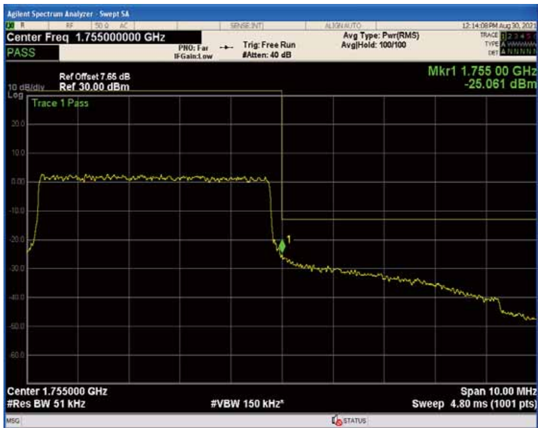
Band4 QAM16 BW=5MHz Channel=20375 RB Size=1 Position=#0
