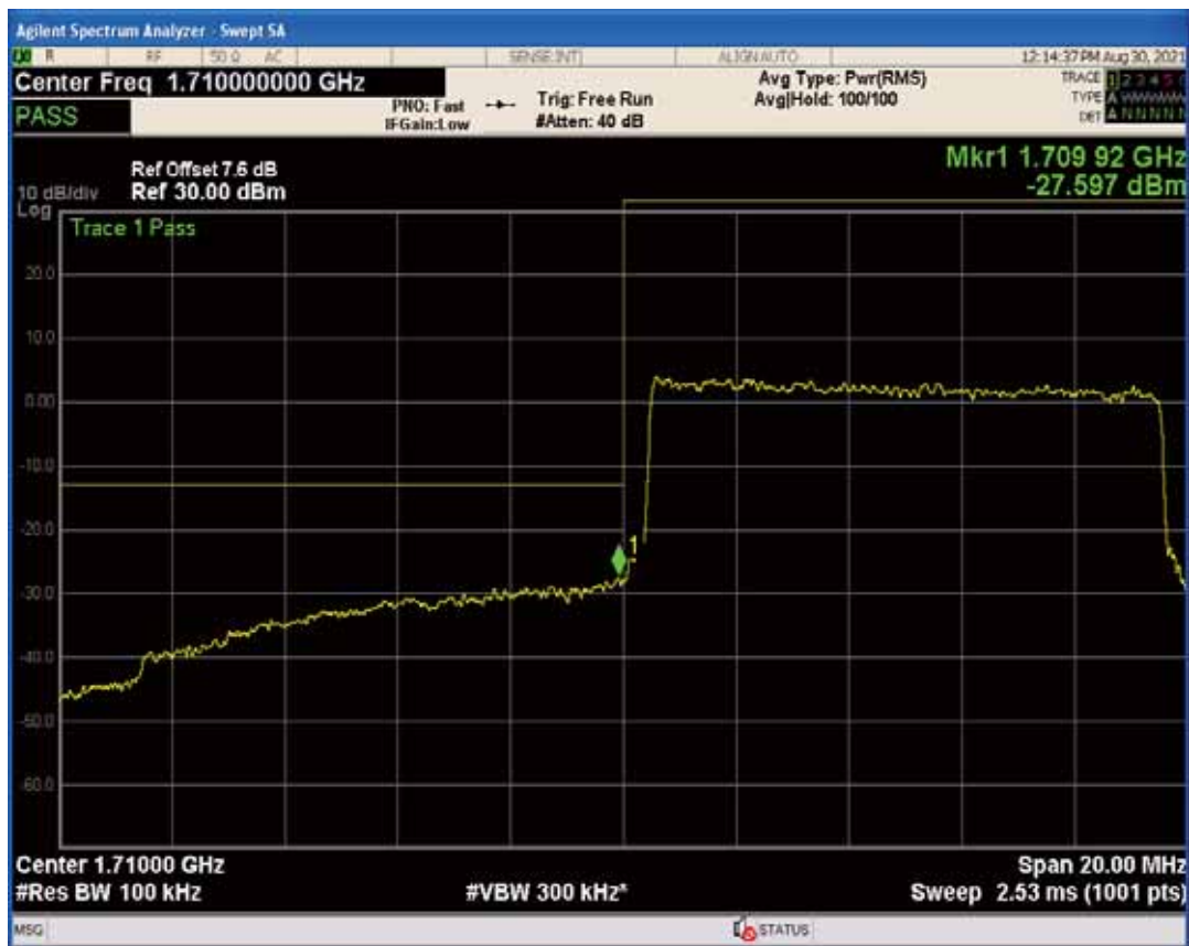
Band4 QAM16 BW=10MHz Channel=20000 RB Size=1 Position=#Max
