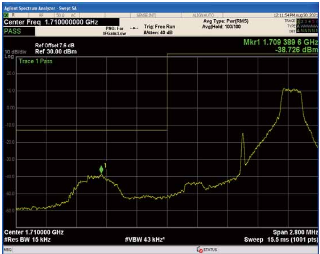
Band4 QPSK BW=1.4MHz Channel=20393 RB Size=1 Position=#0
