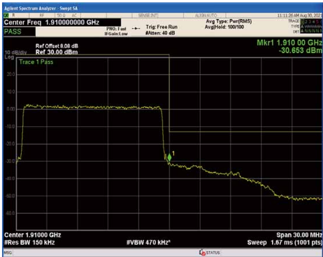
Band2 QAM16 BW=15MHz Channel=19125 RB Size=1 Position=#Max
