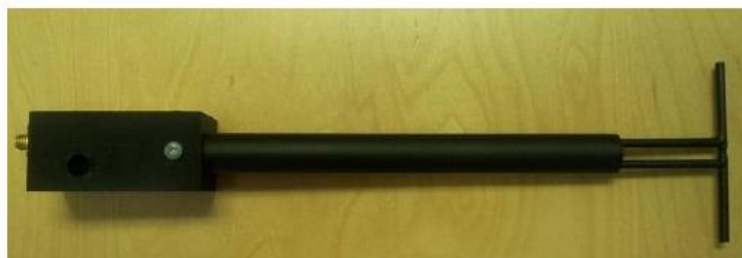
Figure 1 – MVG COMOSAR Validation Dipole
