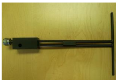
Figure 1 – MVG COMOSAR Validation Dipole
