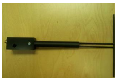
Figure 1 – MVG COMOSAR Validation Dipole
