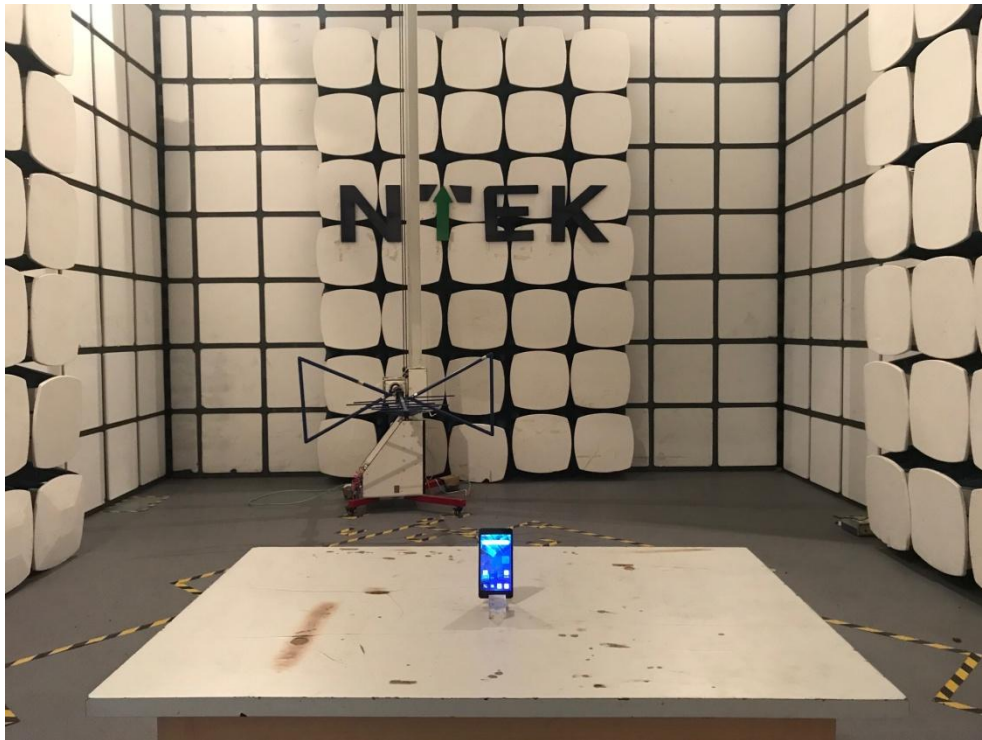
Radiated Measurement Photos(30MHz~1GHz )
