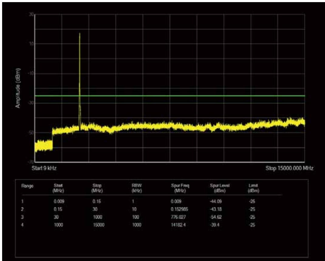
Band7 QPSK BW=20MHz Channel=21100 RB Size=1 Position=#0
