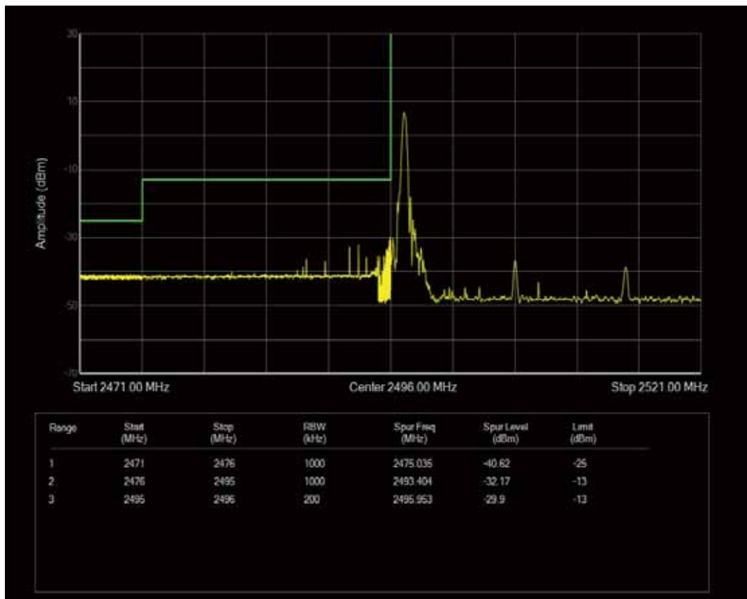
Band41 QAM16 BW=20MHz Channel=39750 RB Size=100 Position=#0
