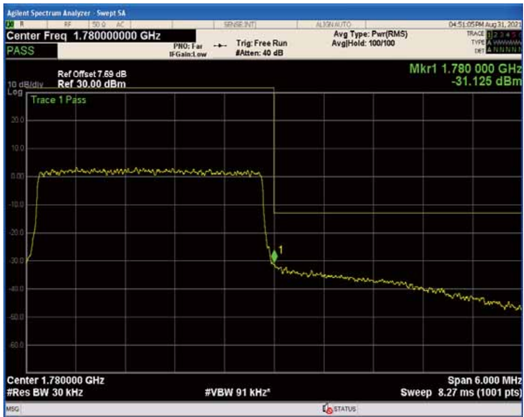
Band66 QPSK BW=5MHz Channel=132647 RB Size=1 Position=#0
