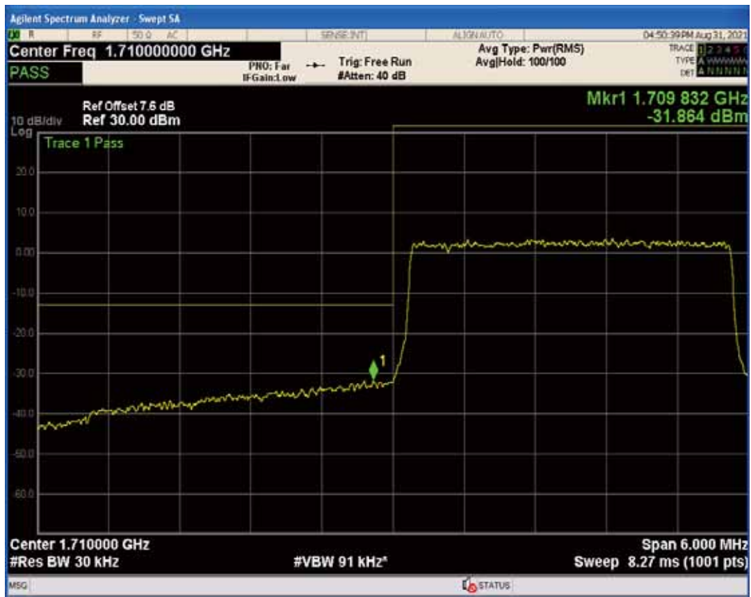
Band66 QPSK BW=3MHz Channel=132657 RB Size=1 Position=#0
