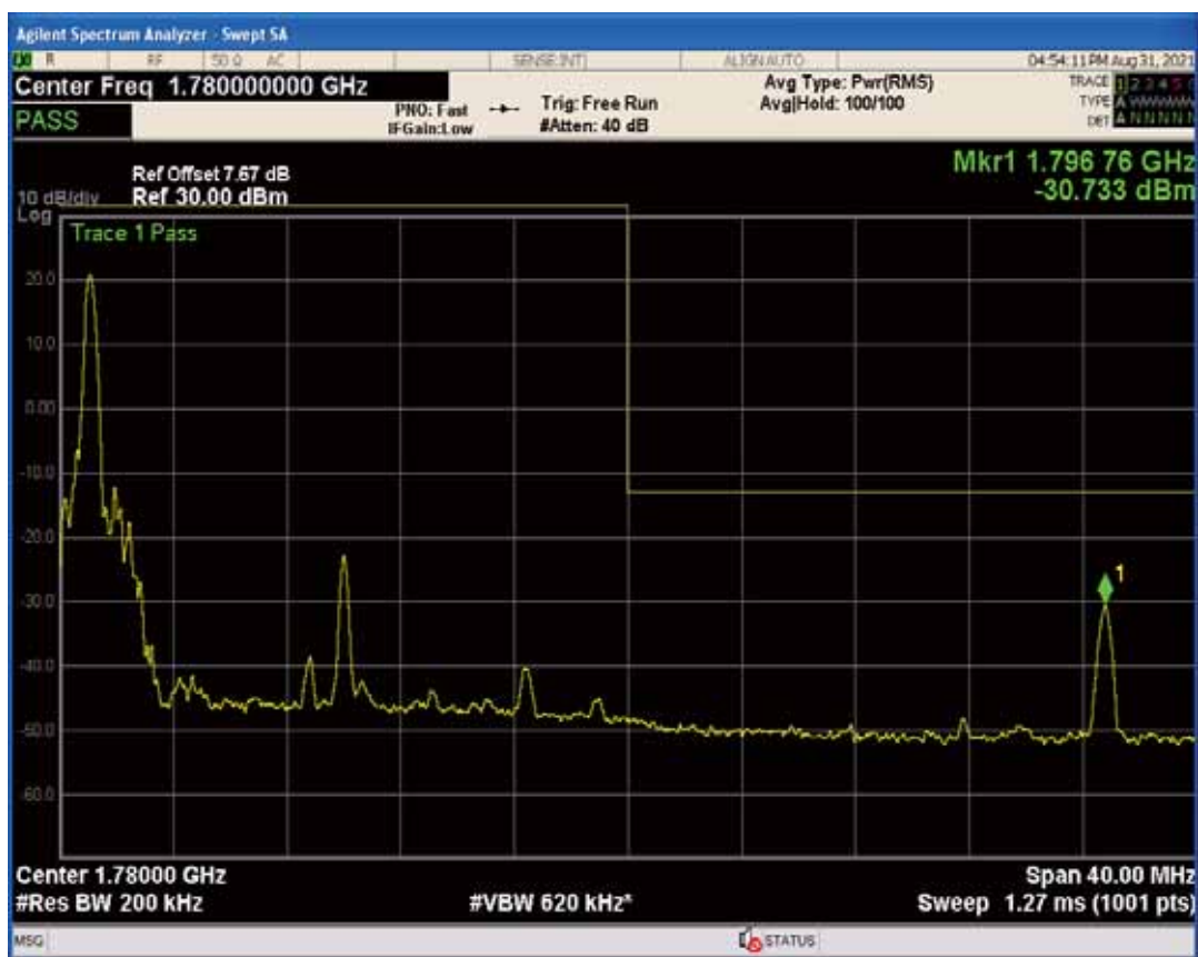
Band66 QAM16 BW=20MHz Channel=132572 RB Size=100 Position=#0
