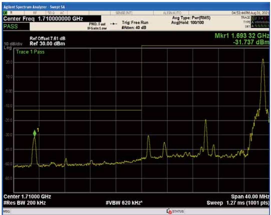
Band66 QAM16 BW=20MHz Channel=132072 RB Size=1 Position=#0
