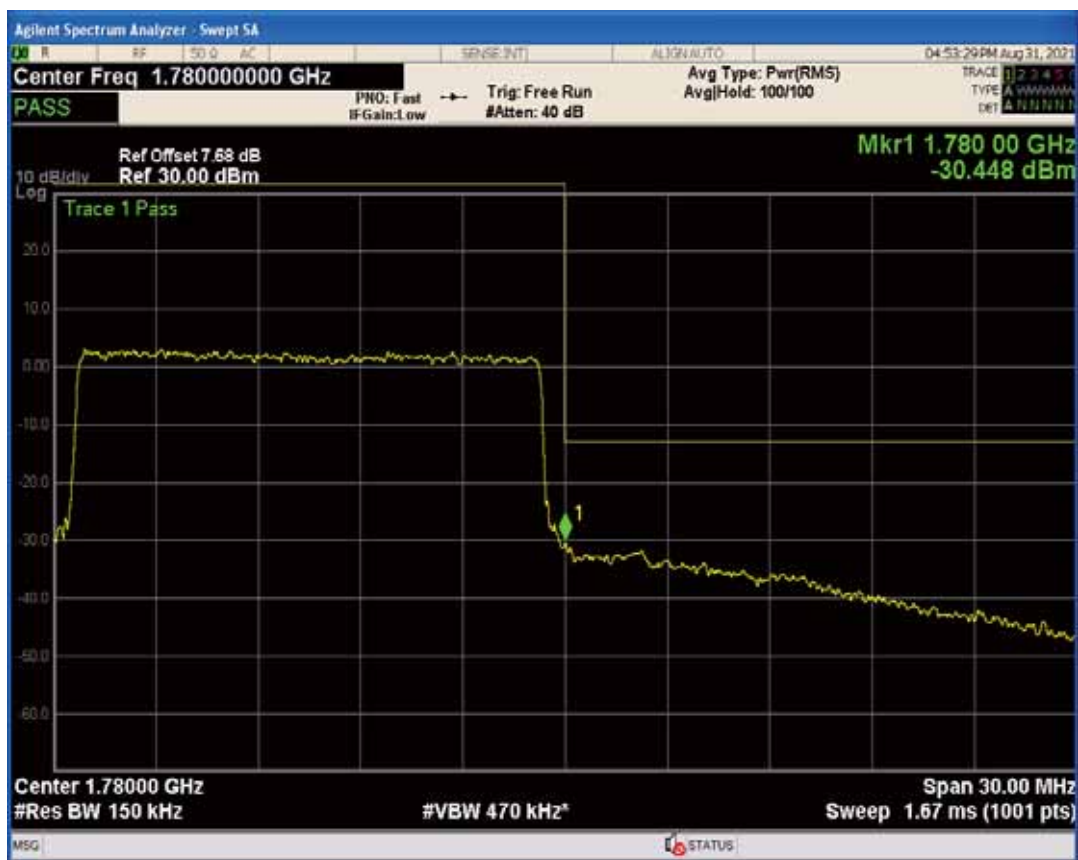
Band66 QAM16 BW=15MHz Channel=132597 RB Size=1 Position=#Max
