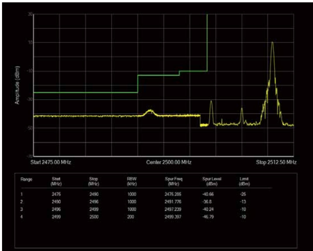
Band7 QAM16 BW=10MHz Channel=20800 RB Size=50 Position=#0
