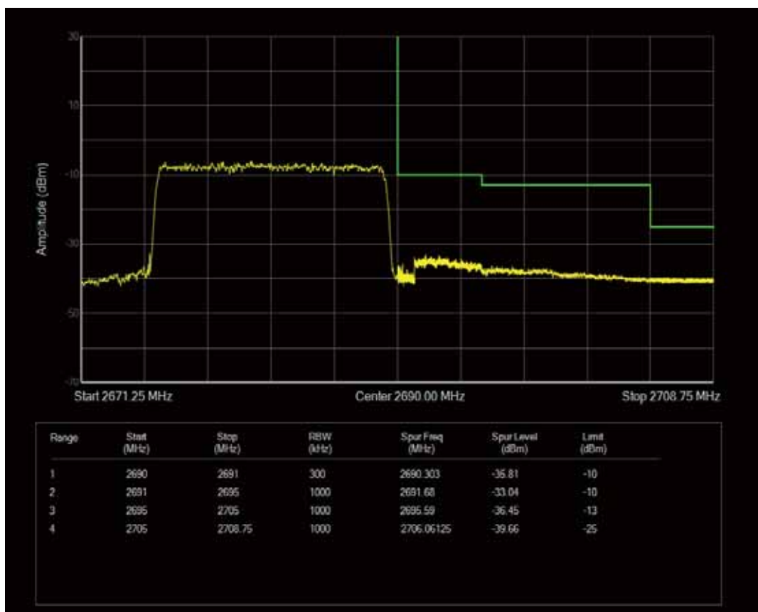
Band41 QPSK BW=15MHz Channel=41515 RB Size=1 Position=#Max
