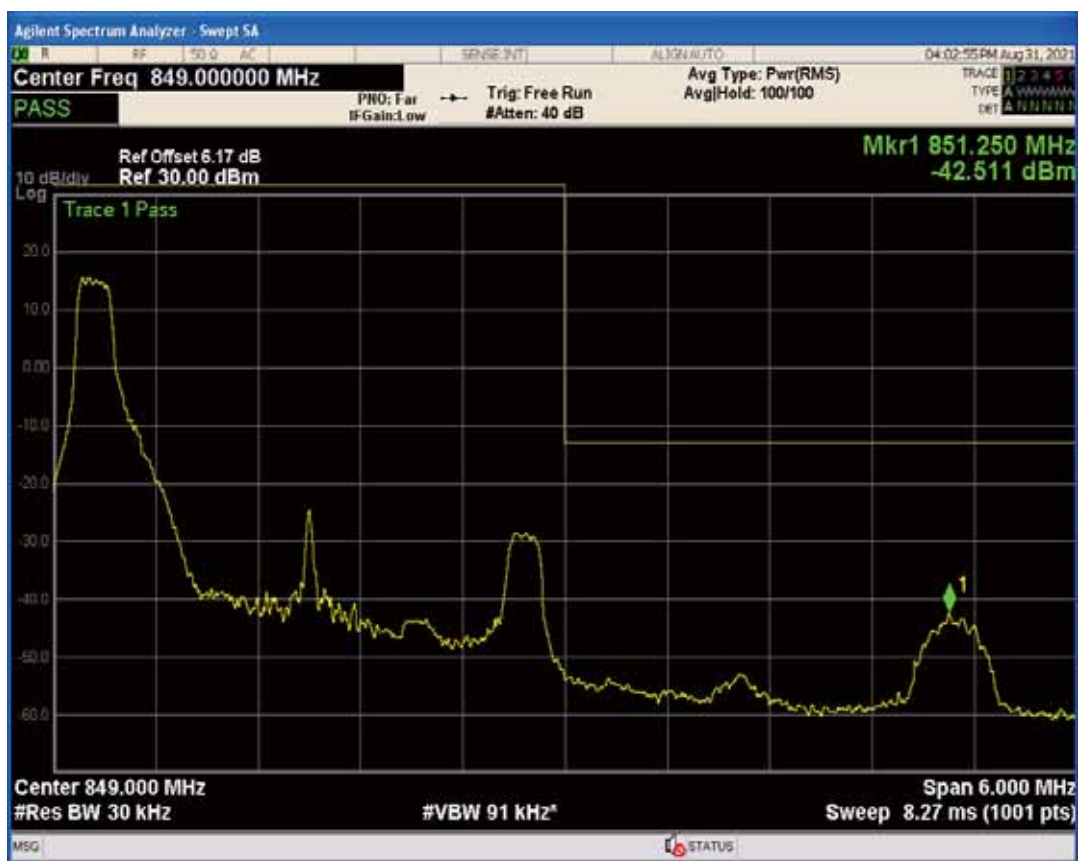
Band5 QAM16 BW=3MHz Channel=20635 RB Size=15 Position=#0
