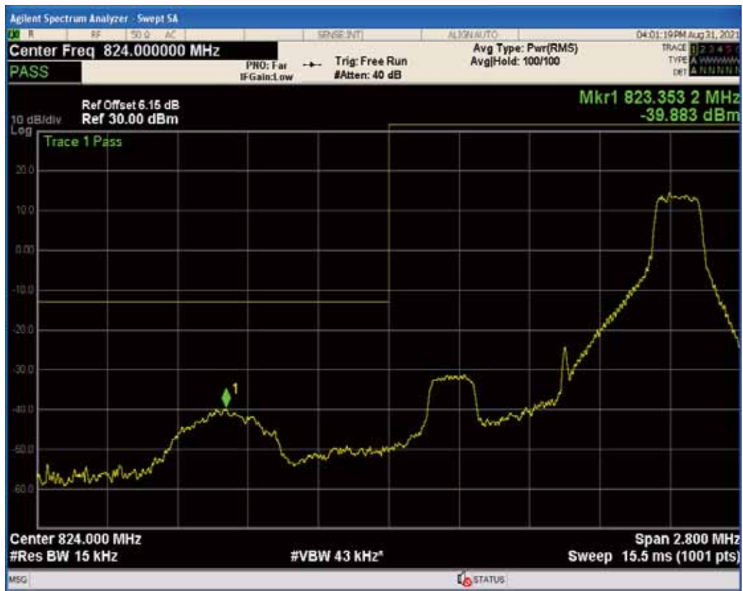
Band5 QPSK BW=1.4MHz Channel=20407 RB Size=6 Position=#0
