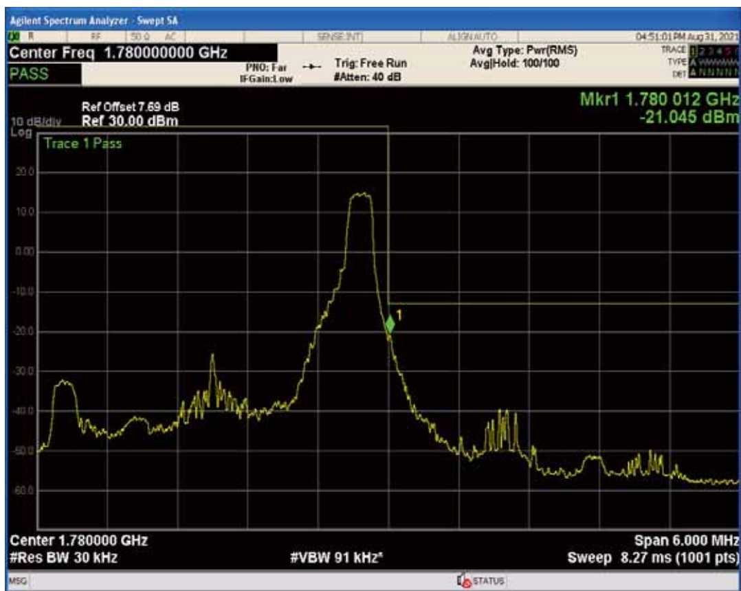
Band66 QAM16 BW=3MHz Channel=132657 RB Size=15 Position=#0
