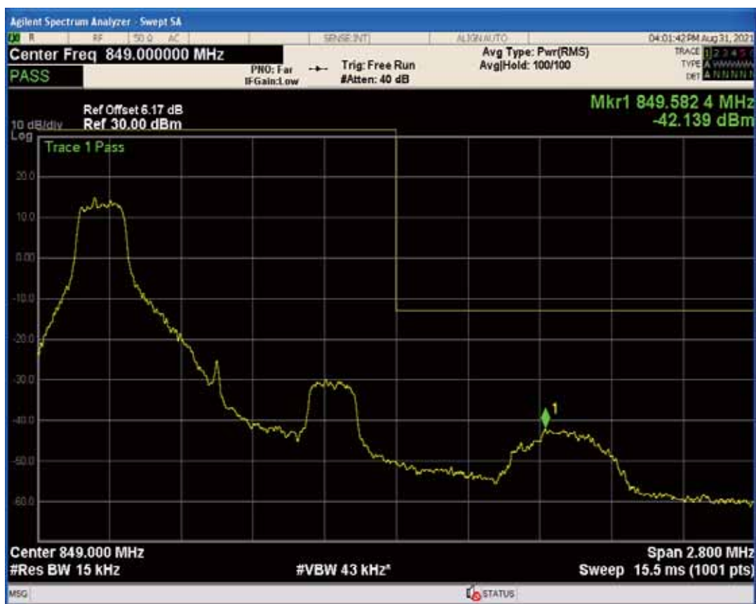
Band5 QAM16 BW=1.4MHz Channel=20407 RB Size=6 Position=#0
