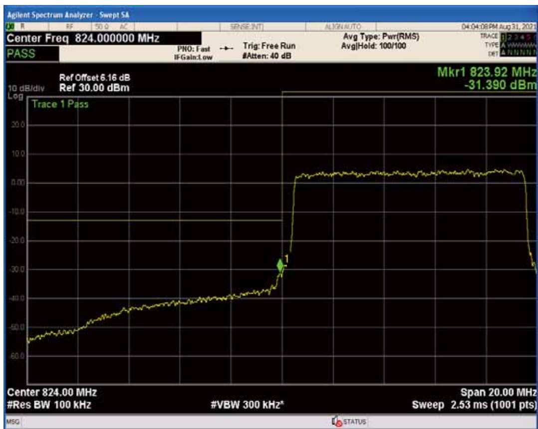
Band5 QAM16 BW=10MHz Channel=20450 RB Size=1 Position=#0
