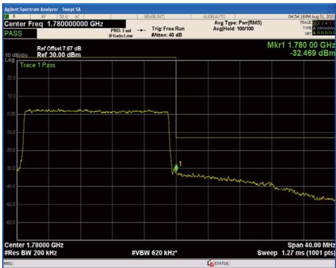
Band66 QAM16 BW=20MHz Channel=132572 RB Size=1 Position=#Max
