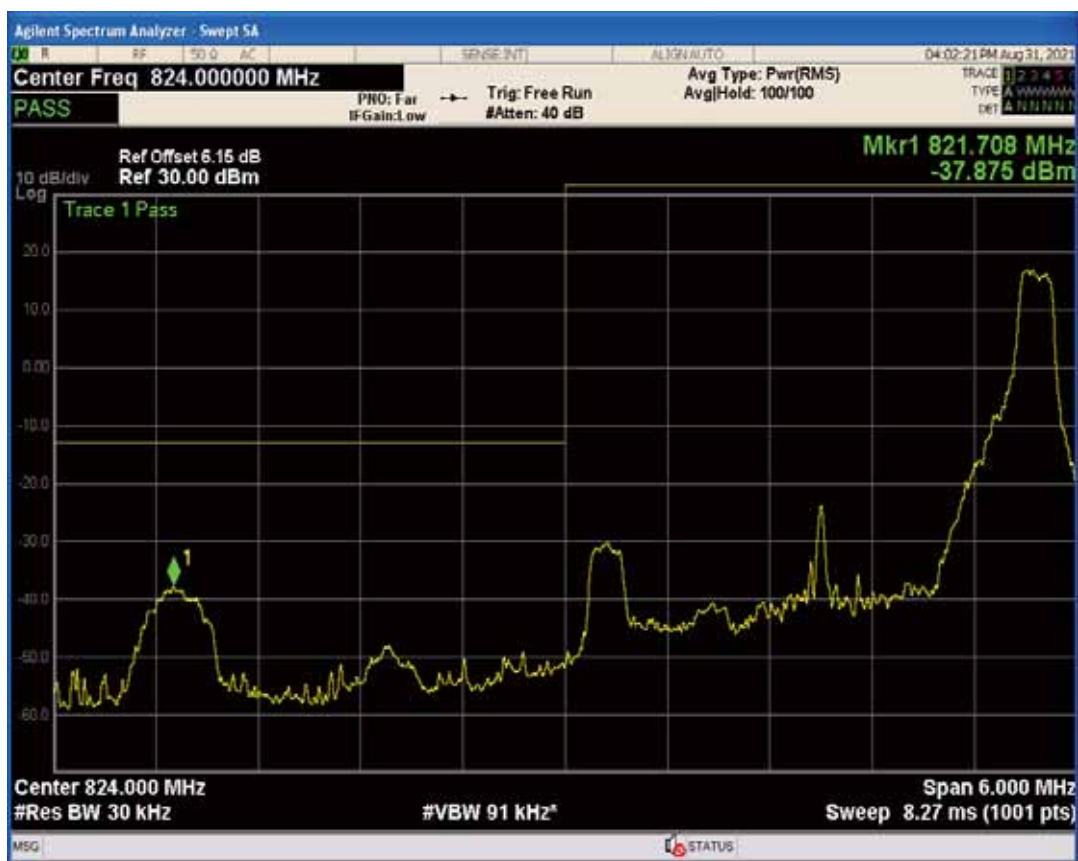
Band5 QPSK BW=3MHz Channel=20415 RB Size=15 Position=#0
