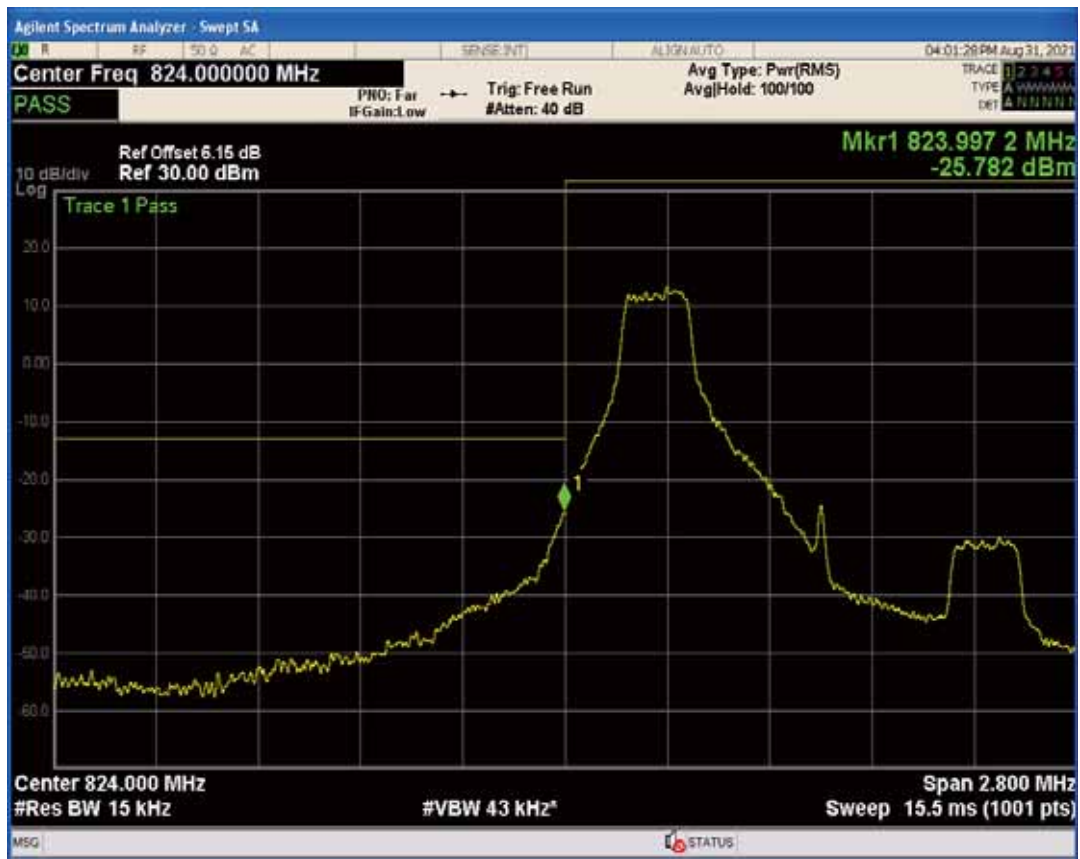
Band5 QAM16 BW=1.4MHz Channel=20407 RB Size=1 Position=#Max
