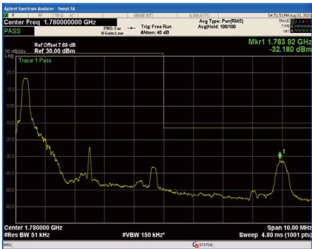
Band66 QAM16 BW=5MHz Channel=132647 RB Size=25 Position=#0
