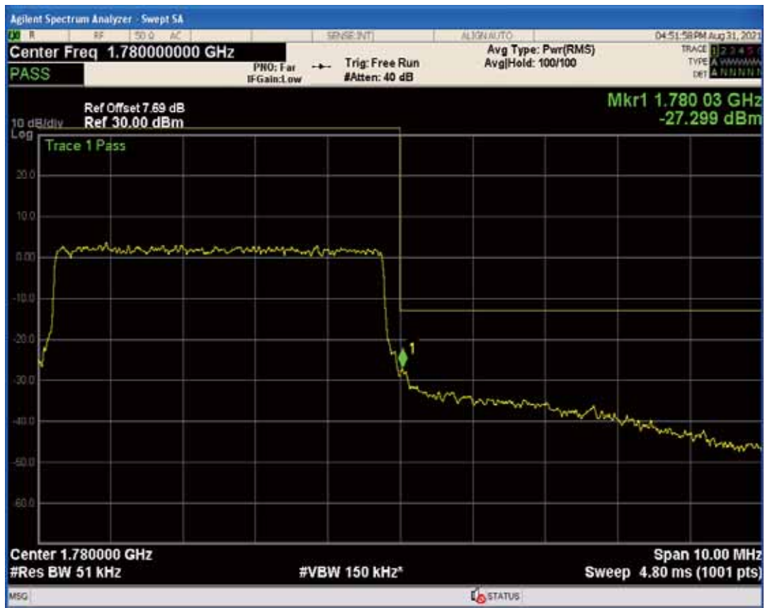
Band66 QPSK BW=10MHz Channel=132022 RB Size=1 Position=#0
