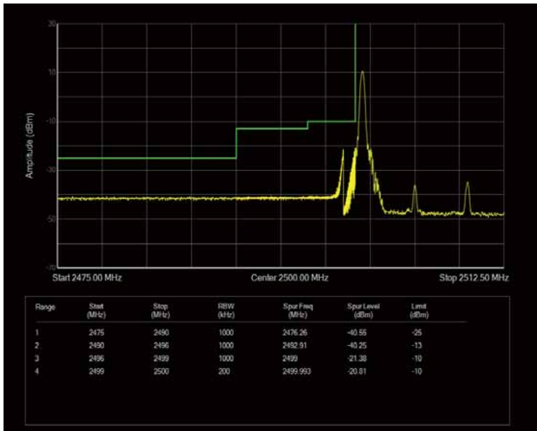
Band7 QAM16 BW=10MHz Channel=20800 RB Size=1 Position=#Max
