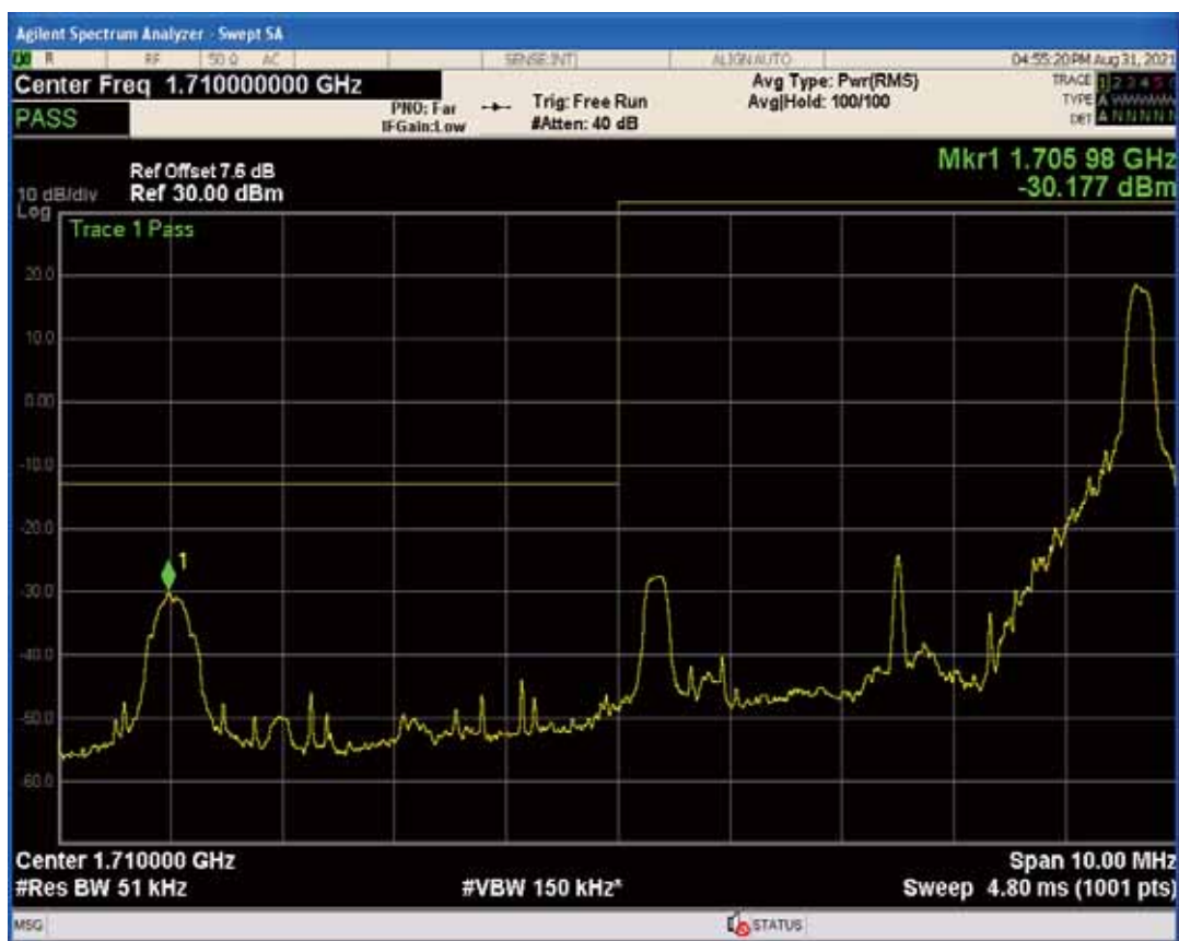
Band66 QAM16 BW=5MHz Channel=131997 RB Size=1 Position=#0
