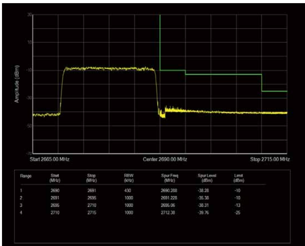
Band5 QPSK BW=1.4MHz Channel=20407 RB Size=1 Position=#0
