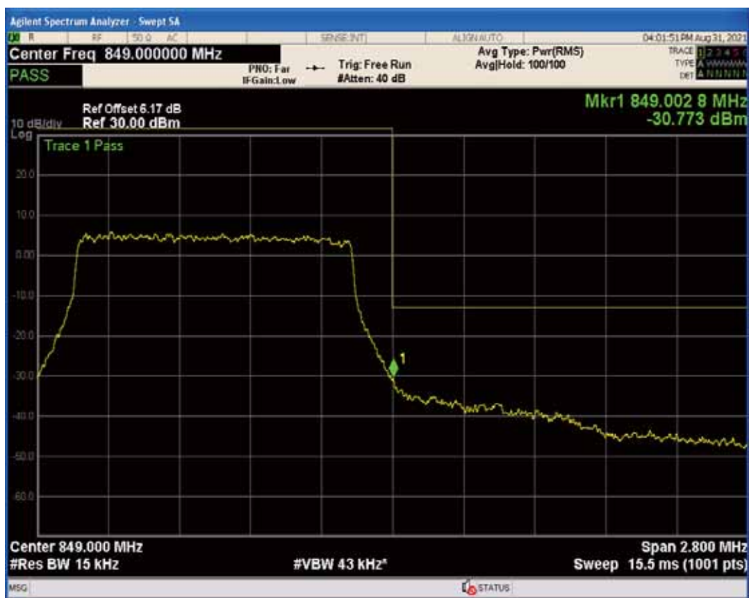
Band5 QAM16 BW=1.4MHz Channel=20643 RB Size=1 Position=#Max
