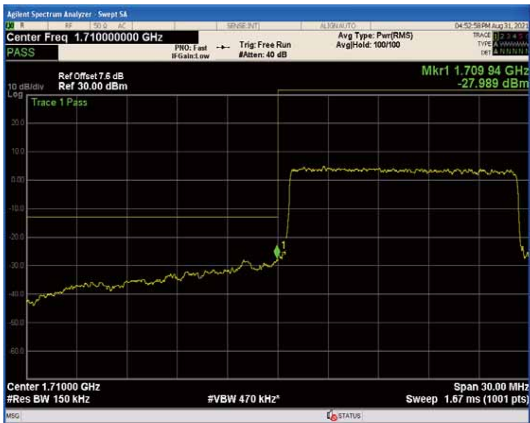
Band66 QPSK BW=15MHz Channel=132047 RB Size=1 Position=#Max
