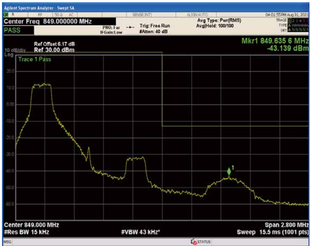
Band5 QPSK BW=1.4MHz Channel=20643 RB Size=6 Position=#0
