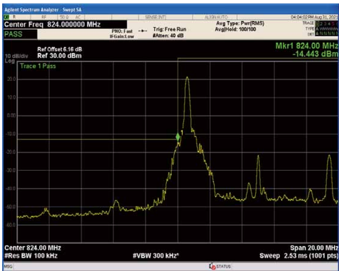
Band5 QAM16 BW=5MHz Channel=20625 RB Size=25 Position=#0
