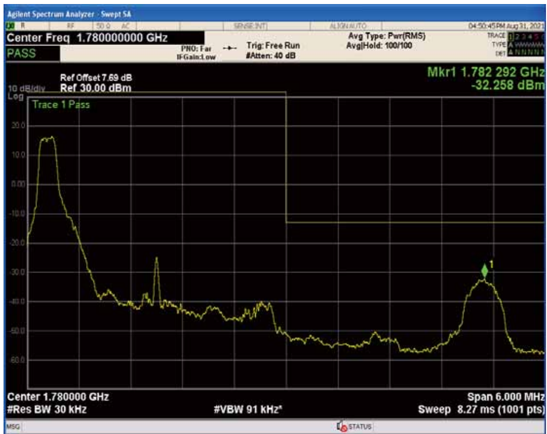
Band66 QPSK BW=3MHz Channel=132657 RB Size=1 Position=#Max
