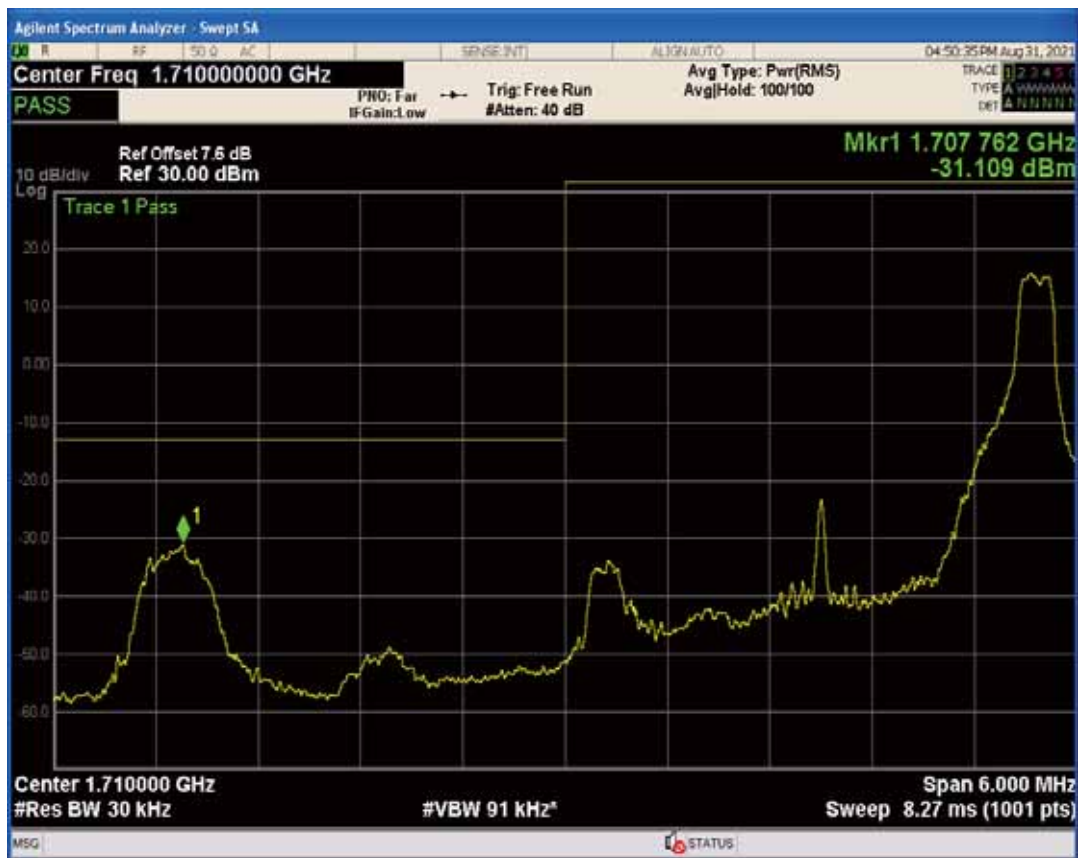
Band66 QAM16 BW=3MHz Channel=131987 RB Size=15 Position=#0
