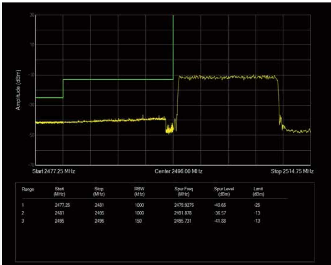
Band41 QAM16 BW=15MHz Channel=39725 RB Size=1 Position=#0
