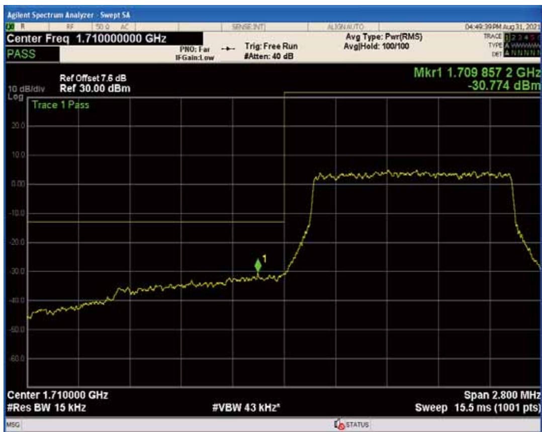
Band66 QPSK BW=1.4MHz Channel=132665 RB Size=1 Position=#Max
