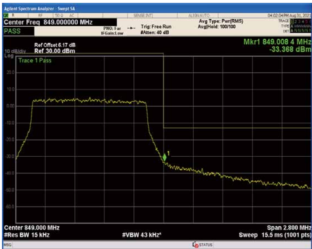
Band5 QPSK BW=3MHz Channel=20415 RB Size=1 Position=#Max
