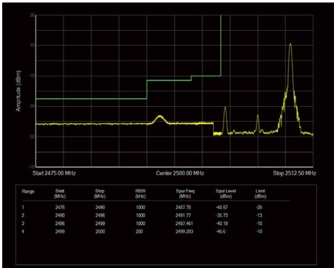
Band7 QAM16 BW=10MHz Channel=20800 RB Size=1 Position=#0
