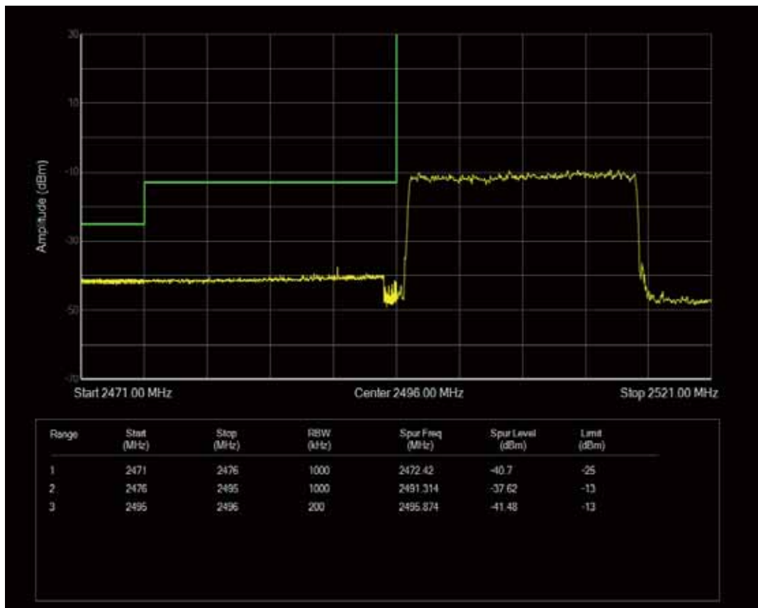
Band41 QAM16 BW=20MHz Channel=39750 RB Size=1 Position=#Max
