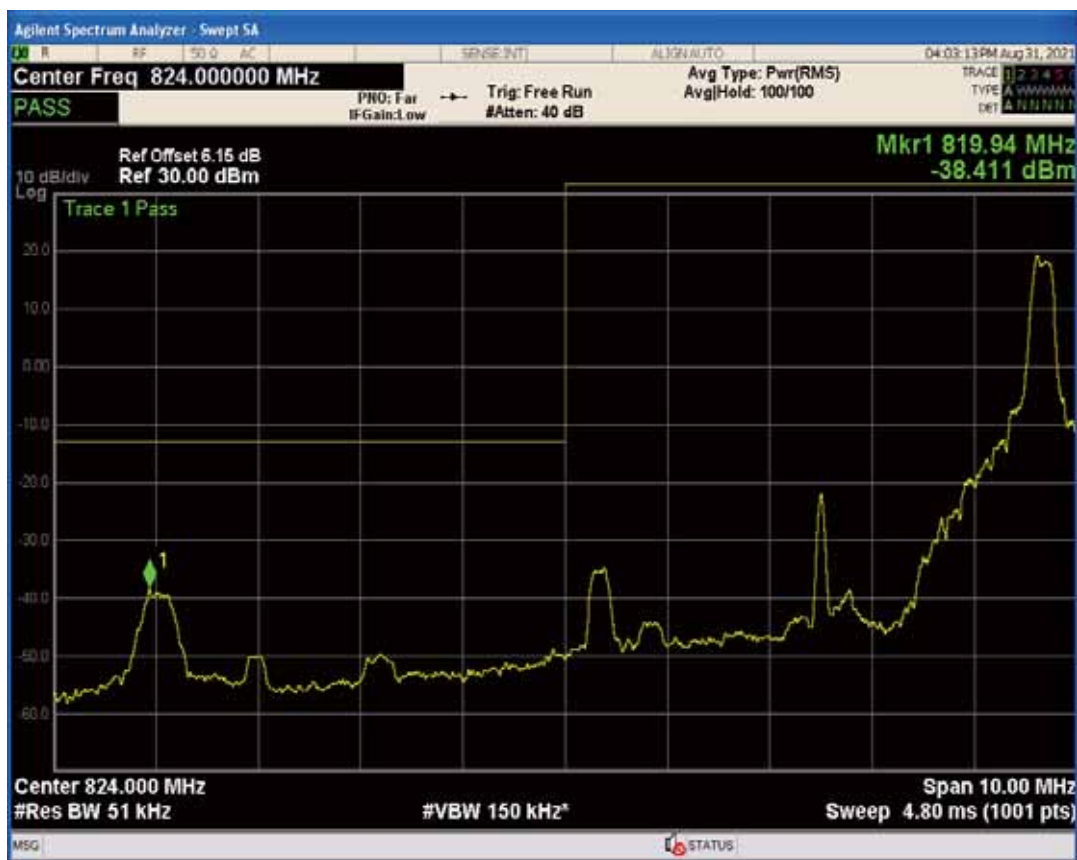
Band5 QPSK BW=5MHz Channel=20425 RB Size=1 Position=#0
