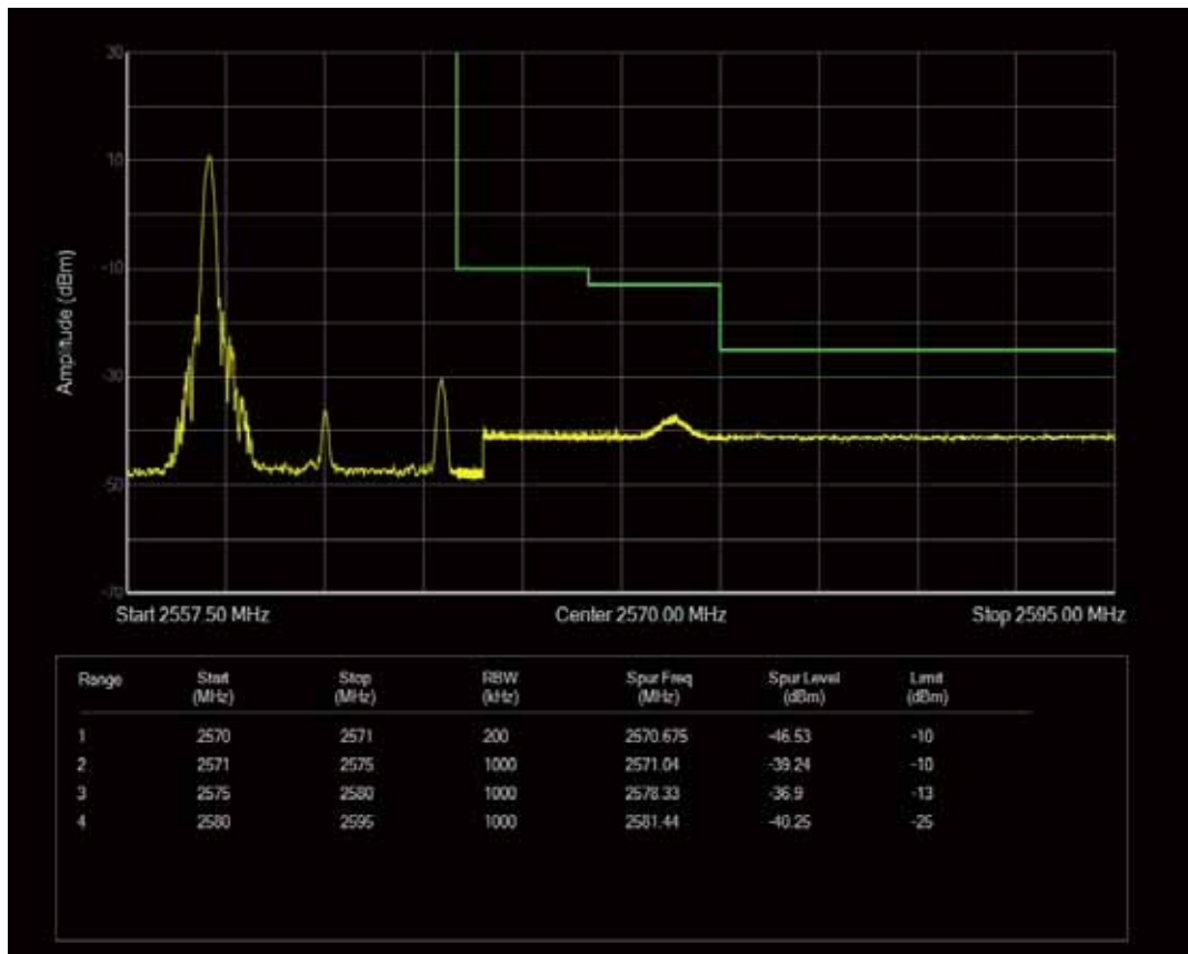
Band7 QAM16 BW=10MHz Channel=21400 RB Size=1 Position=#Max
