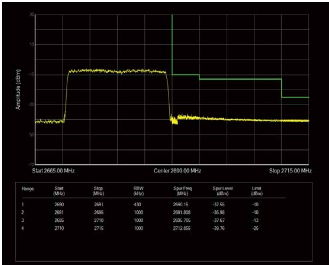
Band41 QAM16 BW=20MHz Channel=41490 RB Size=1 Position=#Max
