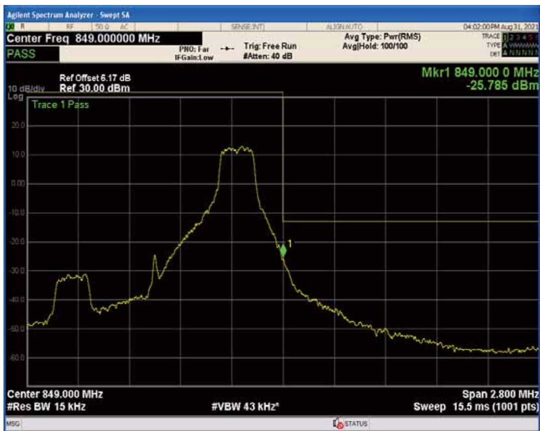
Band5 QPSK BW=3MHz Channel=20415 RB Size=1 Position=#0
