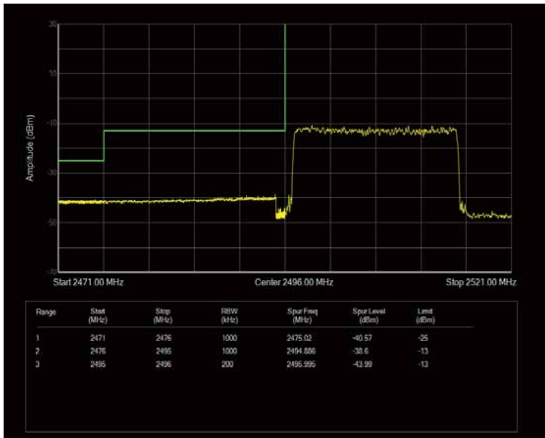
Band41 QPSK BW=20MHz Channel=41490 RB Size=1 Position=#Max
