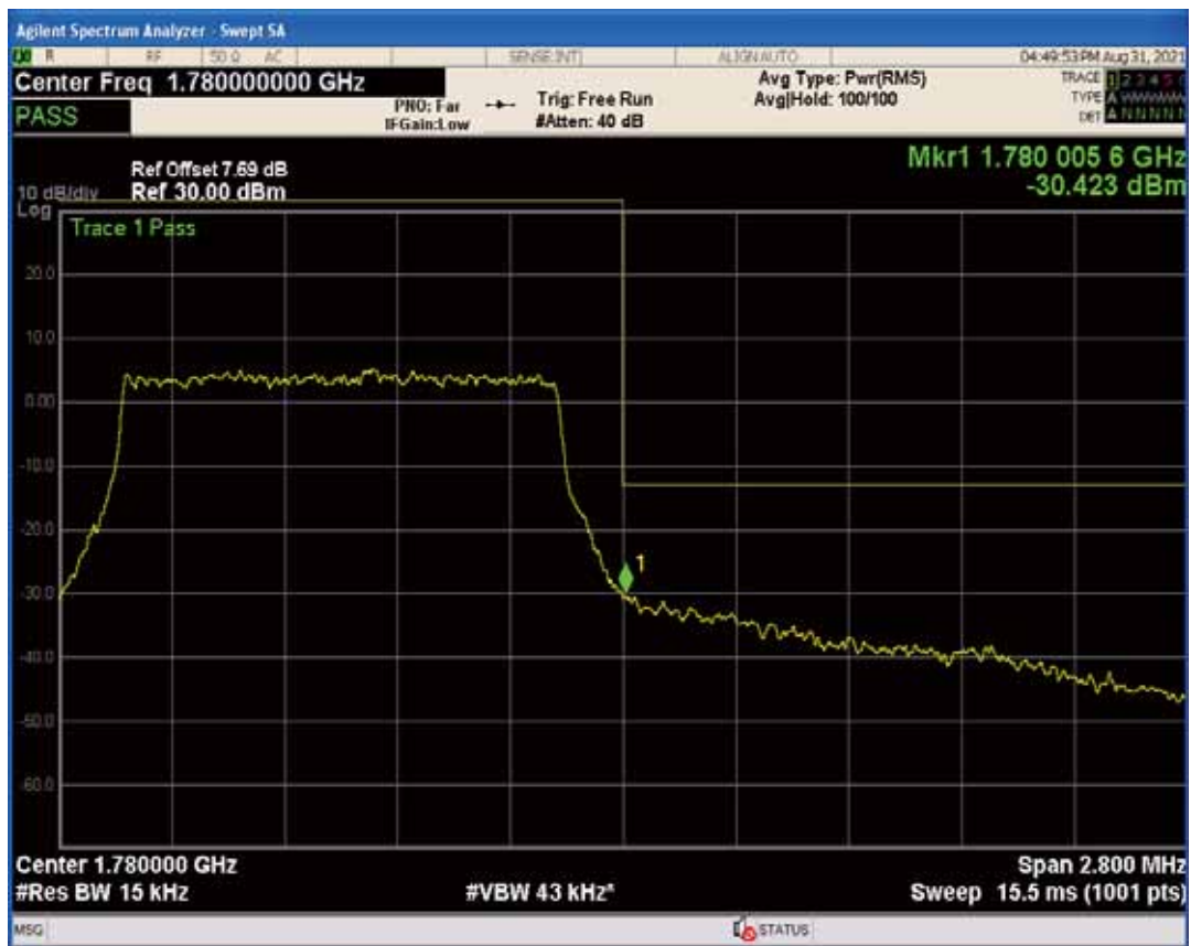
Band66 QAM16 BW=1.4MHz Channel=132665 RB Size=1 Position=#0
