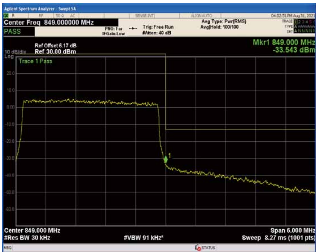
Band5 QAM16 BW=3MHz Channel=20635 RB Size=1 Position=#0
