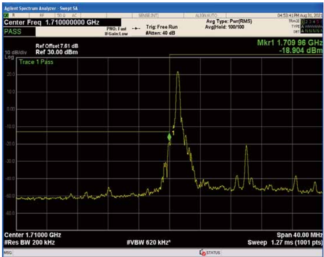
Band66 QPSK BW=20MHz Channel=132072 RB Size=100 Position=#0
