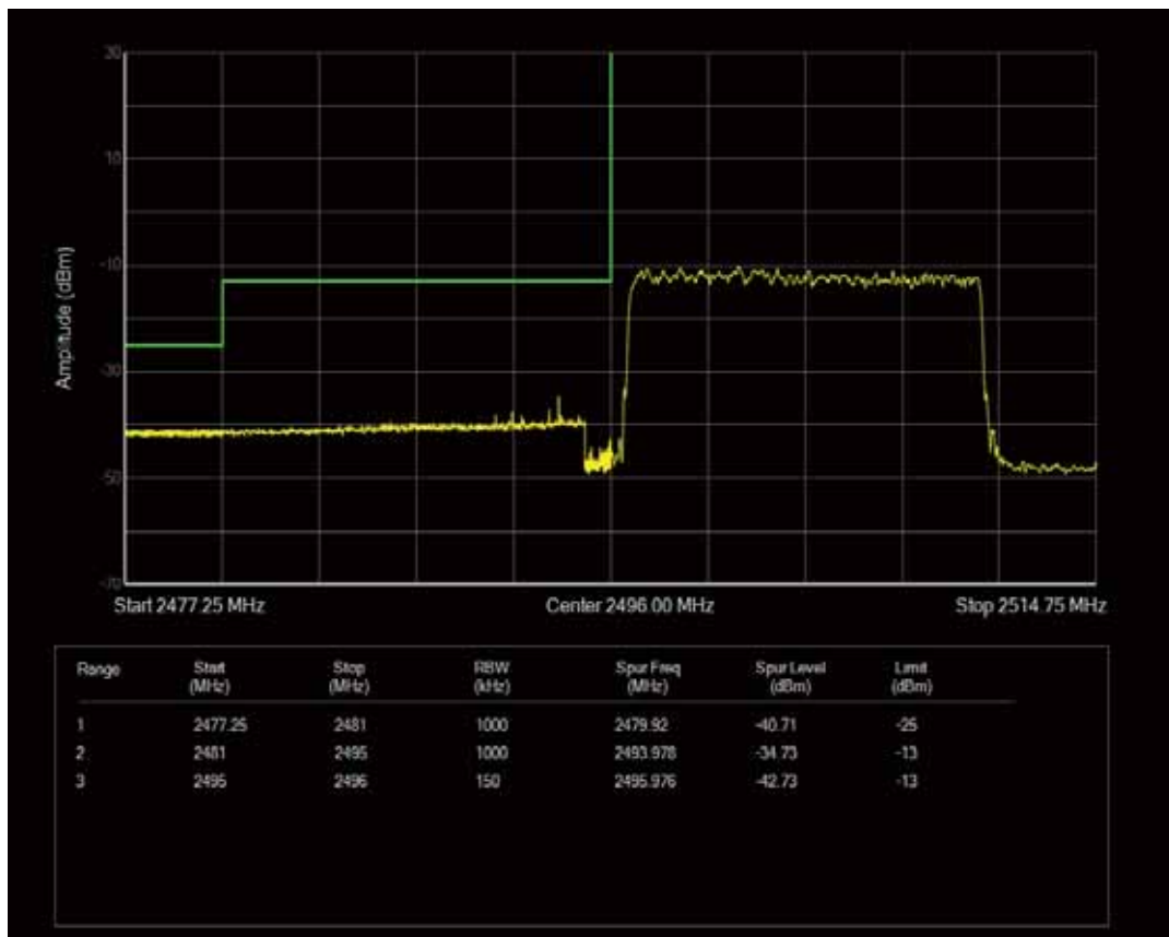
Band41 QAM16 BW=15MHz Channel=39725 RB Size=1 Position=#Max
