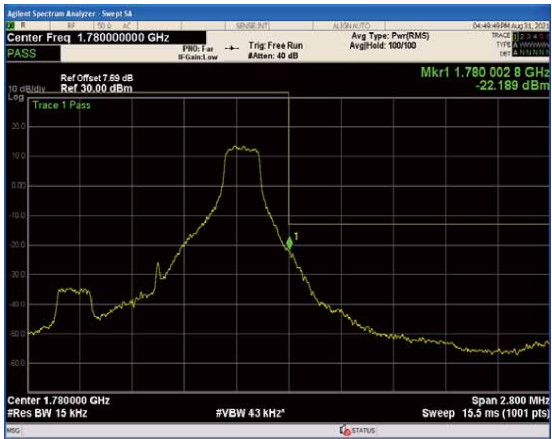
Band66 QPSK BW=1.4MHz Channel=132665 RB Size=6 Position=#0
