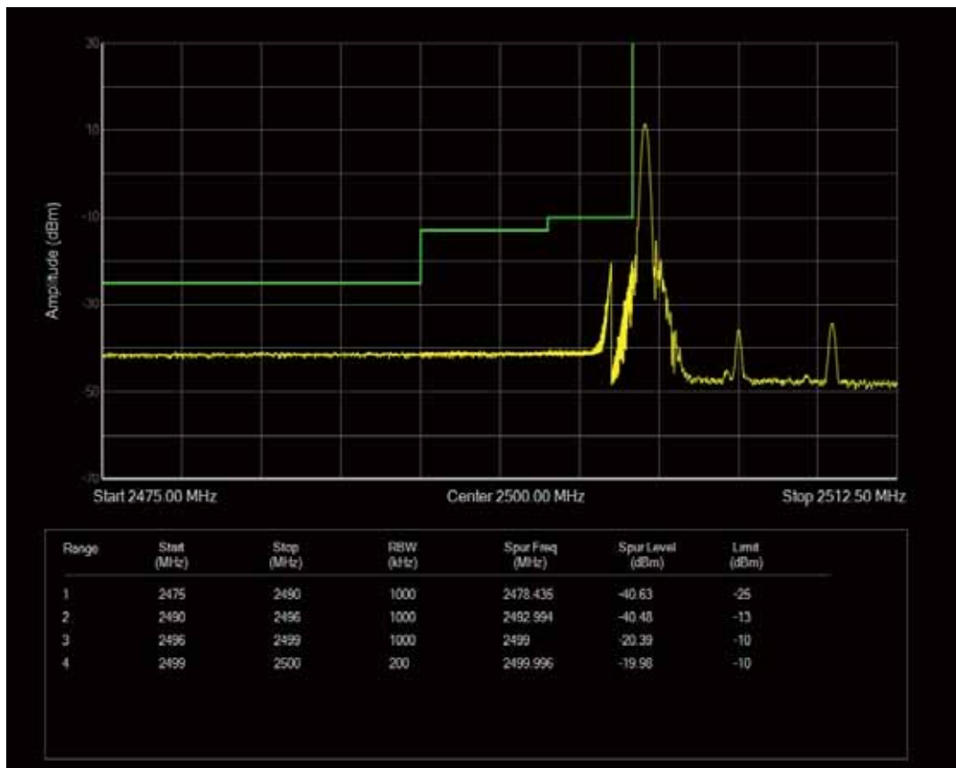
Band7 QPSK BW=10MHz Channel=20800 RB Size=50 Position=#0
