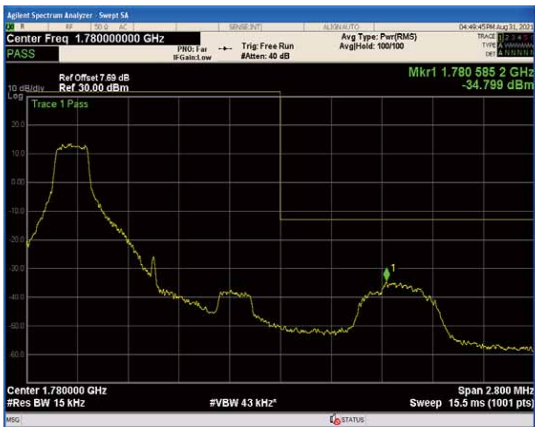
Band66 QAM16 BW=1.4MHz Channel=131979 RB Size=6 Position=#0
