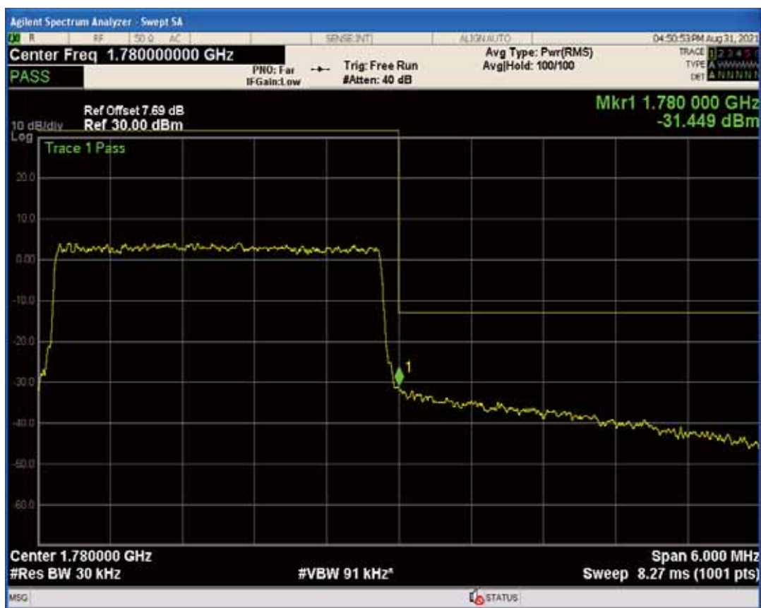
Band66 QAM16 BW=3MHz Channel=132657 RB Size=1 Position=#Max
