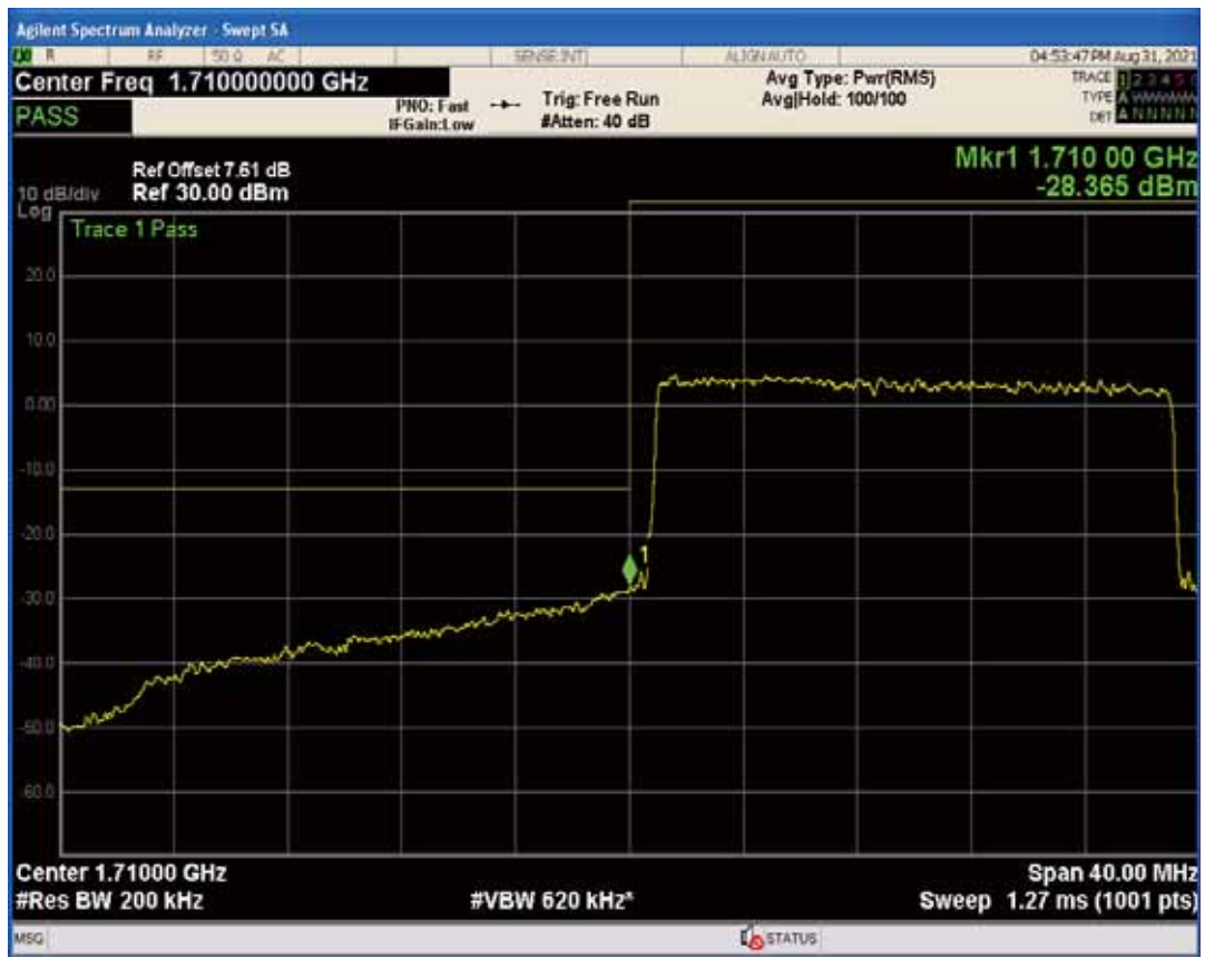
Band66 QPSK BW=20MHz Channel=132072 RB Size=1 Position=#Max
