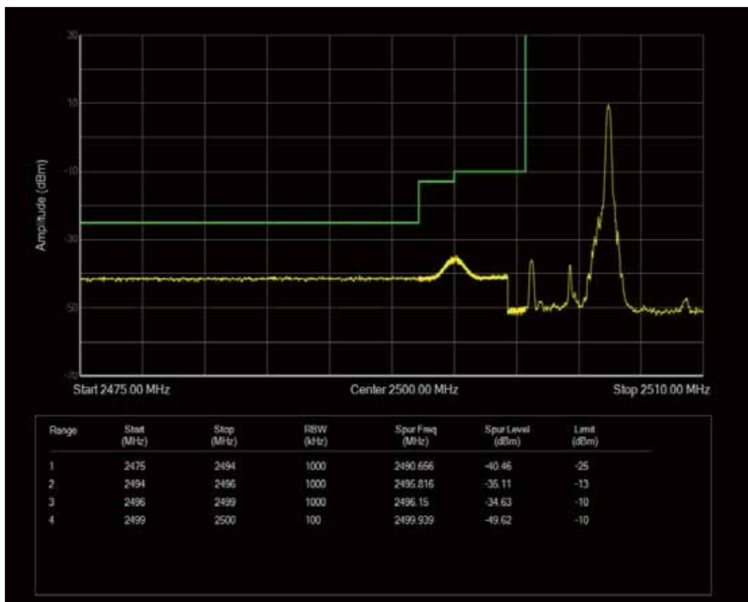
Band7 QPSK BW=5MHz Channel=20775 RB Size=1 Position=#0
