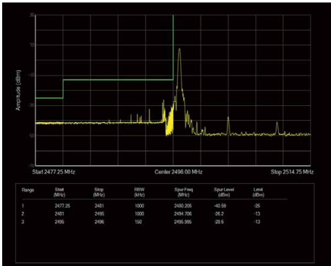
Band41 QPSK BW=15MHz Channel=39725 RB Size=1 Position=#Max
