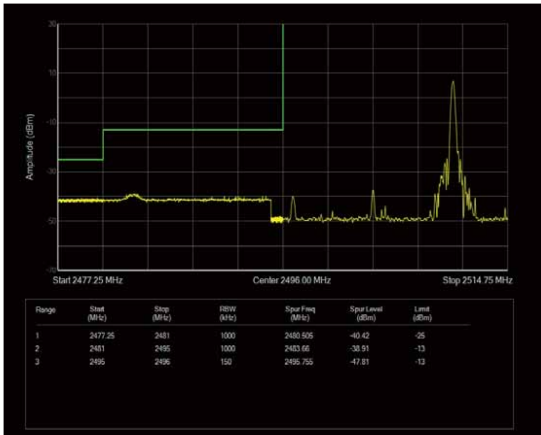
Band41 QPSK BW=15MHz Channel=39725 RB Size=75 Position=#0
