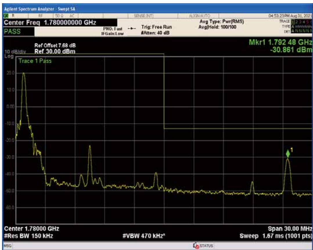
Band66 QAM16 BW=15MHz Channel=132597 RB Size=75 Position=#0
