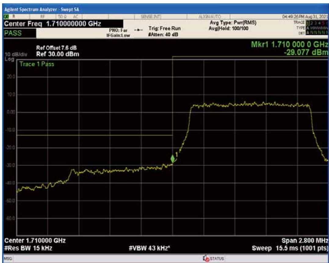
Band66 QAM16 BW=1.4MHz Channel=131979 RB Size=1 Position=#Max
