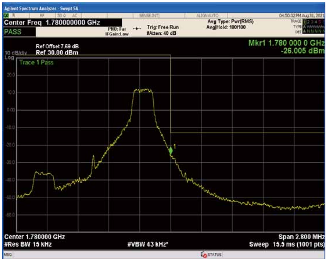
Band66 QPSK BW=3MHz Channel=131987 RB Size=1 Position=#0
