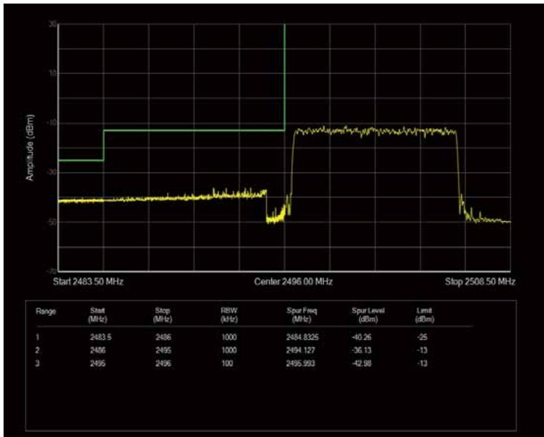
Band41 QPSK BW=10MHz Channel=41540 RB Size=1 Position=#Max
