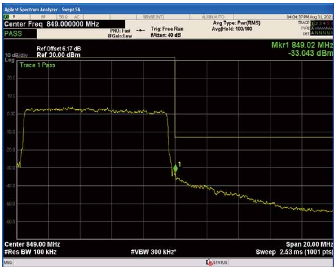
Band66 QPSK BW=1.4MHz Channel=131979 RB Size=1 Position=#0
