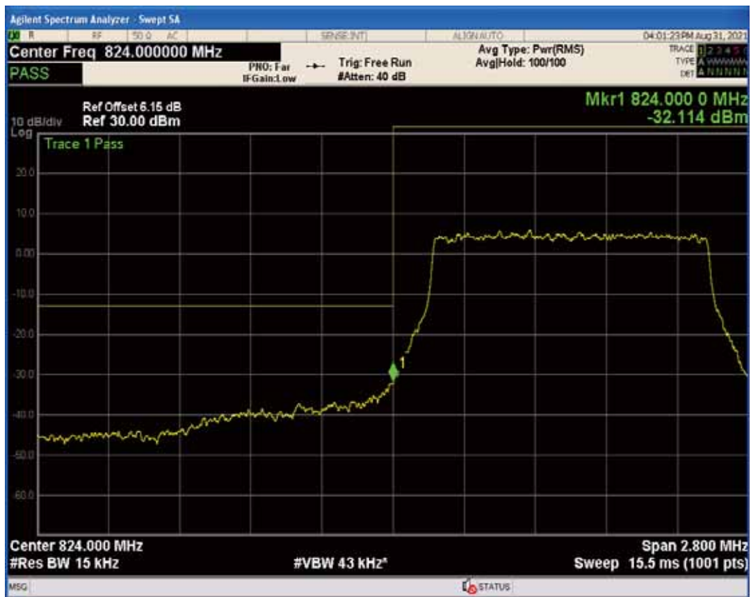
Band5 QAM16 BW=1.4MHz Channel=20407 RB Size=1 Position=#0
