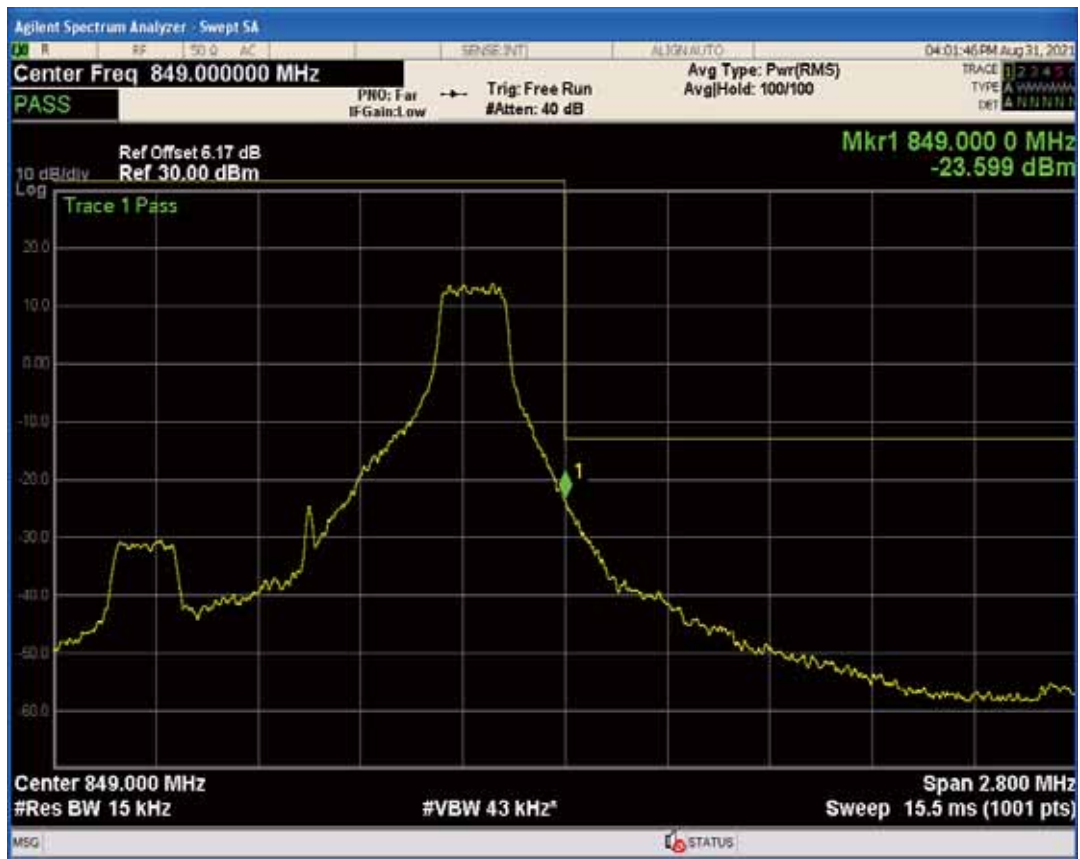
Band5 QAM16 BW=1.4MHz Channel=20643 RB Size=1 Position=#0
