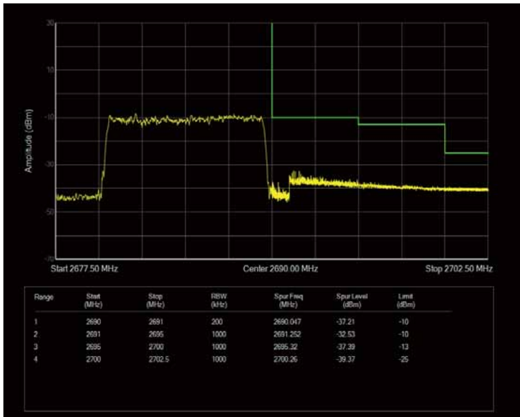
Band41 QPSK BW=15MHz Channel=39725 RB Size=1 Position=#0
