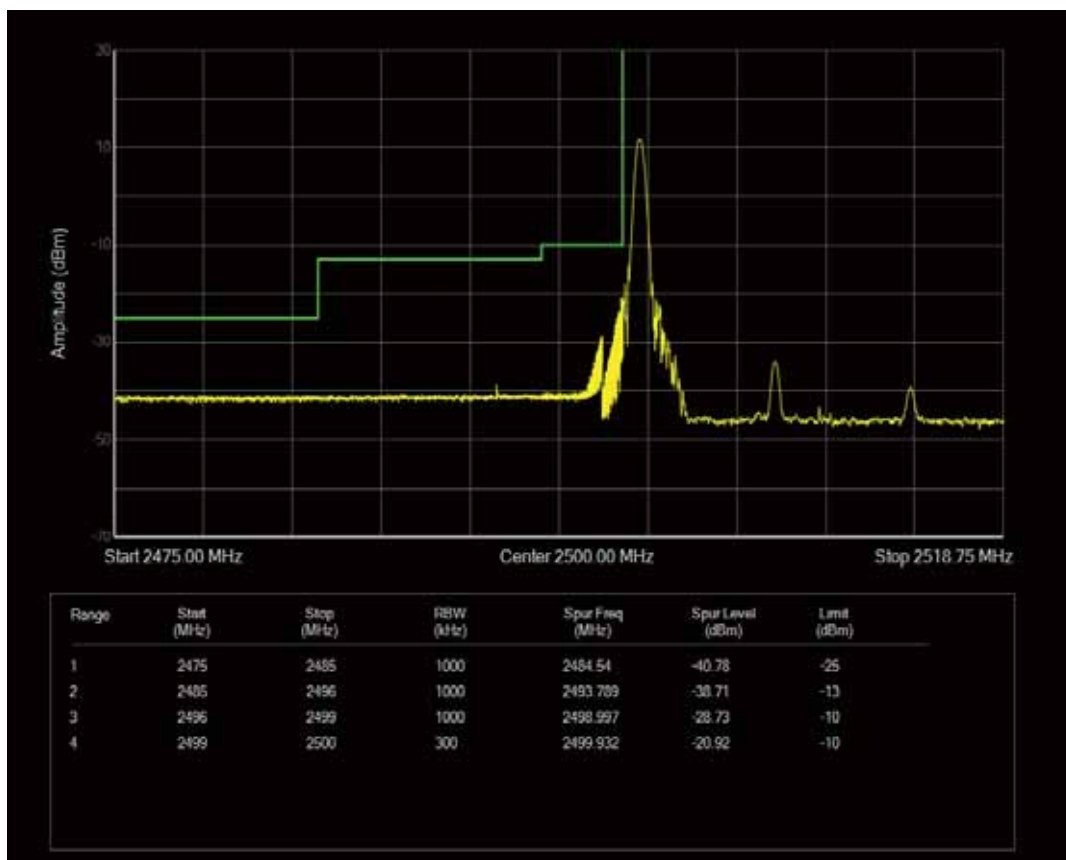
Band7 QPSK BW=15MHz Channel=20825 RB Size=1 Position=#Max
