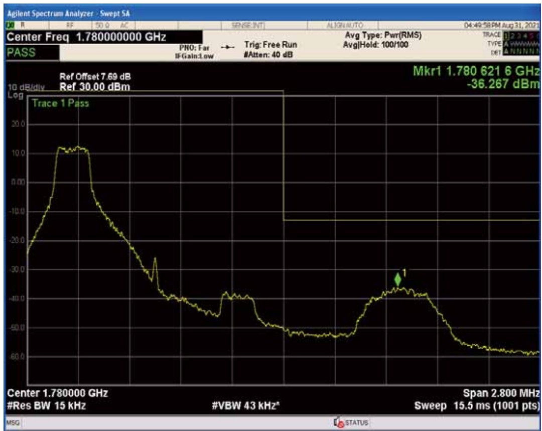
Band66 QAM16 BW=1.4MHz Channel=132665 RB Size=1 Position=#Max
