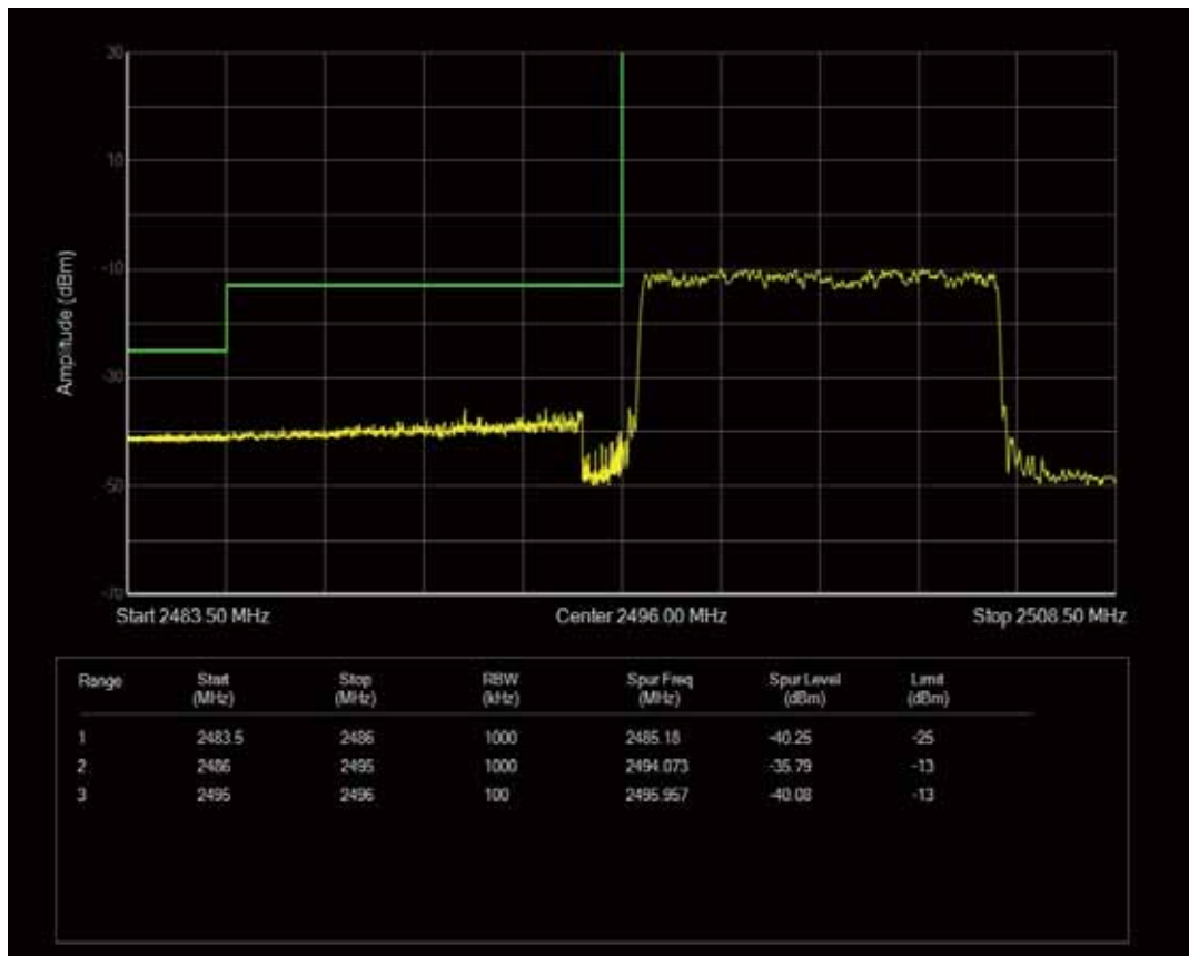
Band41 QPSK BW=10MHz Channel=39700 RB Size=1 Position=#Max
