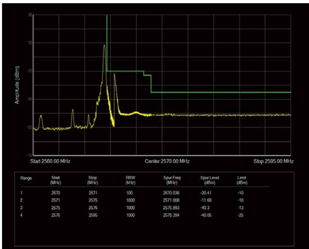
Band7 QAM16 BW=5MHz Channel=21425 RB Size=1 Position=#0
