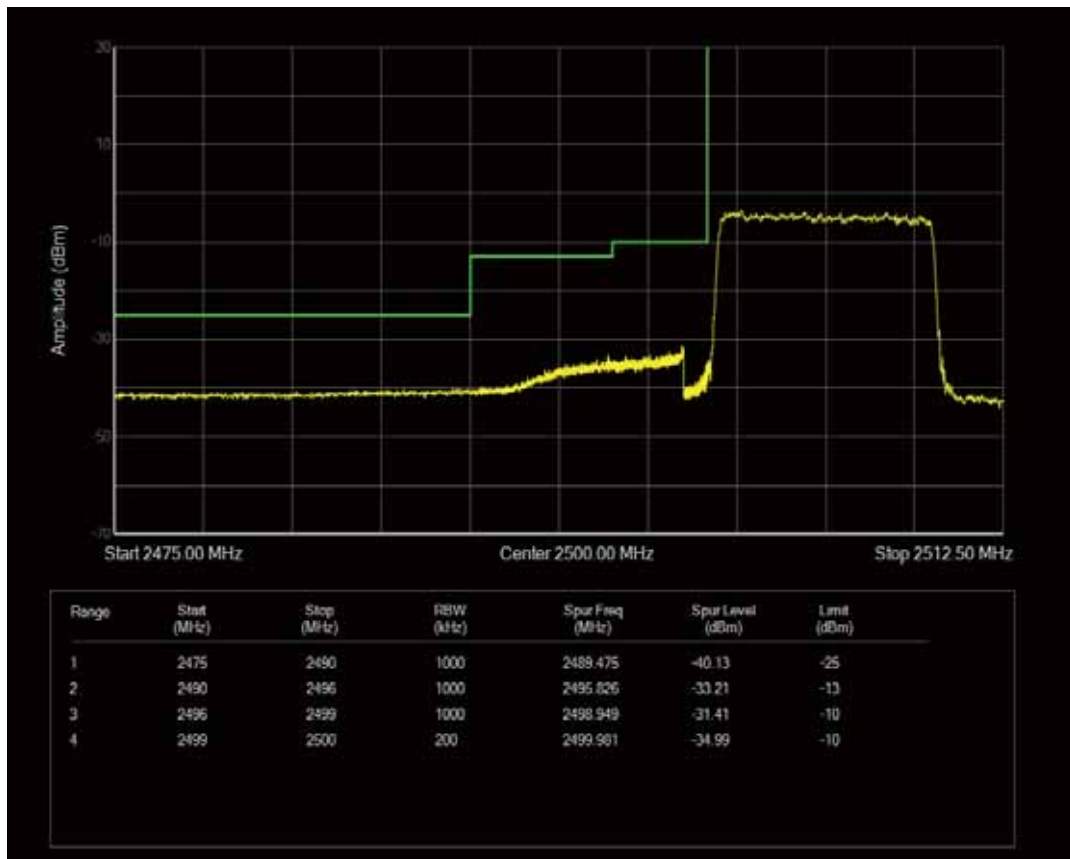
Band7 QPSK BW=10MHz Channel=20800 RB Size=1 Position=#Max
