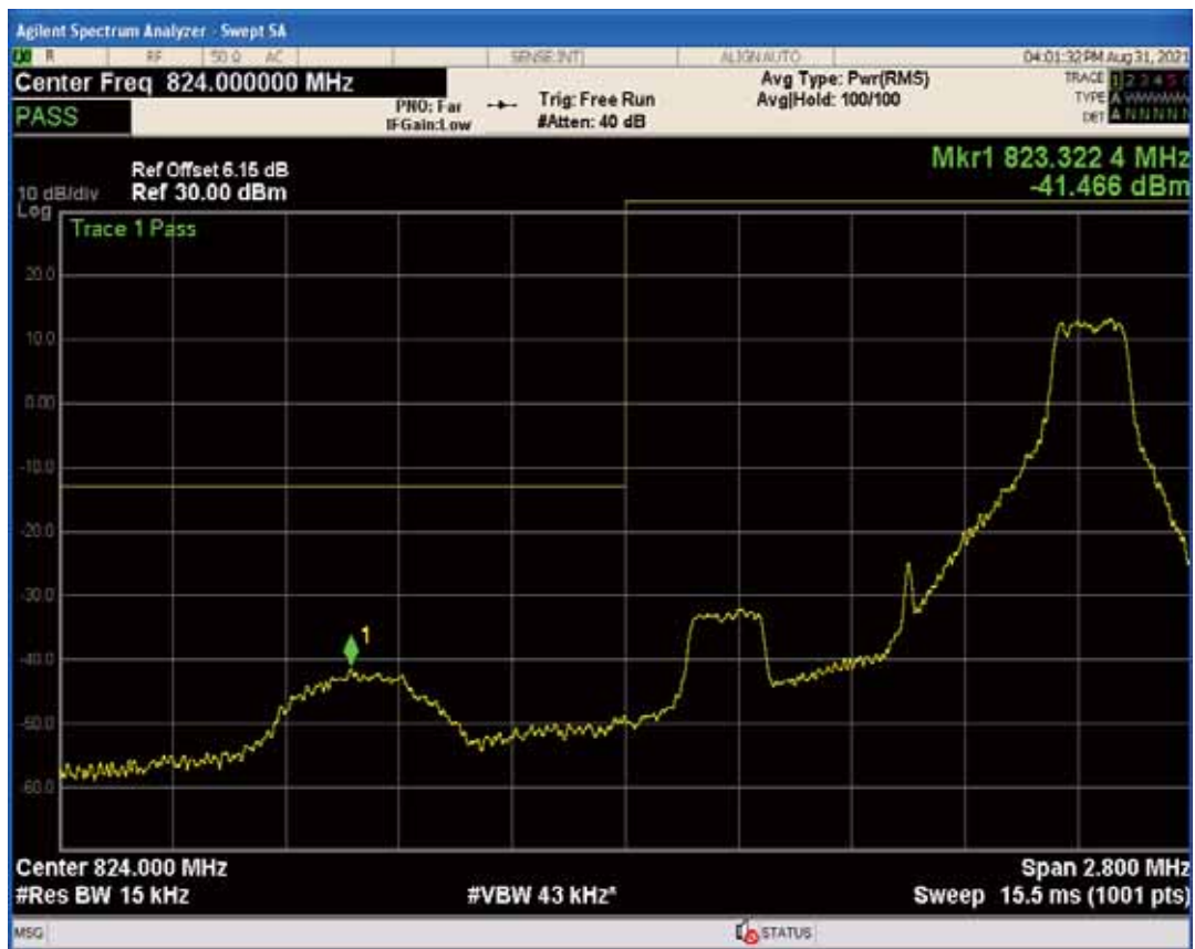
Band5 QPSK BW=1.4MHz Channel=20643 RB Size=1 Position=#0
