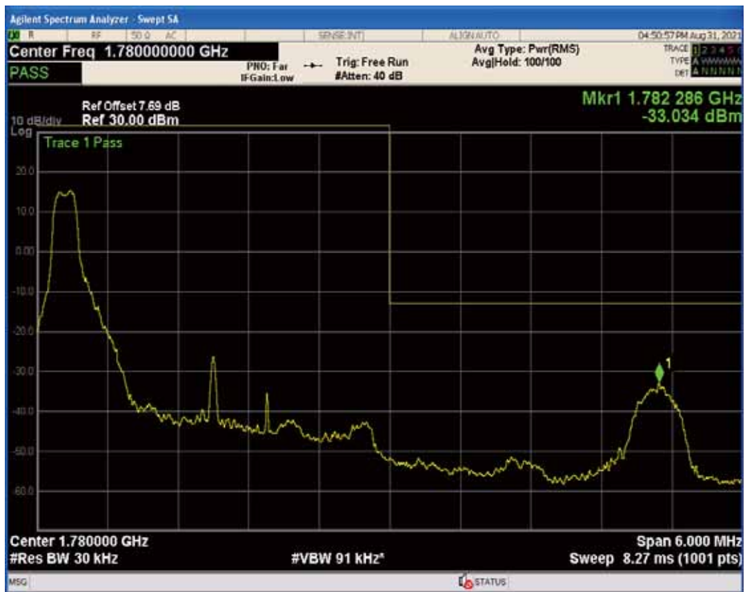
Band66 QPSK BW=3MHz Channel=132657 RB Size=15 Position=#0
