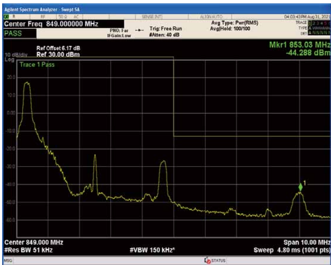
Band5 QAM16 BW=5MHz Channel=20625 RB Size=1 Position=#Max
