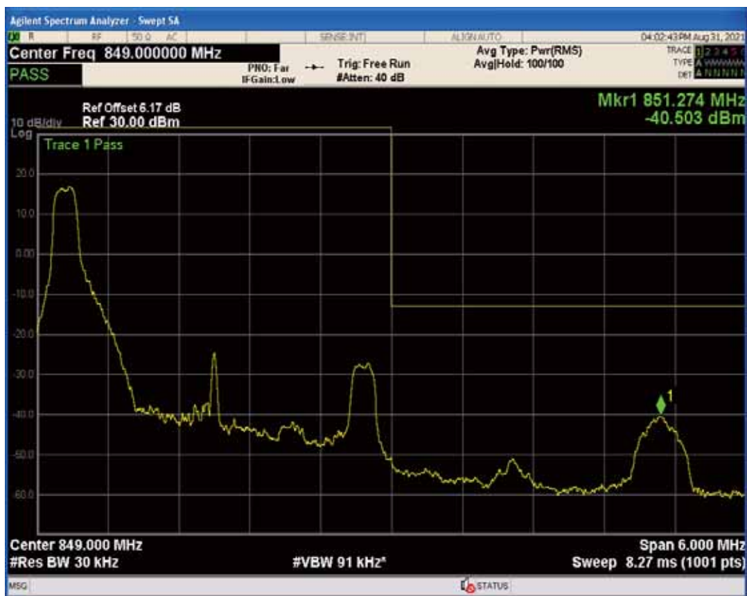
Band5 QPSK BW=3MHz Channel=20635 RB Size=1 Position=#Max
