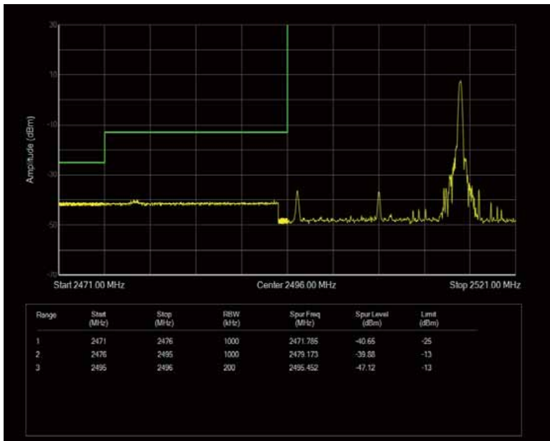
Band41 QPSK BW=20MHz Channel=39750 RB Size=1 Position=#0
