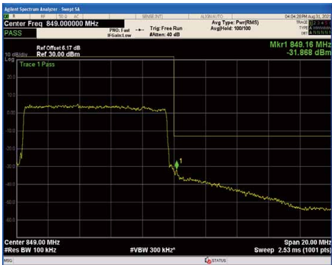
Band5 QAM16 BW=10MHz Channel=20600 RB Size=1 Position=#0
