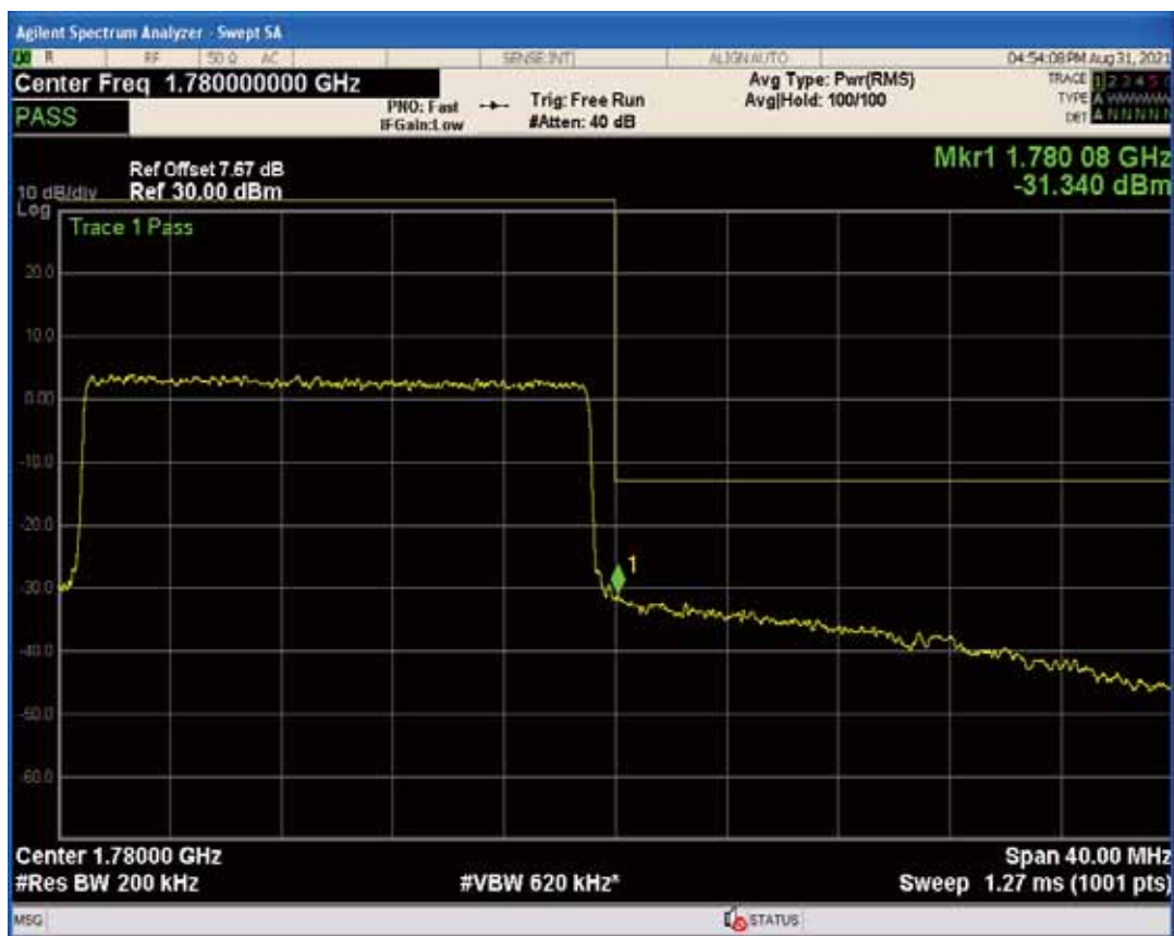
Band66 QAM16 BW=20MHz Channel=132572 RB Size=1 Position=#0
