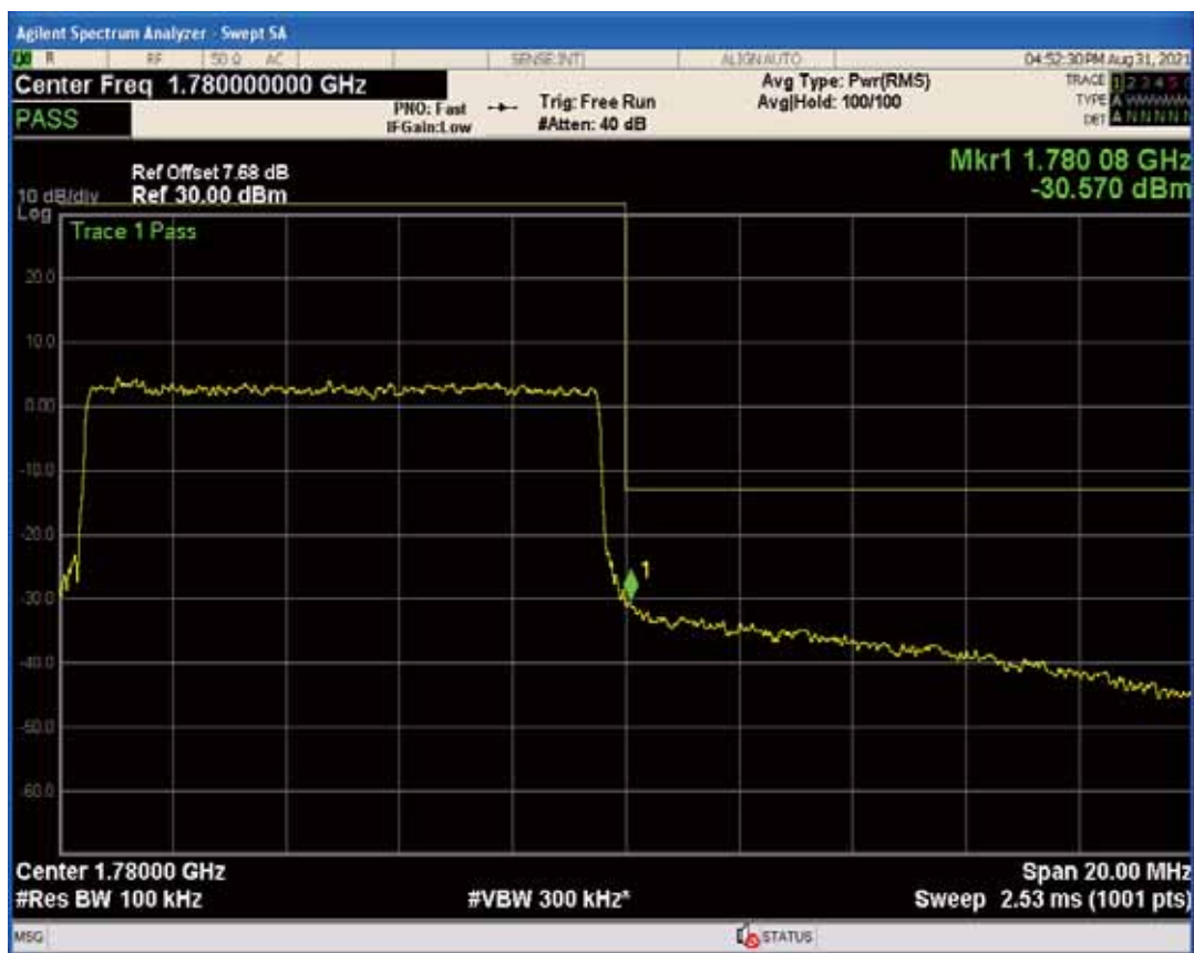
Band66 QAM16 BW=10MHz Channel=132622 RB Size=1 Position=#0
