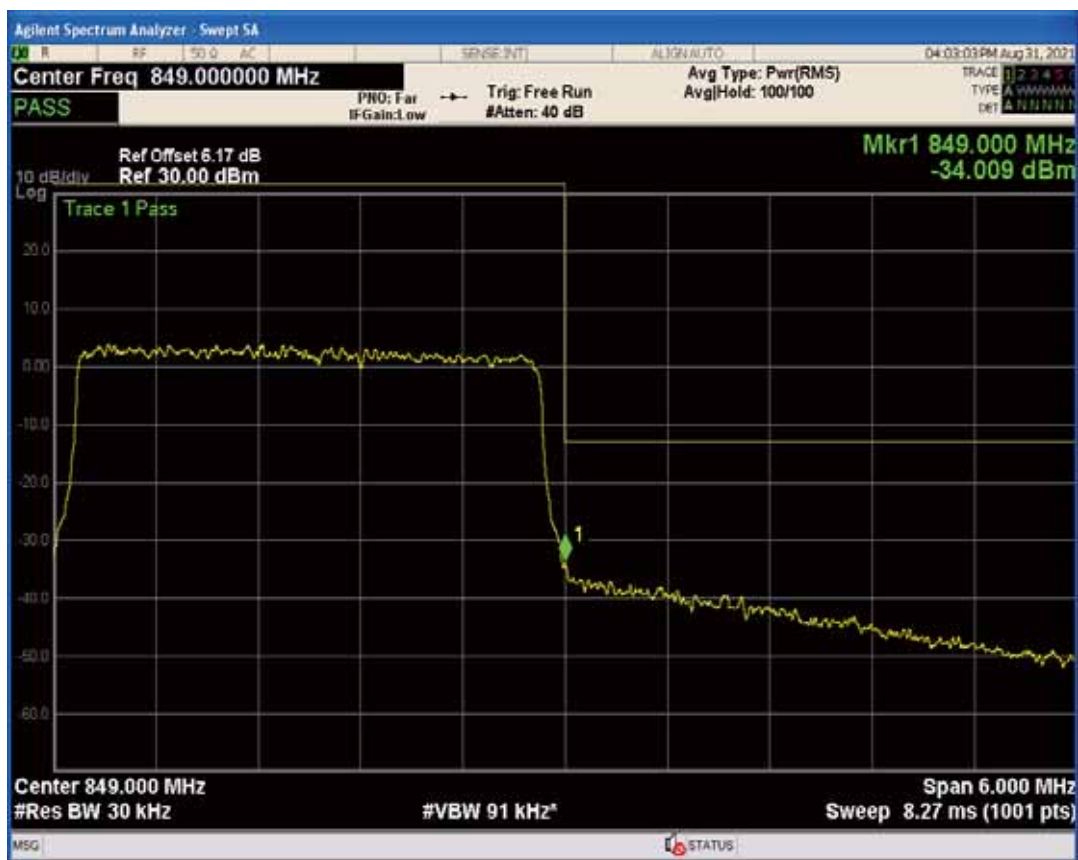
Band5 QAM16 BW=3MHz Channel=20635 RB Size=1 Position=#Max
