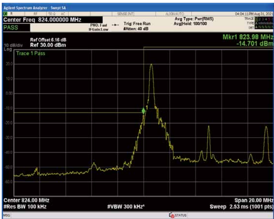
Band5 QAM16 BW=10MHz Channel=20450 RB Size=1 Position=#Max
