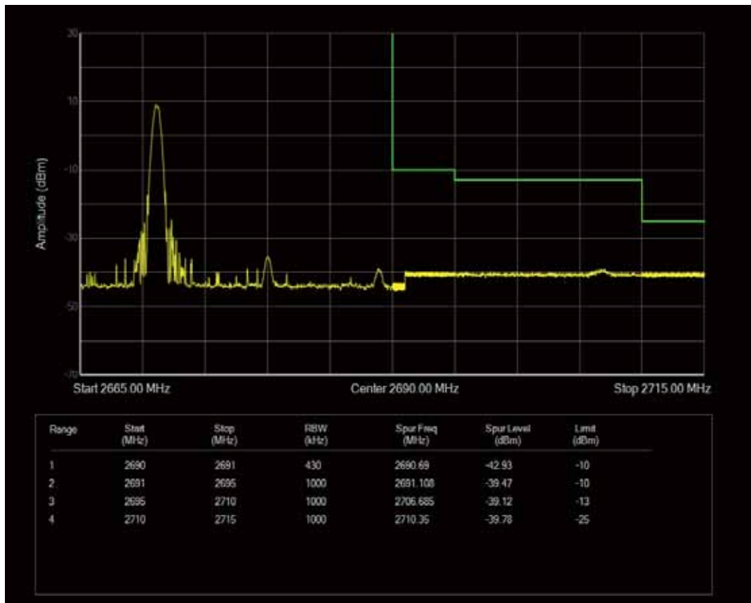
Band41 QAM16 BW=20MHz Channel=41490 RB Size=1 Position=#0
