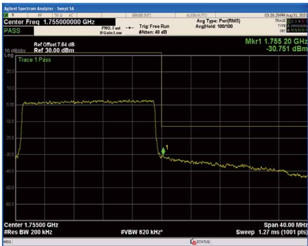
Band4 QAM16 BW=20MHz Channel=20300 RB Size=1 Position=#Max
