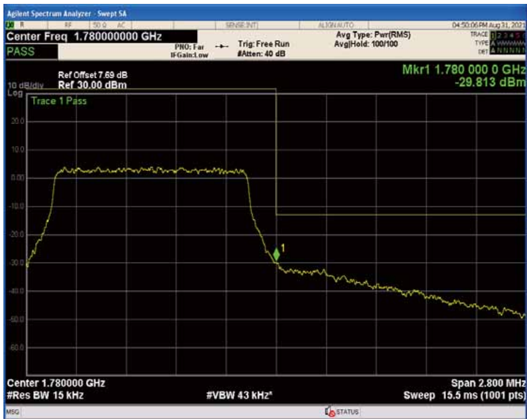
Band66 QPSK BW=3MHz Channel=131987 RB Size=1 Position=#Max
