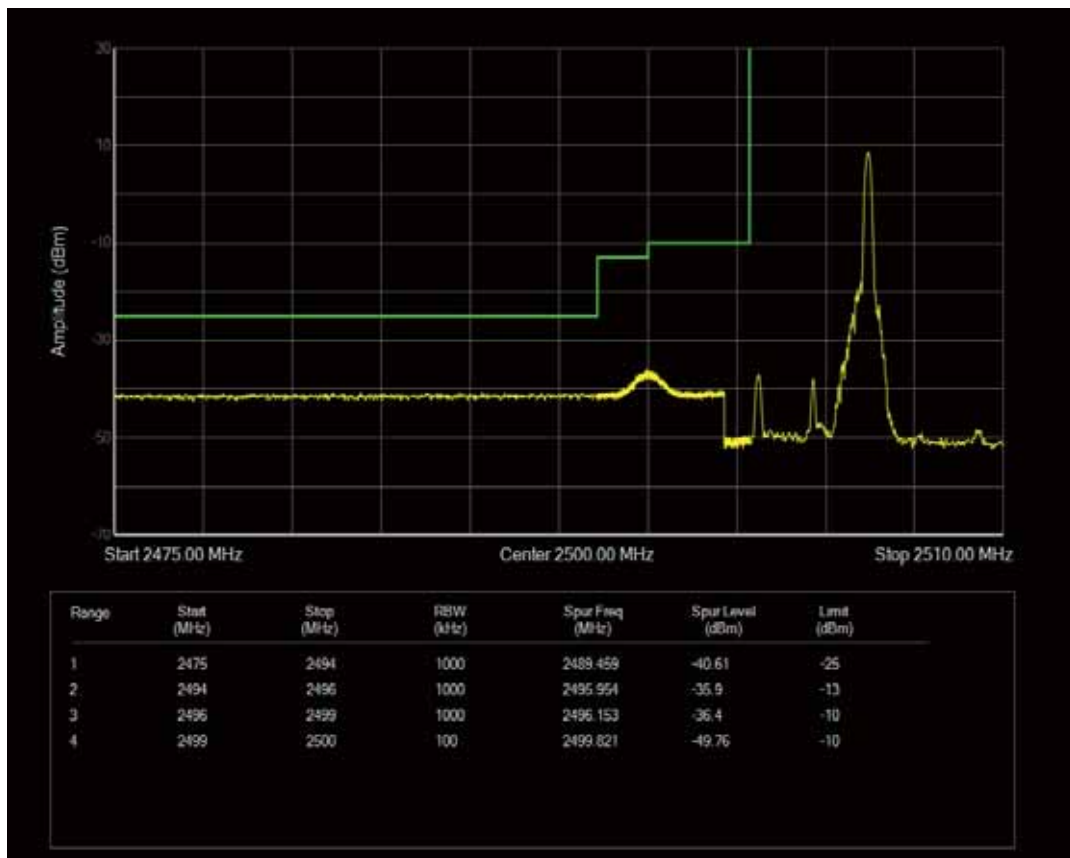
Band7 QAM16 BW=5MHz Channel=20775 RB Size=25 Position=#0
