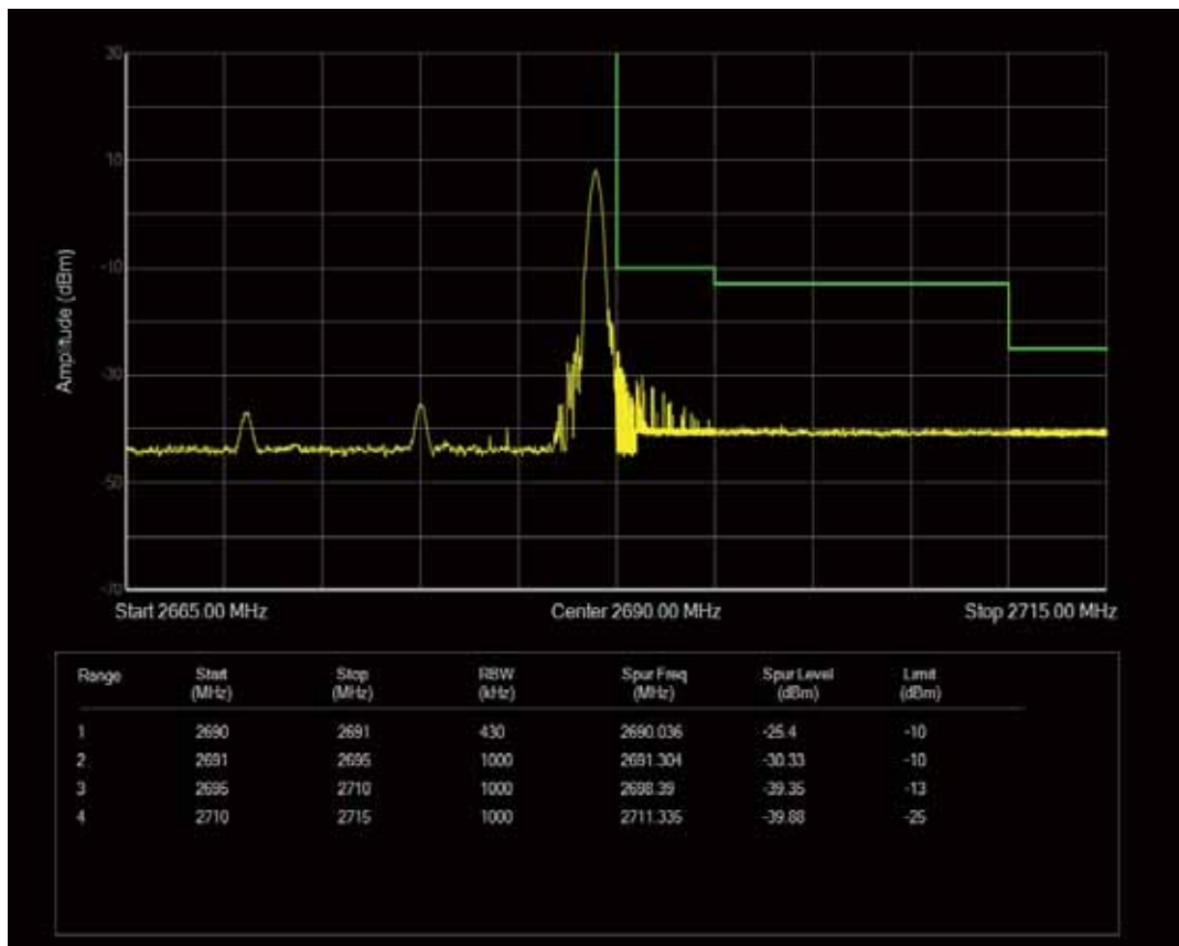
Band41 QPSK BW=20MHz Channel=41490 RB Size=1 Position=#0
