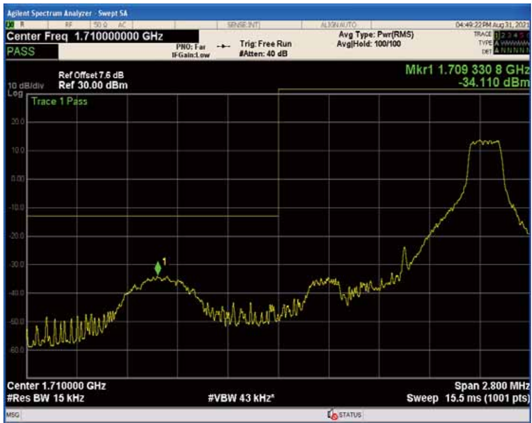
Band66 QAM16 BW=1.4MHz Channel=131979 RB Size=1 Position=#0
