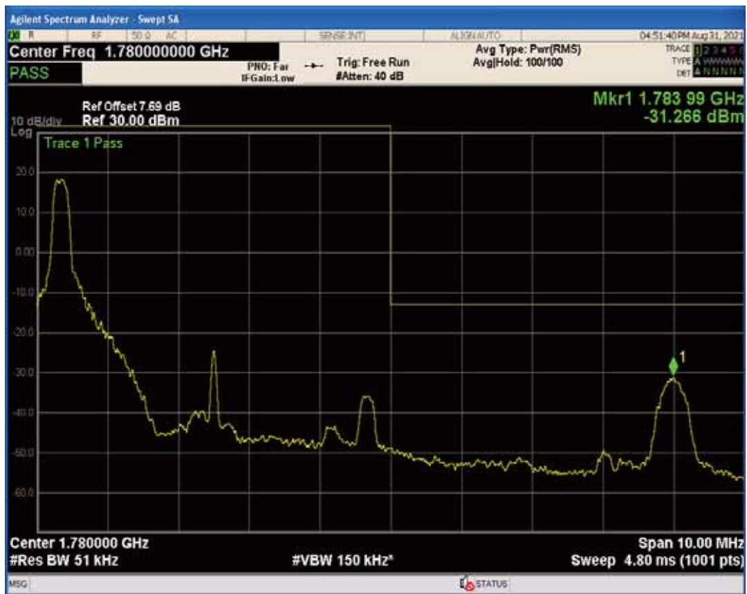
Band66 QPSK BW=5MHz Channel=132647 RB Size=1 Position=#Max
