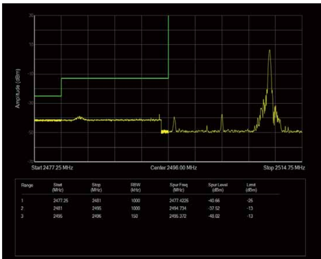
Band41 QPSK BW=15MHz Channel=41515 RB Size=1 Position=#0
