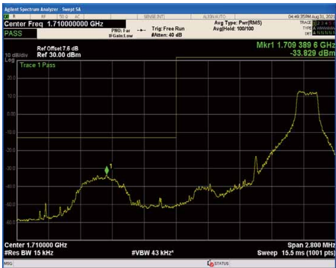
Band66 QPSK BW=1.4MHz Channel=132665 RB Size=1 Position=#0
