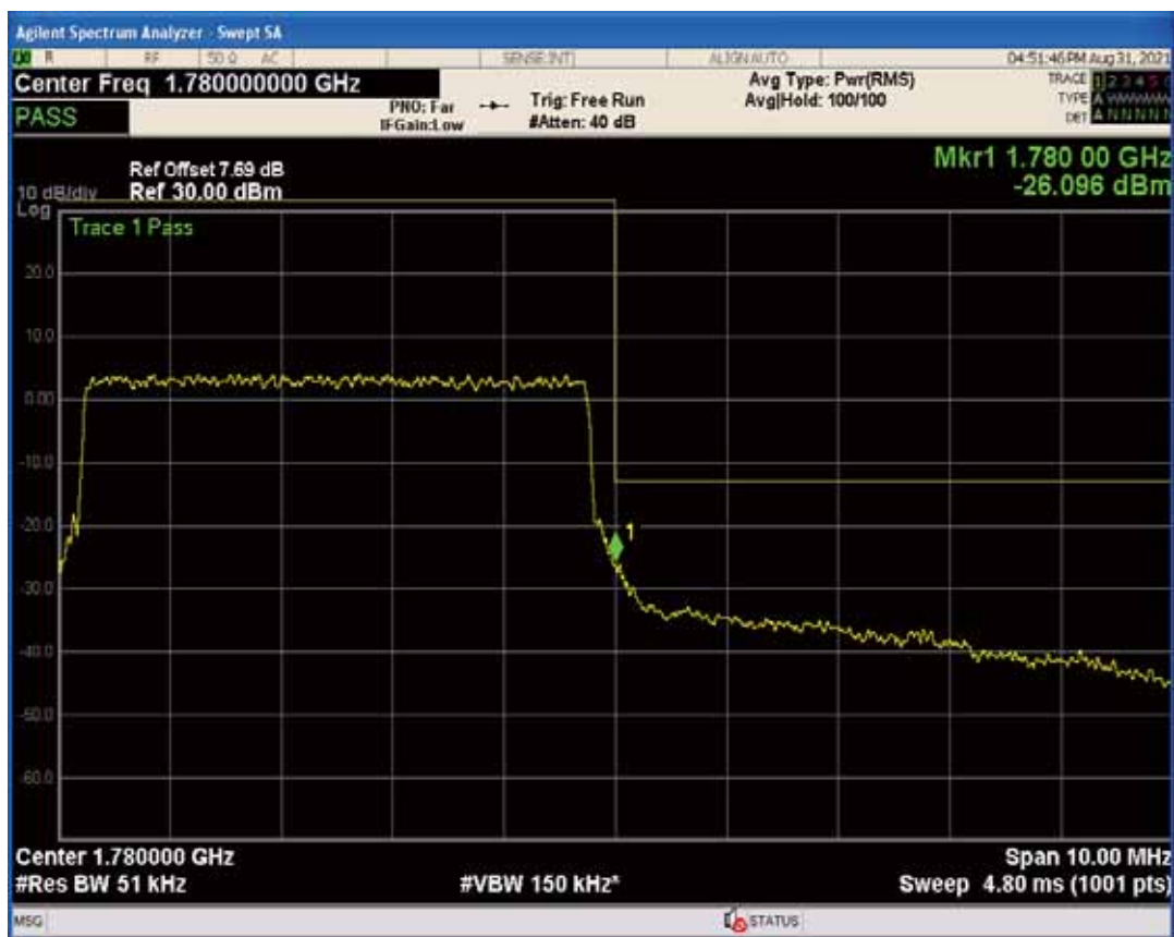
Band66 QAM16 BW=5MHz Channel=132647 RB Size=1 Position=#Max
