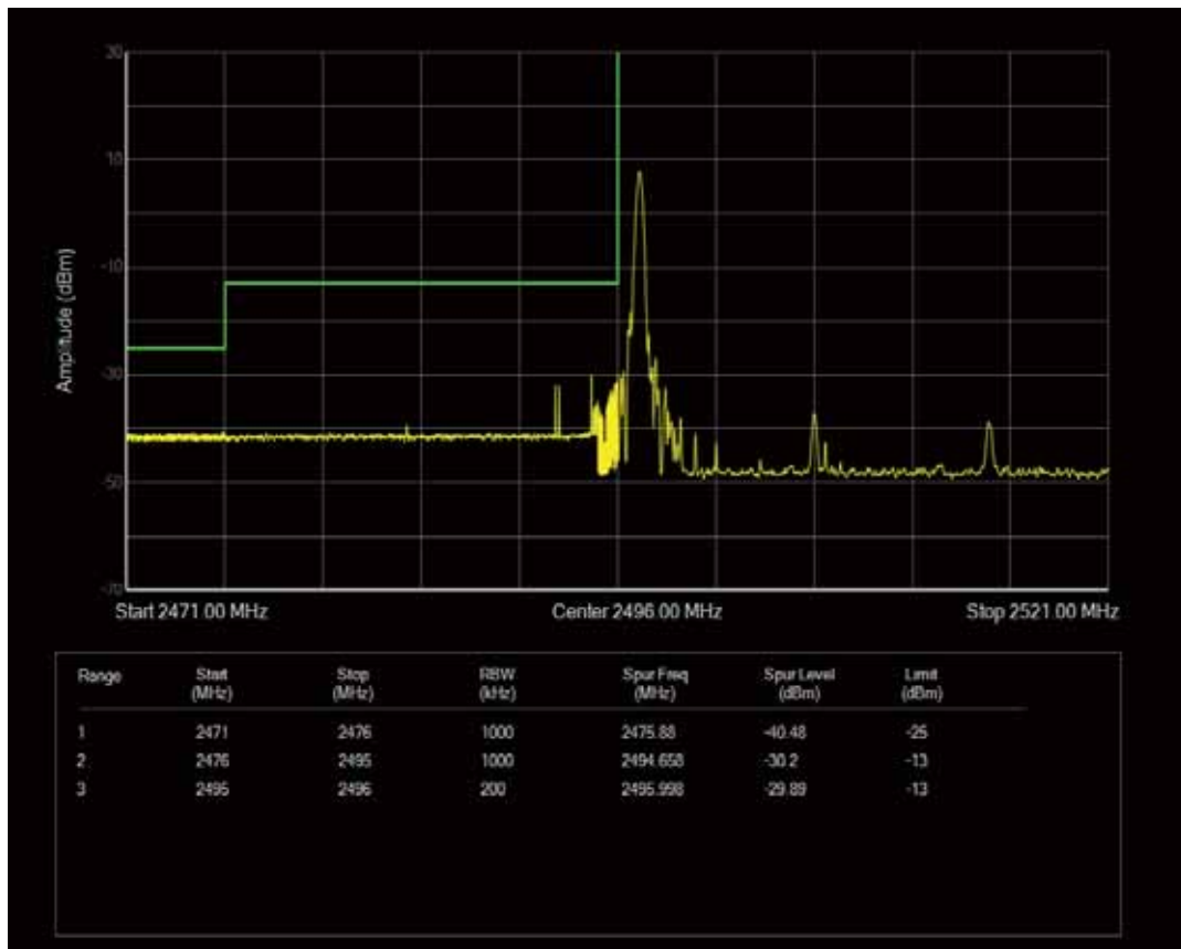
Band41 QPSK BW=20MHz Channel=39750 RB Size=100 Position=#0
