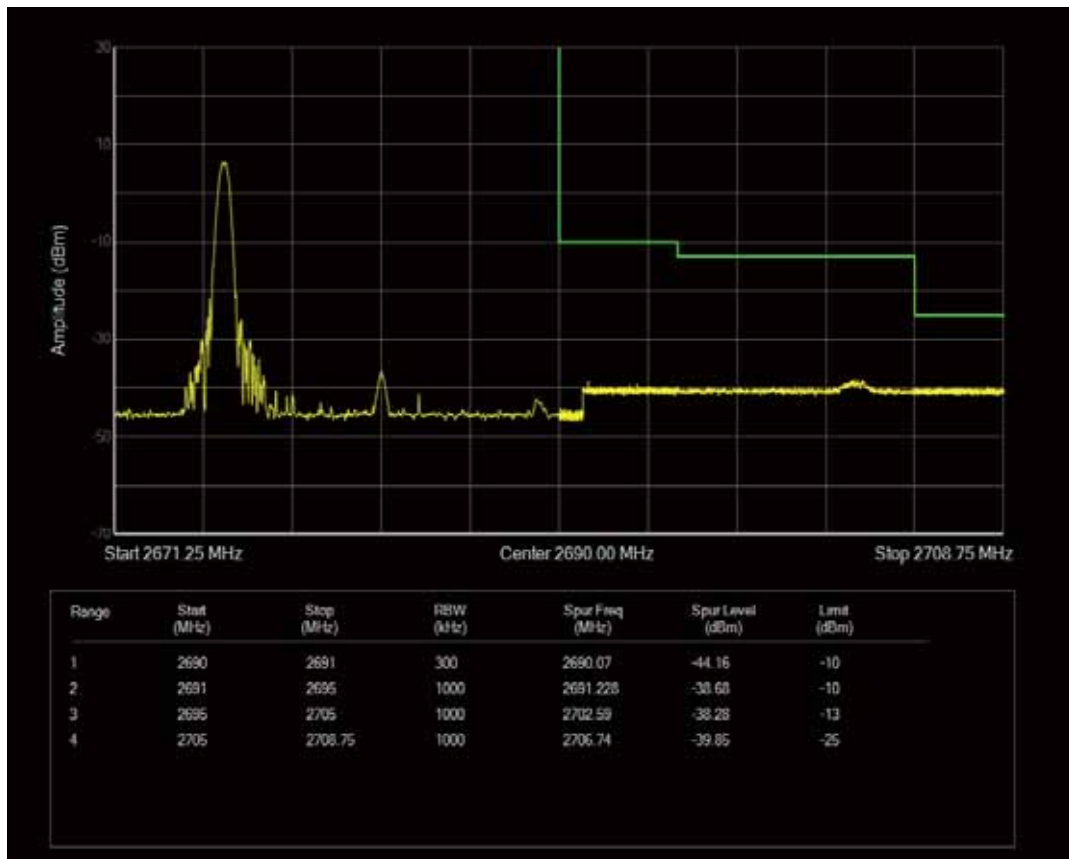
Band41 QAM16 BW=15MHz Channel=41515 RB Size=1 Position=#Max
