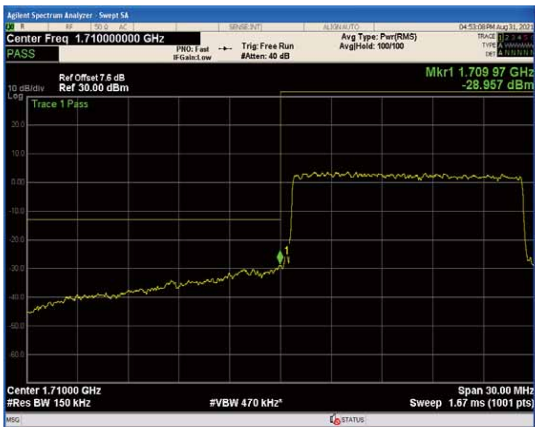
Band66 QPSK BW=15MHz Channel=132597 RB Size=1 Position=#0
