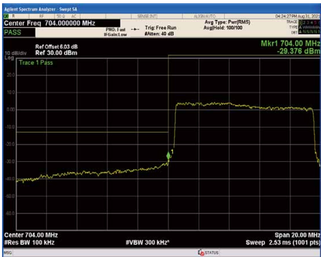
Band17 QPSK BW=10MHz Channel=23800 RB Size=1 Position=#Max
