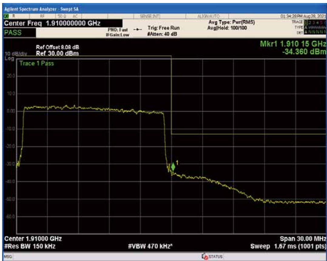
Band2 QPSK BW=20MHz Channel=18700 RB Size=1 Position=#Max
