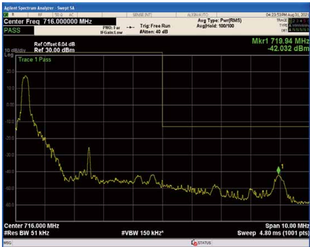
Band17 QPSK BW=5MHz Channel=23825 RB Size=25 Position=#0
