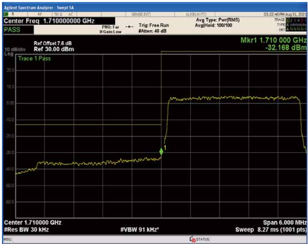
Band4 QPSK BW=3MHz Channel=19965 RB Size=1 Position=#Max
