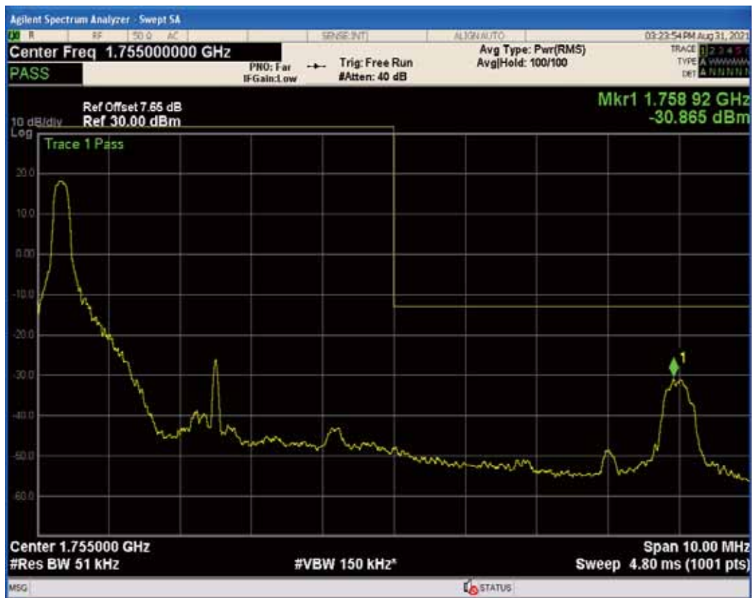
Band4 QPSK BW=5MHz Channel=20375 RB Size=1 Position=#Max
