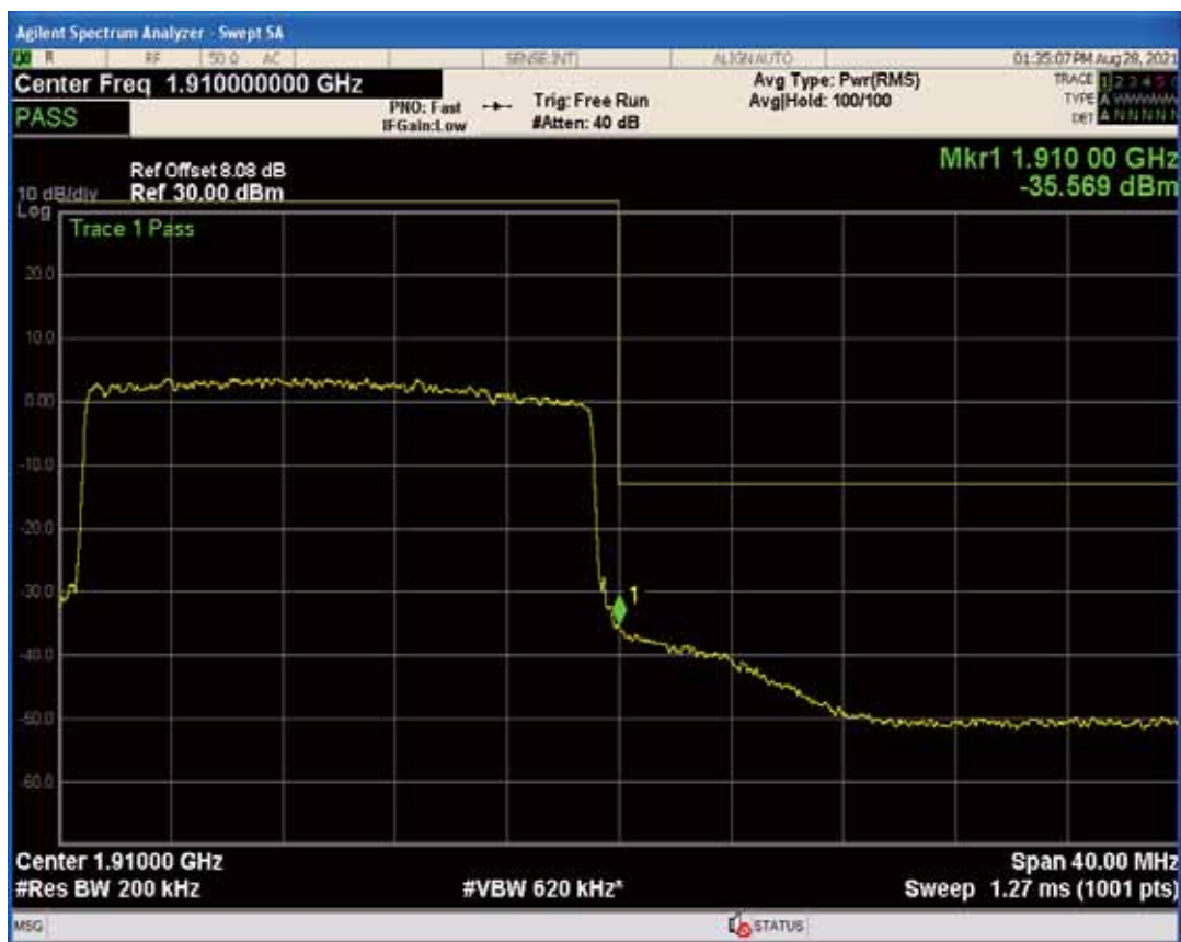
Band2 QAM16 BW=20MHz Channel=19100 RB Size=1 Position=#0
