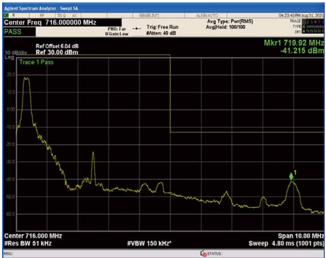
Band17 QPSK BW=5MHz Channel=23825 RB Size=1 Position=#Max
