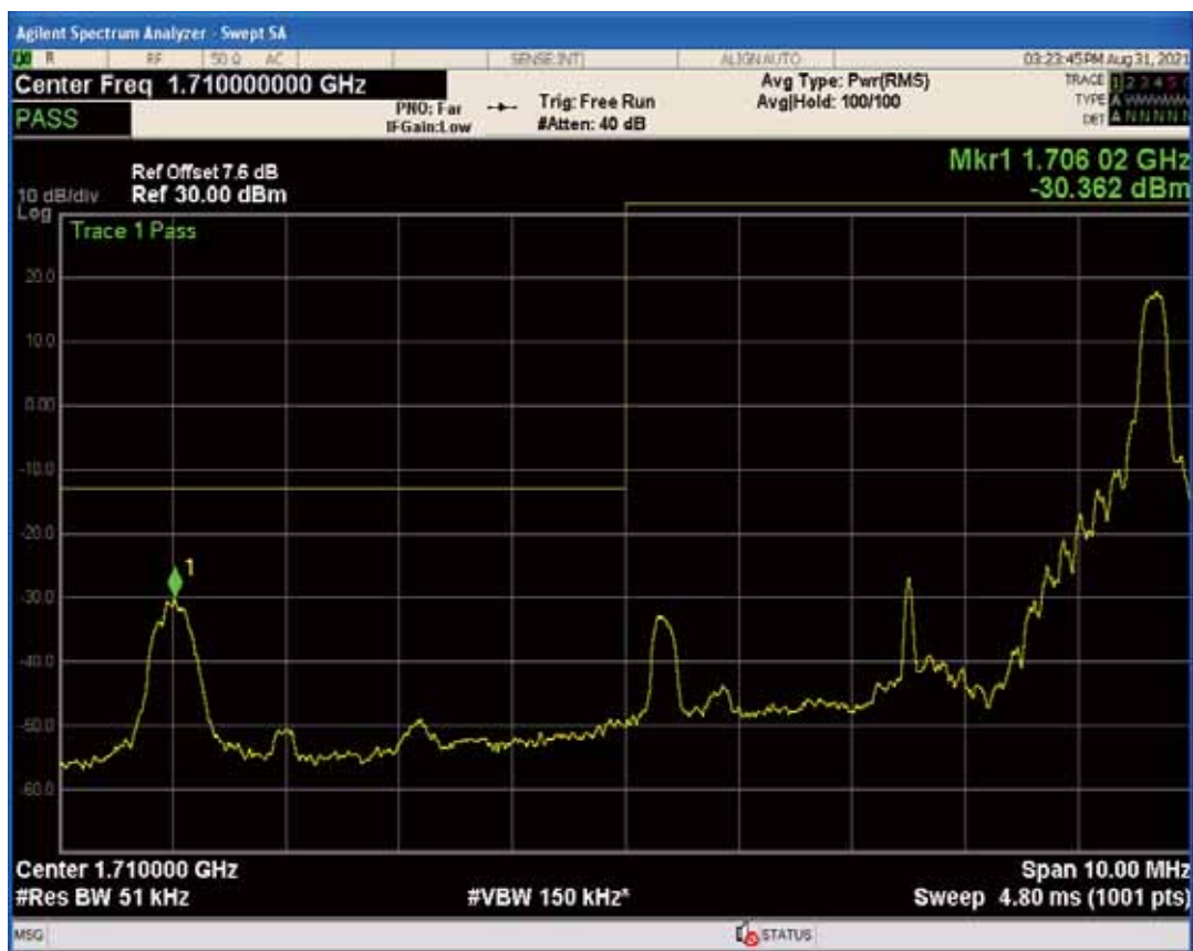
Band4 QAM16 BW=5MHz Channel=19975 RB Size=25 Position=#0
