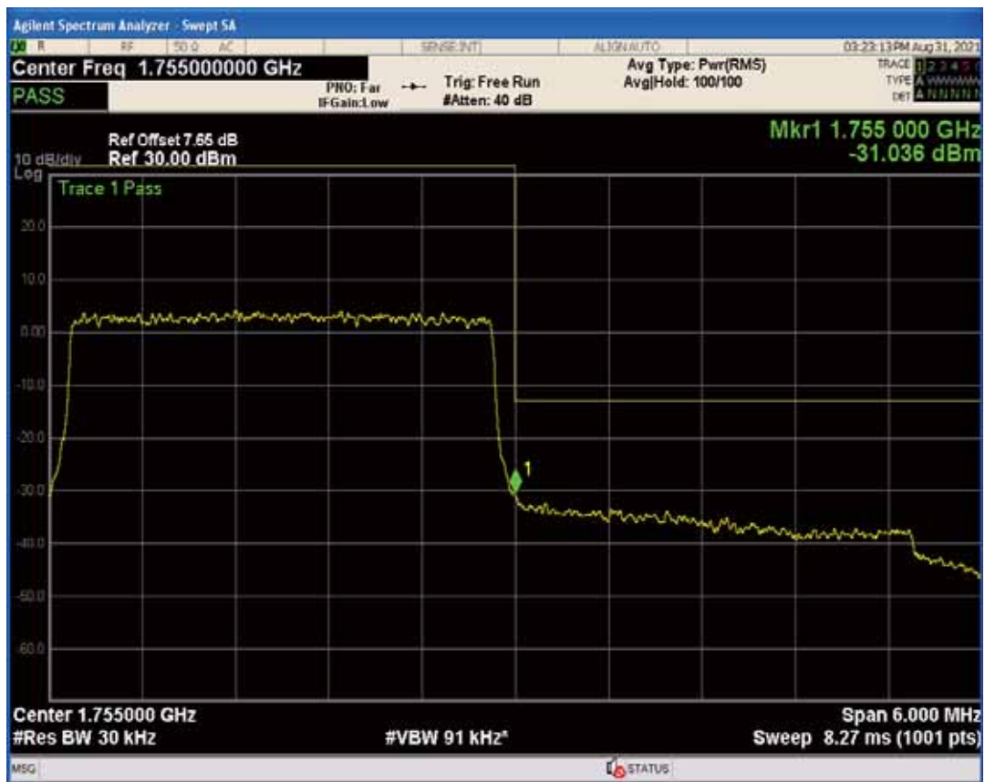
Band4 QAM16 BW=3MHz Channel=20385 RB Size=1 Position=#0
