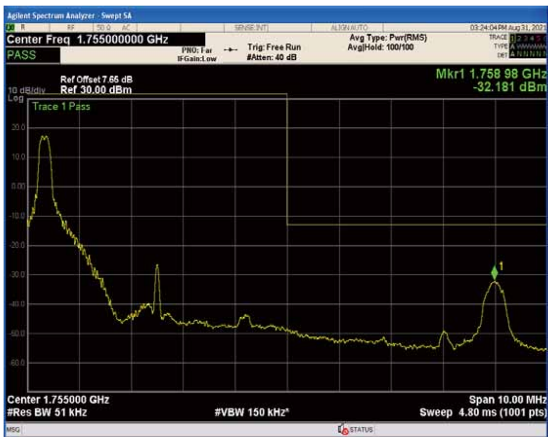
Band4 QAM16 BW=5MHz Channel=20375 RB Size=1 Position=#Max
