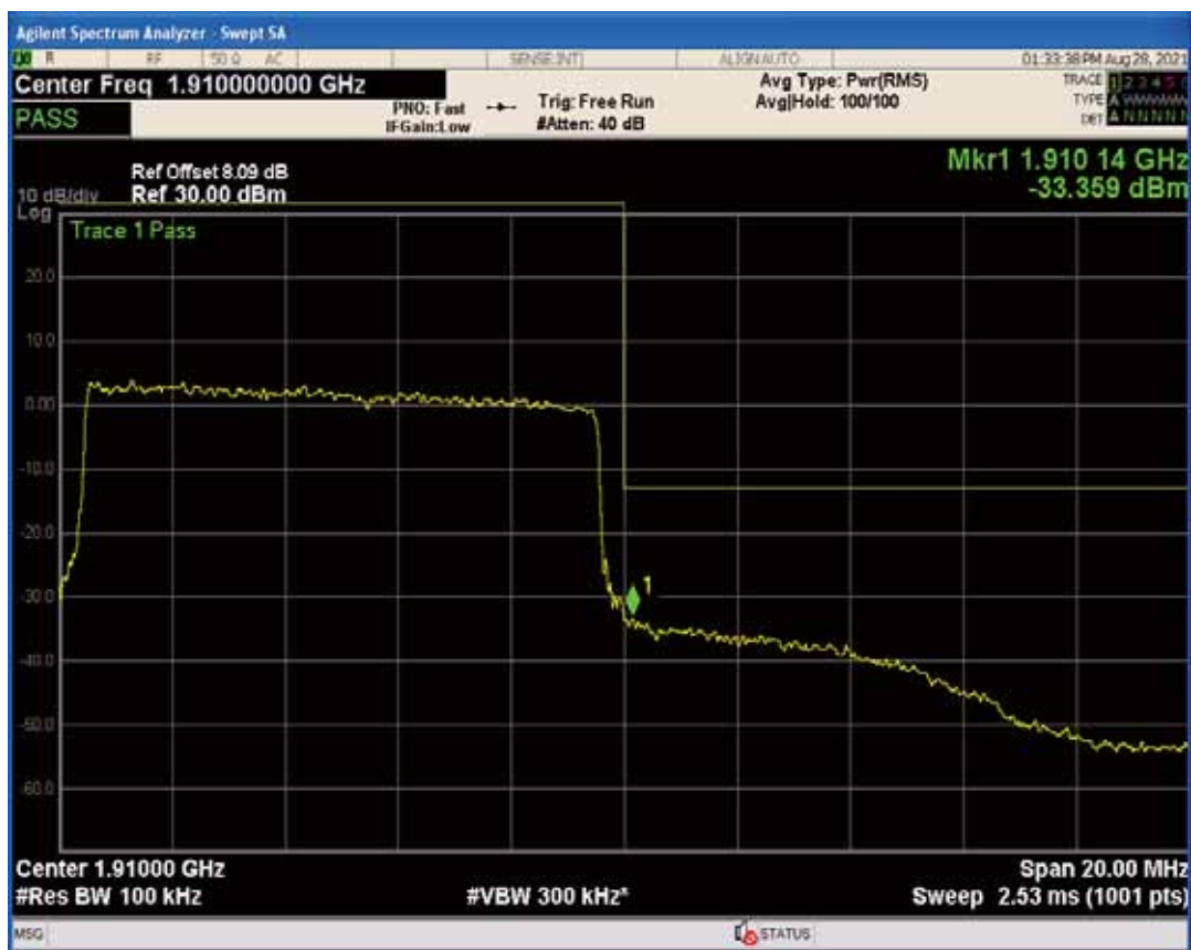
Band2 QAM16 BW=10MHz Channel=19150 RB Size=1 Position=#Max
