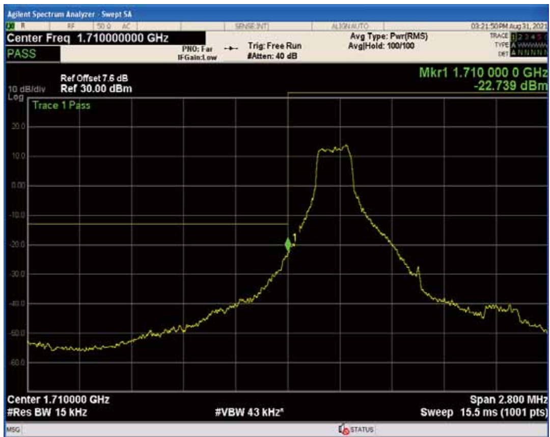
Band4 QPSK BW=1.4MHz Channel=19957 RB Size=6 Position=#0
