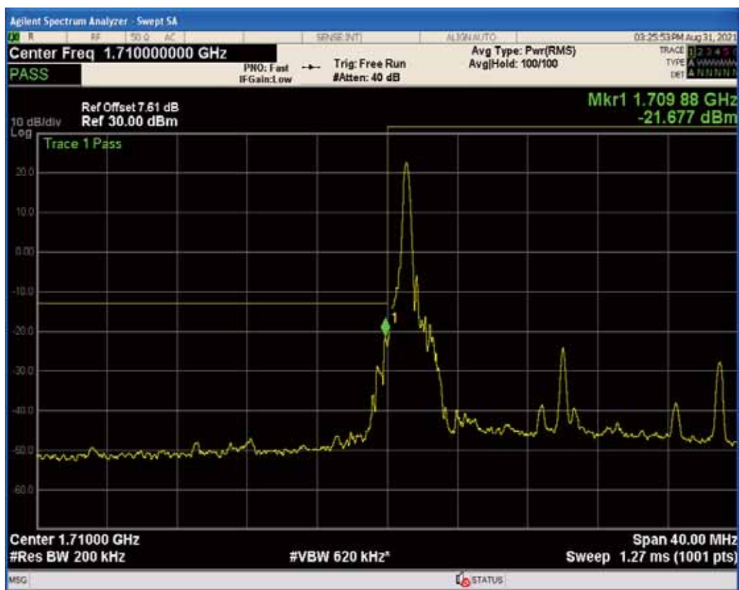
Band4 QAM16 BW=15MHz Channel=20325 RB Size=75 Position=#0
