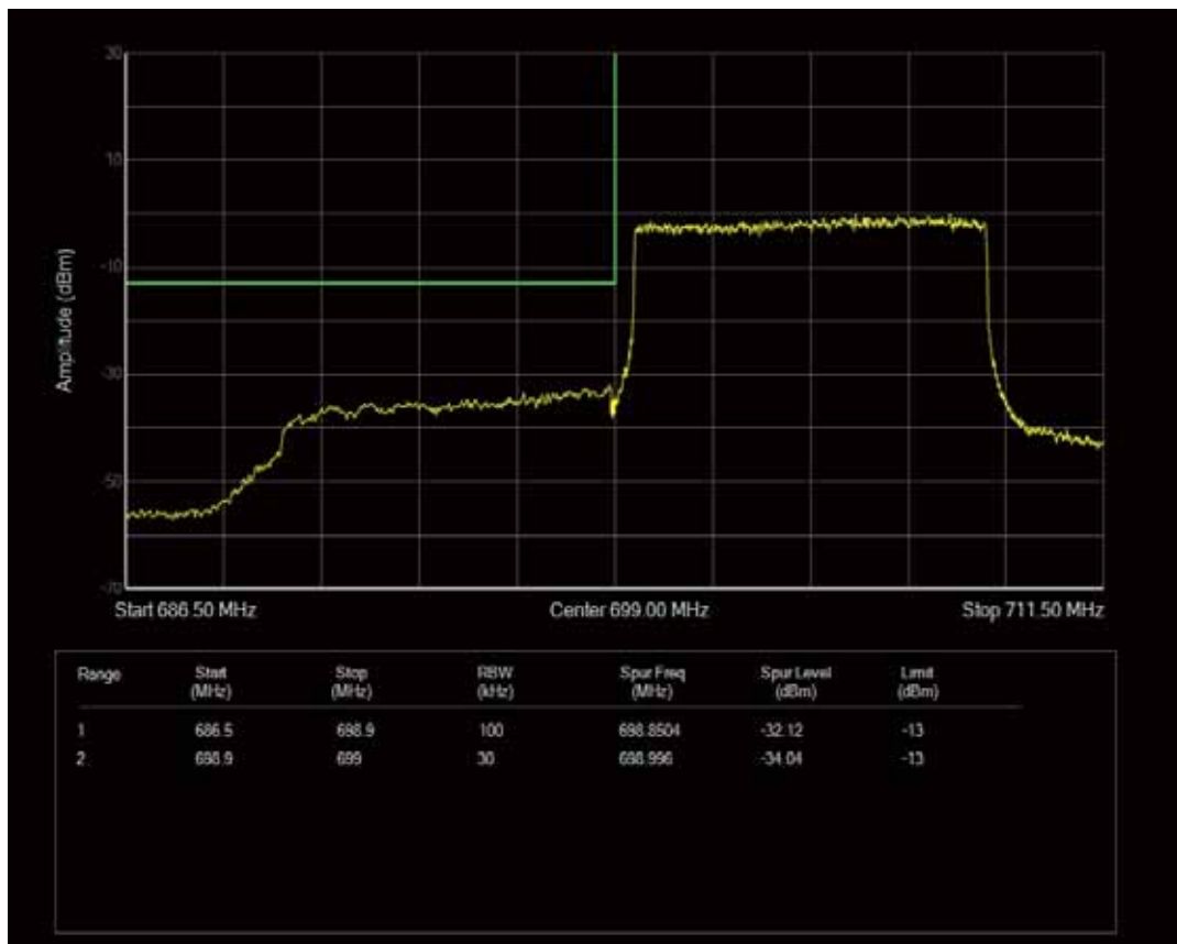
Band12 QAM16 BW=10MHz Channel=23060 RB Size=1 Position=#Max
