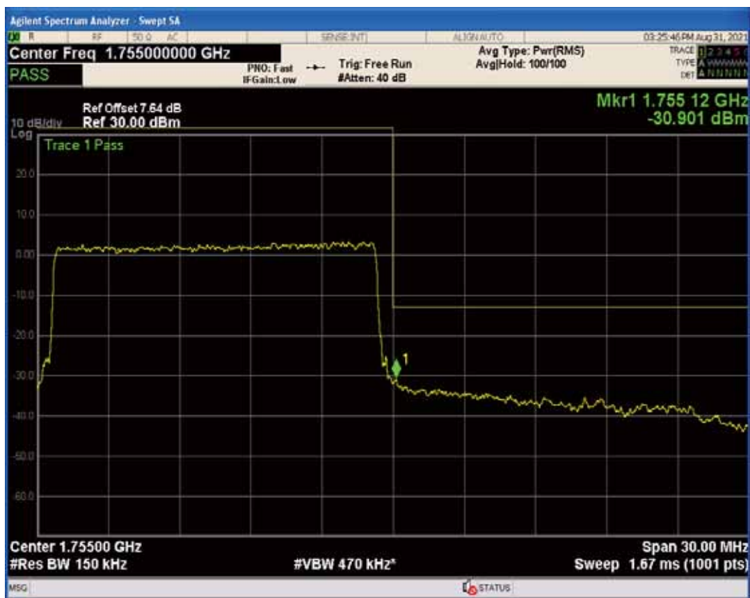
Band4 QPSK BW=20MHz Channel=20050 RB Size=1 Position=#Max
