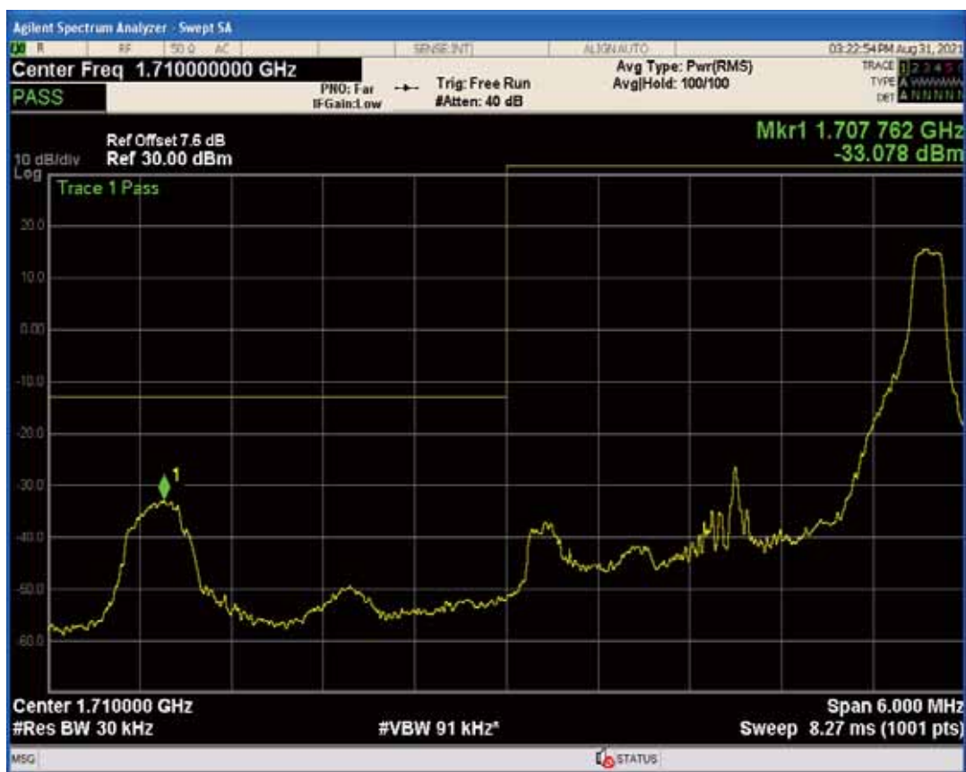
Band4 QAM16 BW=3MHz Channel=19965 RB Size=1 Position=#0
