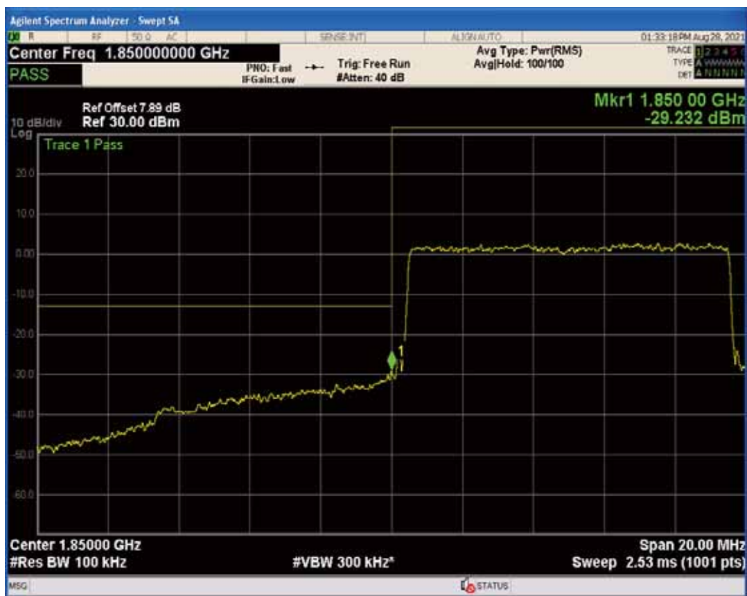
Band2 QPSK BW=10MHz Channel=19150 RB Size=50 Position=#0
