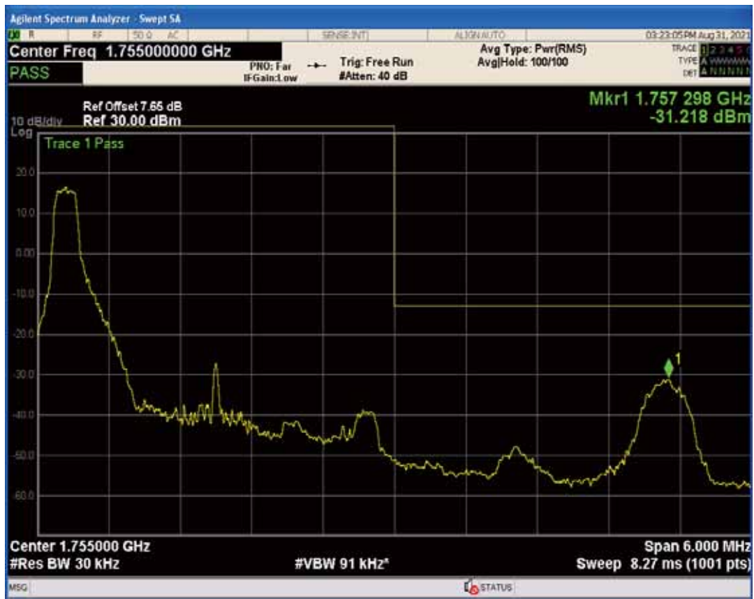
Band4 QPSK BW=3MHz Channel=20385 RB Size=15 Position=#0
