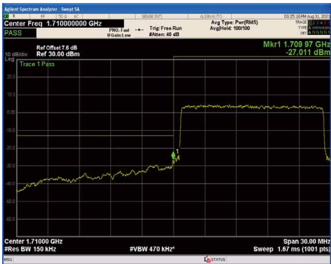
Band4 QAM16 BW=15MHz Channel=20025 RB Size=1 Position=#0
