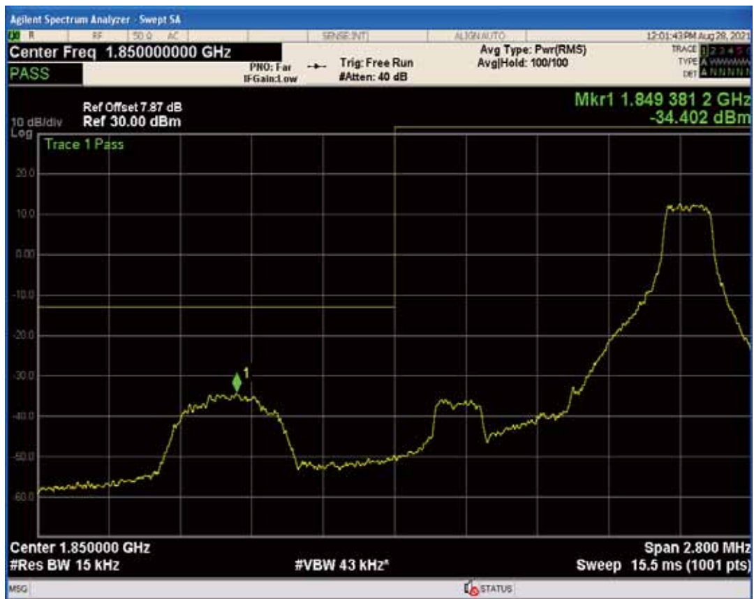
Band2 QAM16 BW=1.4MHz Channel=18607 RB Size=6 Position=#0
