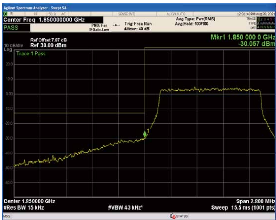
Band2 QPSK BW=1.4MHz Channel=19193 RB Size=1 Position=#0
