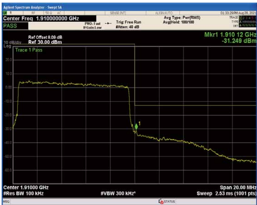
Band2 QPSK BW=10MHz Channel=19150 RB Size=1 Position=#Max
