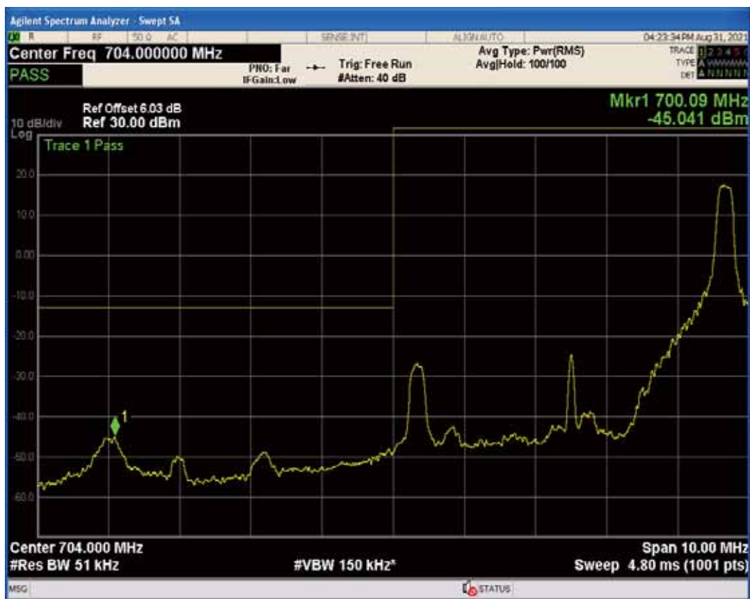
Band17 QAM16 BW=5MHz Channel=23755 RB Size=25 Position=#0
