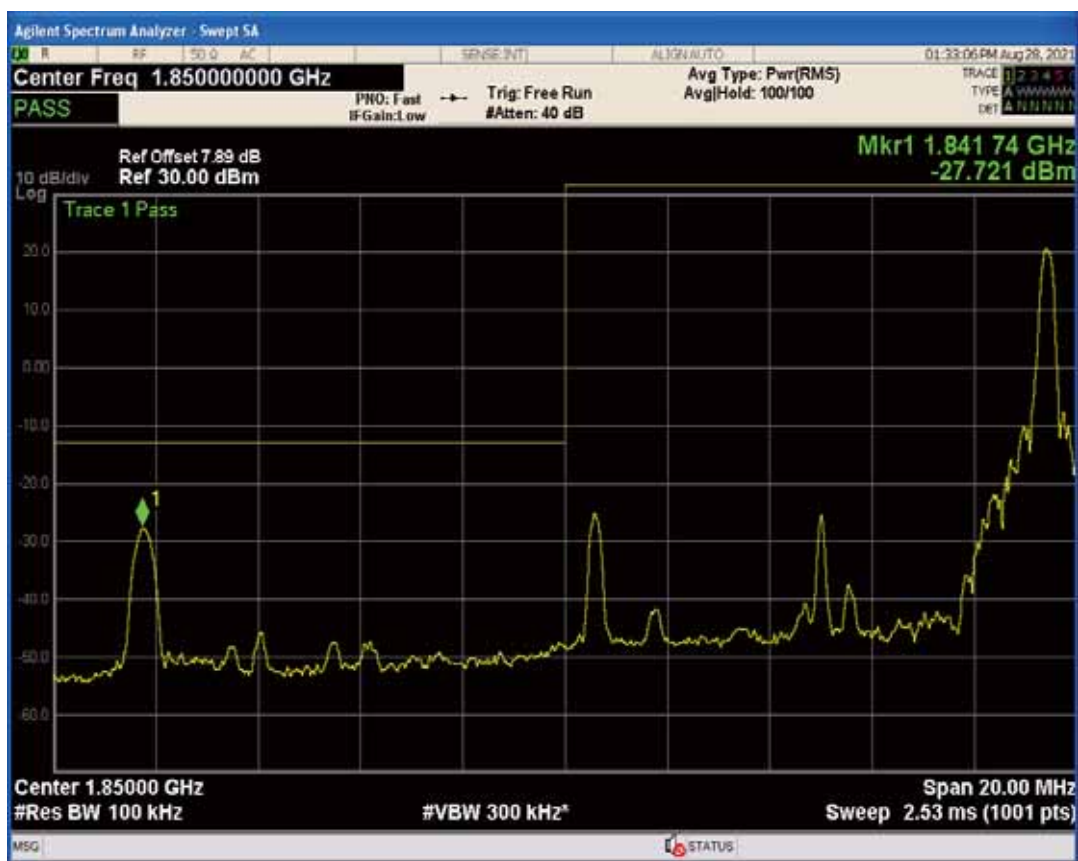
Band2 QPSK BW=10MHz Channel=18650 RB Size=50 Position=#0
