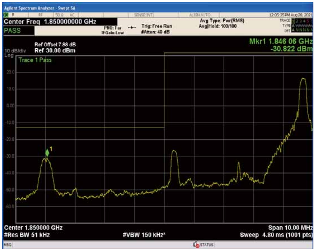
Band2 QAM16 BW=5MHz Channel=18625 RB Size=25 Position=#0
