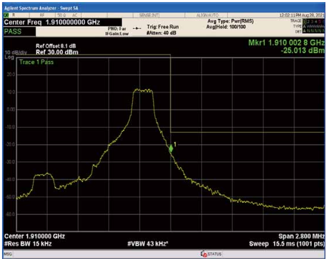
Band2 QPSK BW=3MHz Channel=18615 RB Size=1 Position=#0
