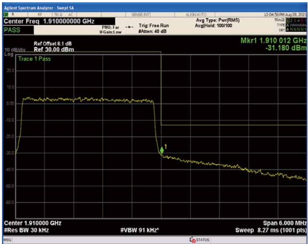
Band2 QAM16 BW=3MHz Channel=19185 RB Size=1 Position=#0
