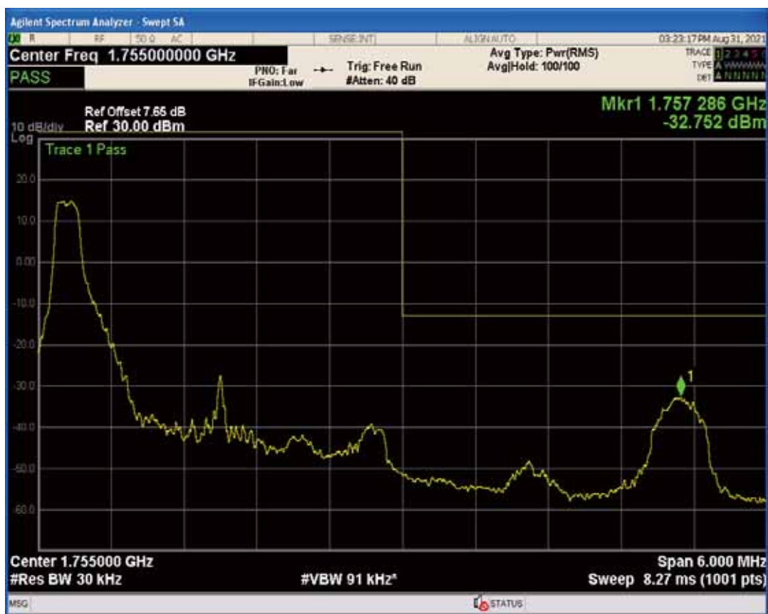
Band4 QAM16 BW=3MHz Channel=20385 RB Size=1 Position=#Max
