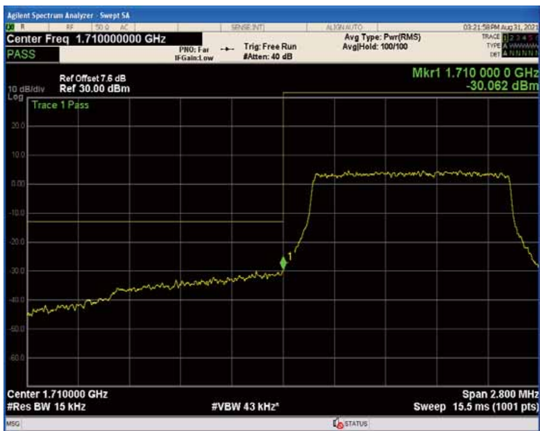
Band4 QPSK BW=1.4MHz Channel=20393 RB Size=1 Position=#0
