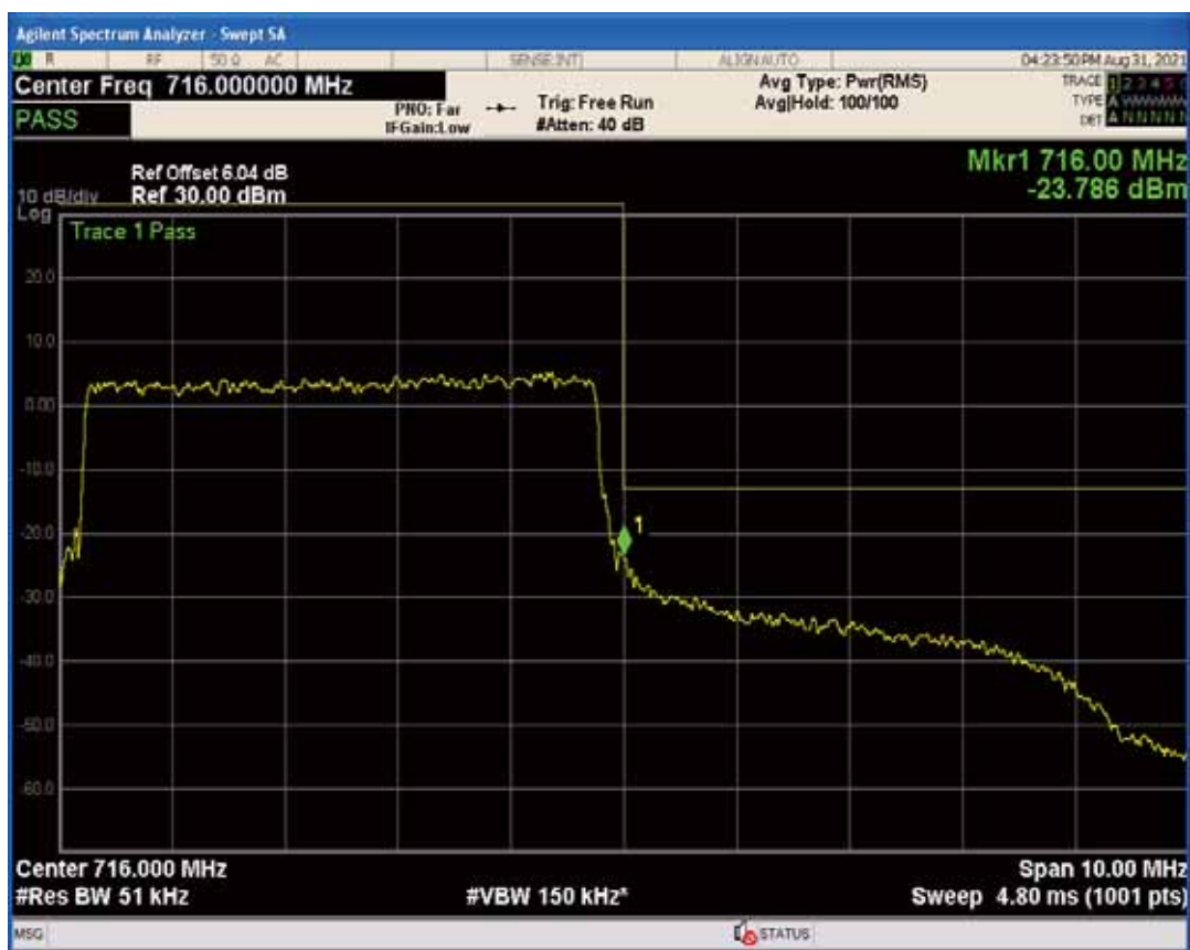
Band17 QAM16 BW=5MHz Channel=23825 RB Size=25 Position=#0
