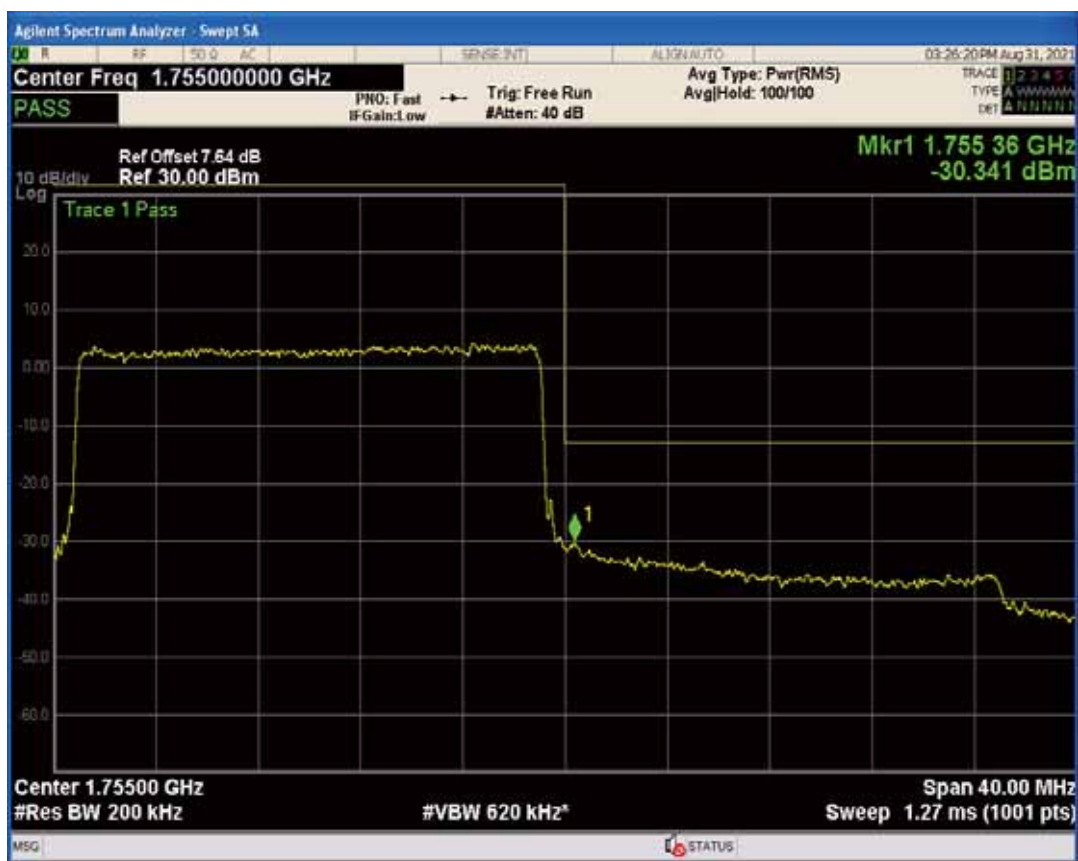
Band4 QPSK BW=20MHz Channel=20300 RB Size=1 Position=#Max
