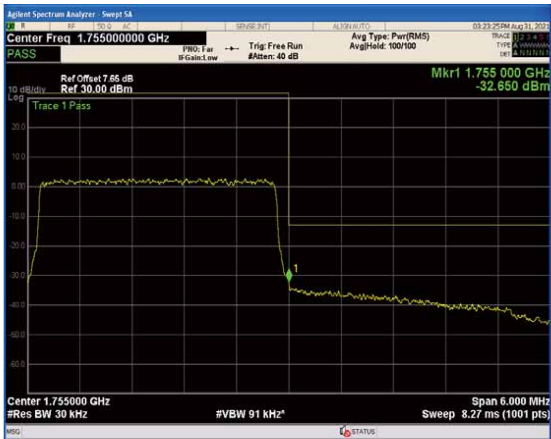
Band4 QPSK BW=5MHz Channel=19975 RB Size=1 Position=#Max
