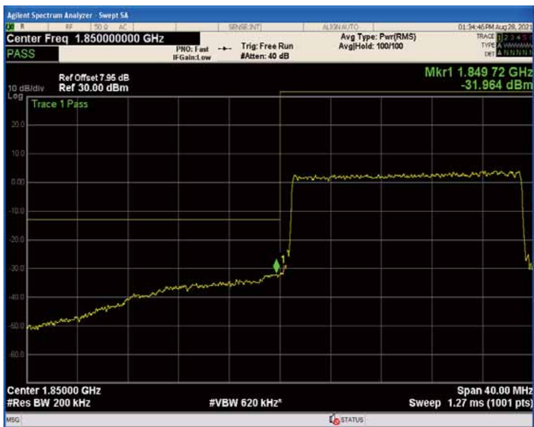
Band2 QAM16 BW=20MHz Channel=18700 RB Size=1 Position=#Max
