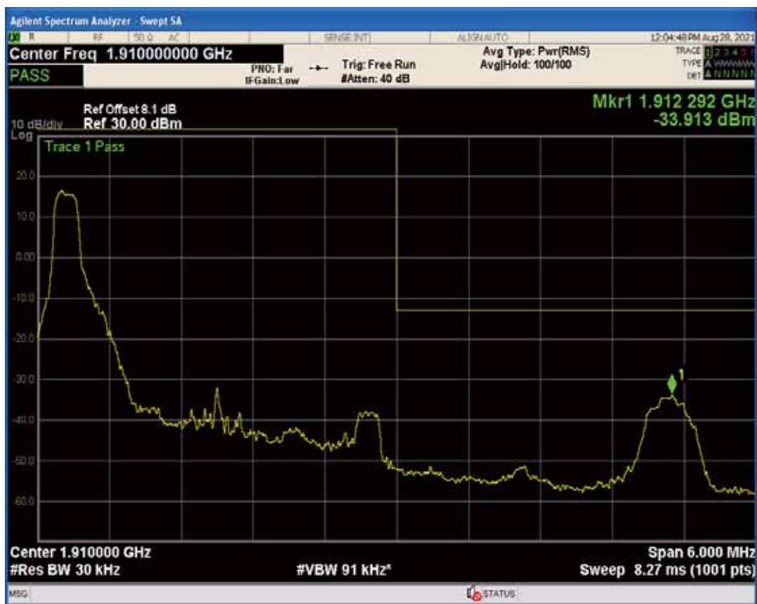
Band2 QPSK BW=3MHz Channel=19185 RB Size=1 Position=#Max
