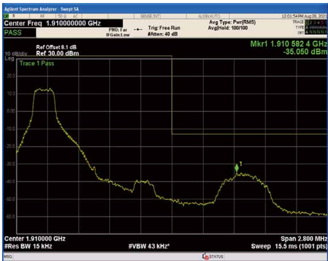
Band2 QPSK BW=1.4MHz Channel=19193 RB Size=1 Position=#Max
