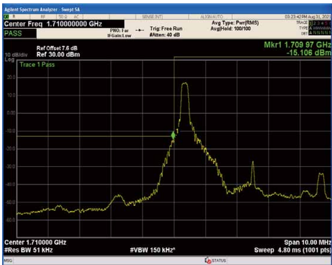
Band4 QAM16 BW=5MHz Channel=19975 RB Size=1 Position=#Max
