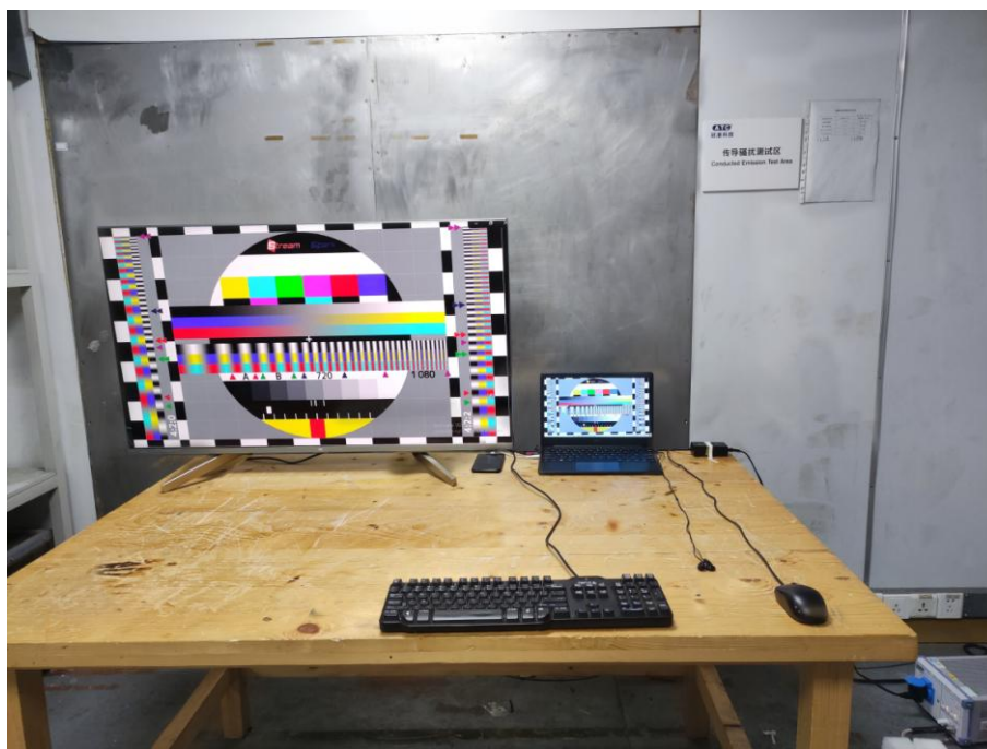
Photo of Conducted Emission Measurement
