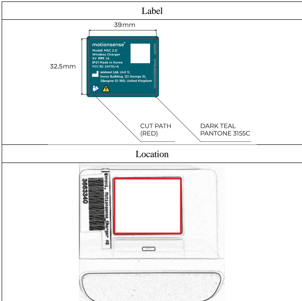
\* This label is attached to the front of the product and not easily removed.
