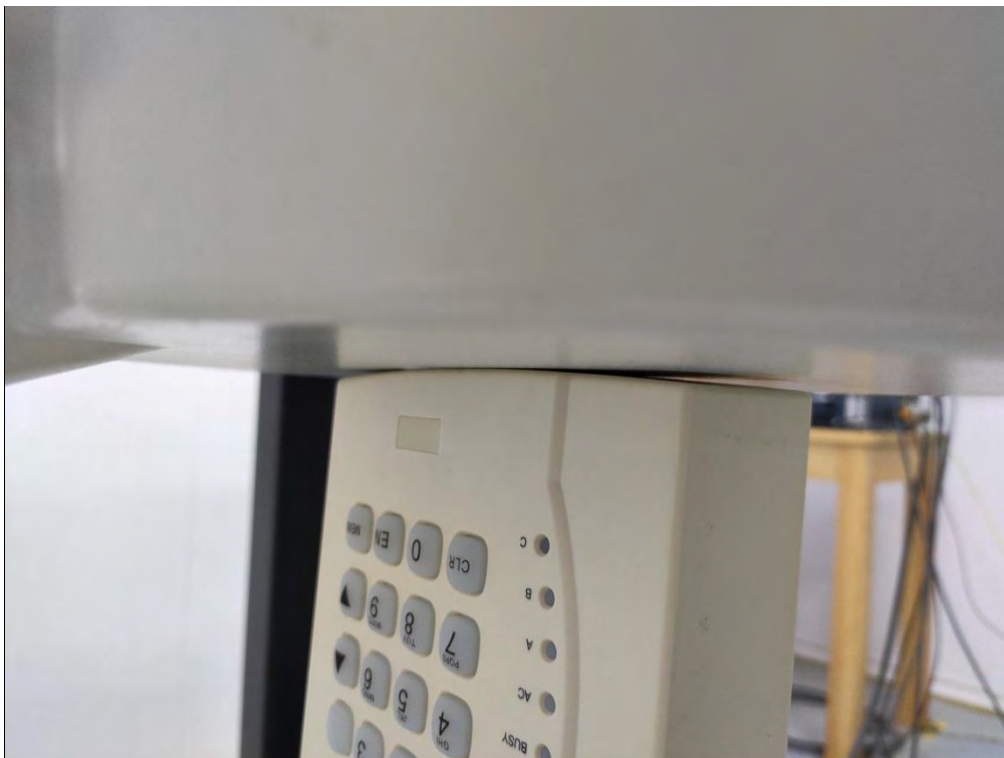
0mm body-worn Bottom Side Setup Photo (hotspot)
