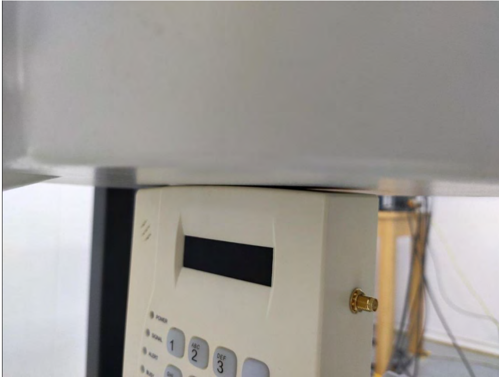
0mm body-worn Top Side Setup Photo (hotspot)
