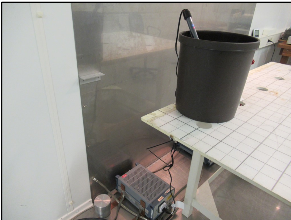
Photo 2: Conducted Test Setup from 150 kHz to 30 MHz
