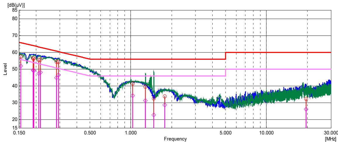
*Note: The plots show the max hold (peak detector) pre-scan results measured. Blue graph represents the result of the N-Line; green graph - the results for L1-Line. The bar graphs indicate the final measurement result applying the dedicated detector at selected frequencies for each limit line (red cycle for quasi peak limit; violet cycle for average limit).*
