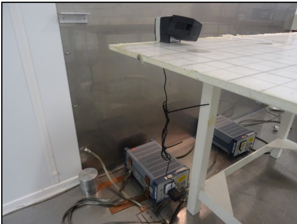
Photo 2: Conducted Test Setup from 150 kHz to 30 MHz
