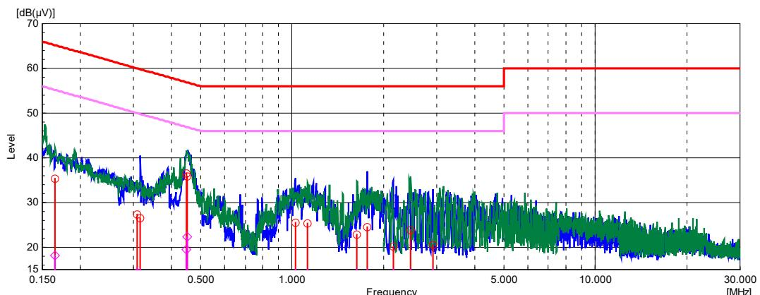
Note: The plots show the max hold (peak detector) pre-scan results measured. Blue graph represents the result of the N-Line; green graph - the results for L1-Line. The bar graphs indicate the final measurement result applying the dedicated detector at selected frequencies for each limit line (red cycle for quasi peak limit; violet cycle for average limit).
