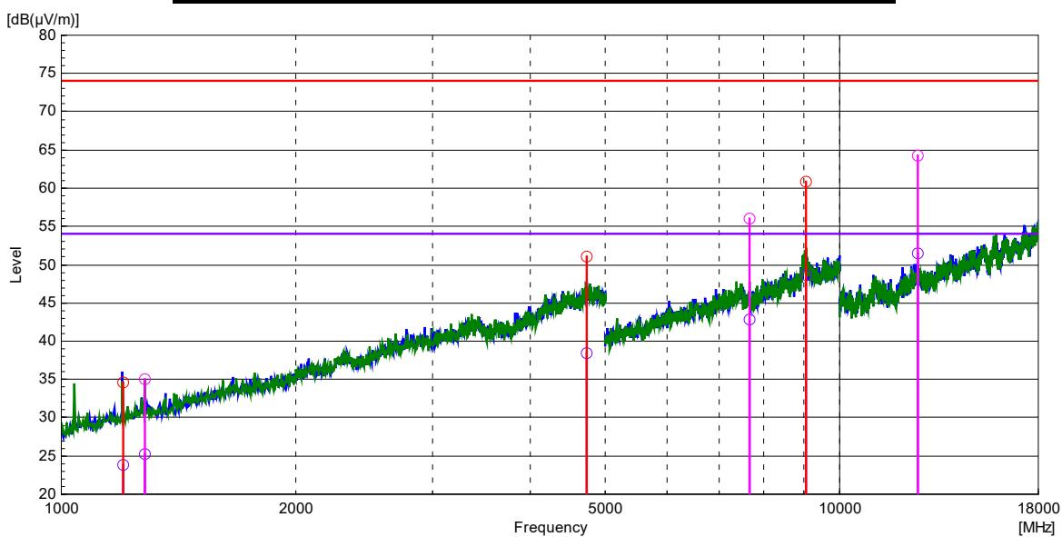
Note: The plots show the max hold (peak detector) pre-scan results measured while rotating the TT continuously and an antenna movement between 1 – 4m height. Blue graph represents the result of the horizontal antenna polarization; green graph the results measured with vertical antenna polarization. The bar graphs indicate the final measurement result applying the dedicated detector at selected frequencies for each limit line (red cycle for peak limit; violet cycle for average limit).
