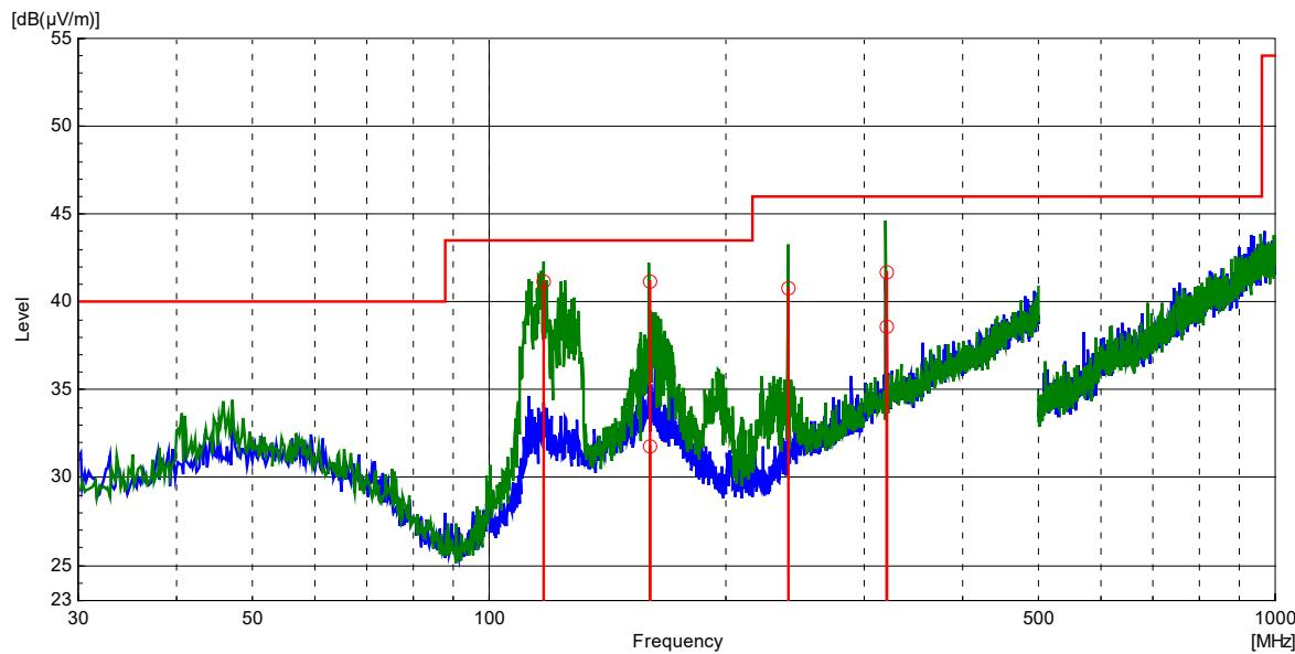
*Note: The plots show the max hold (peak detector) pre-scan results measured while rotating the TT continuously and an antenna movement between 1 – 4m height. Blue graph represents the result of the horizontal antenna polarization; green graph the results measured with vertical antenna polarization. The bar graphs indicate the final measurement result applying the detector at selected frequencies (red cycle for quasi peak limit).*
