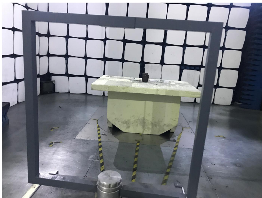
Radiation Emission Test Setup (Below 30MHz)
