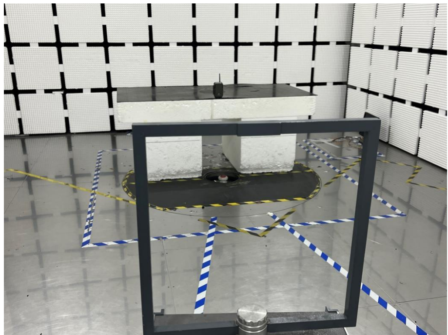
Radiation Emission Test Setup (Below 30MHz)
