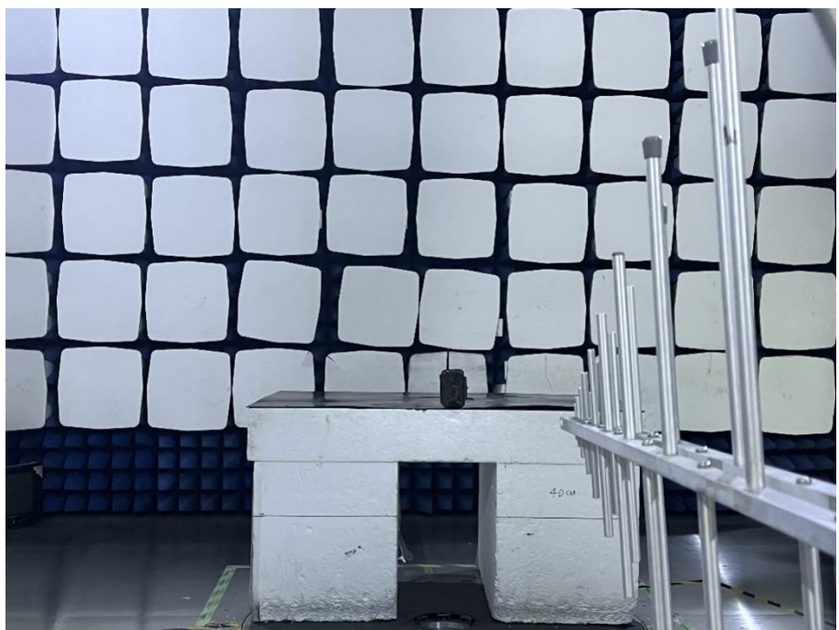
Radiation Emission Test Setup (30MHz to 1GHz)
