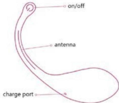
Turn off the device before charging. The cable can be compatible with any port or USB/AC power adapter for charging. It takes about 1.5 hours to get fully charged. The indicator light will flash when charging and will stay
