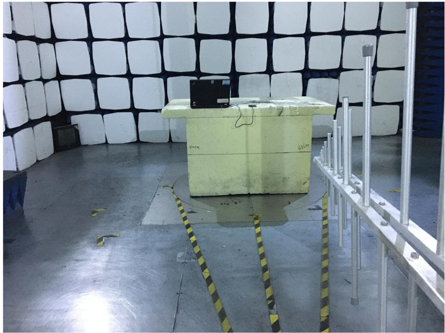
Radiation Emission Test Setup (30MHz to 1GHz)
