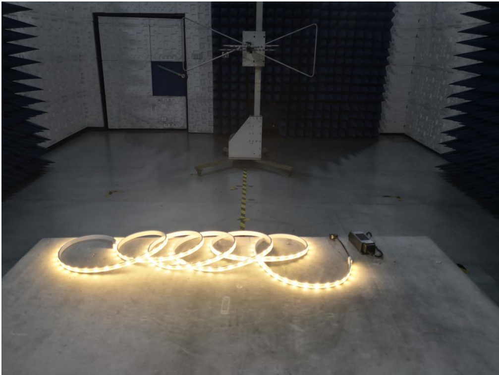
RADIATED EMISSION TEST SETUP ABOVE 1GHZ
