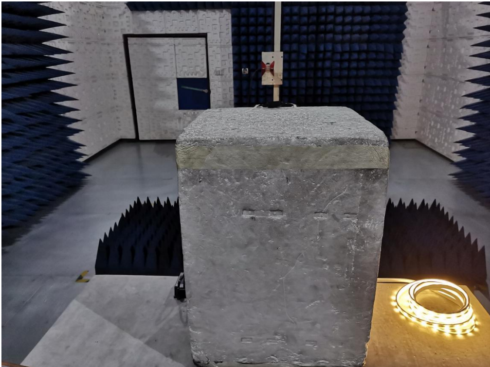
RADIATED EMISSION TEST SETUP ABOVE 1GHZ
