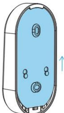
Press and slide up the panel. Install complete
