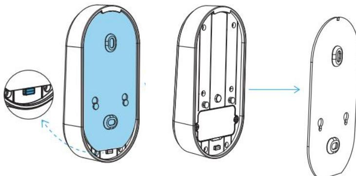
Press the button like the picture, and slide the panel.
