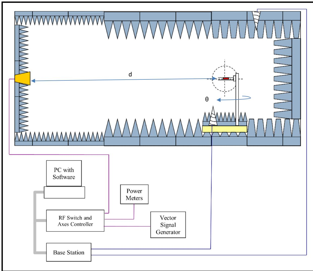
Measurements are performed using a spectrum analyzer. The dotted line around the EUT represents the 30cm diameter spherical quiet zone.
