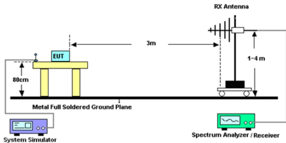
**For radiated test above 1GHz**
