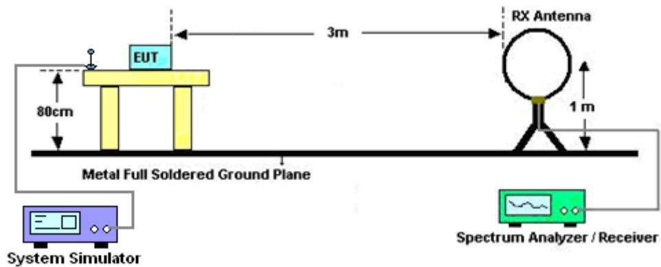
For radiated test from 30MHz to 1GHz
