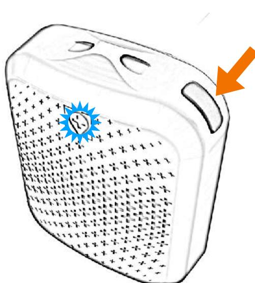
5.6. While blue LED is blinking, tap on update button to initiate firmware update for Tack GPS device.
