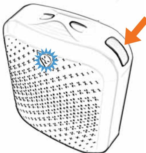
4.6. While blue LED is blinking, tap on update button to initiate firmware update for Tack GPS device.
