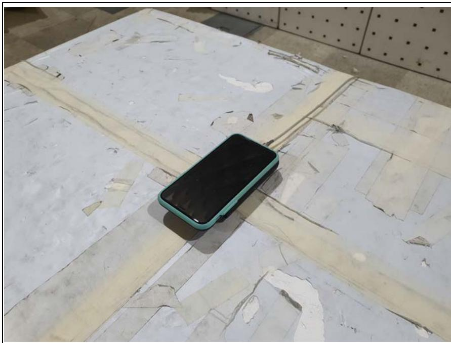
**2. Photo of Radiated Spurious Emission Test (9 kHz ~ 30 MHz)**
