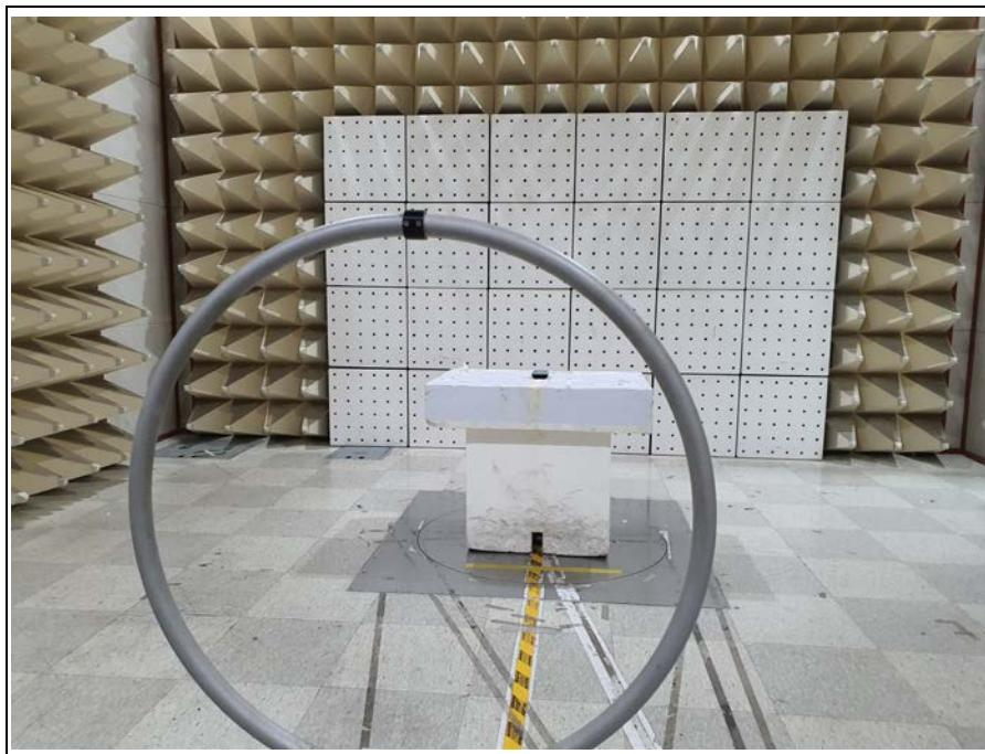
**3. Photo of Radiated Spurious Emission Test (30 MHz ~ 1 000 MHz)**
