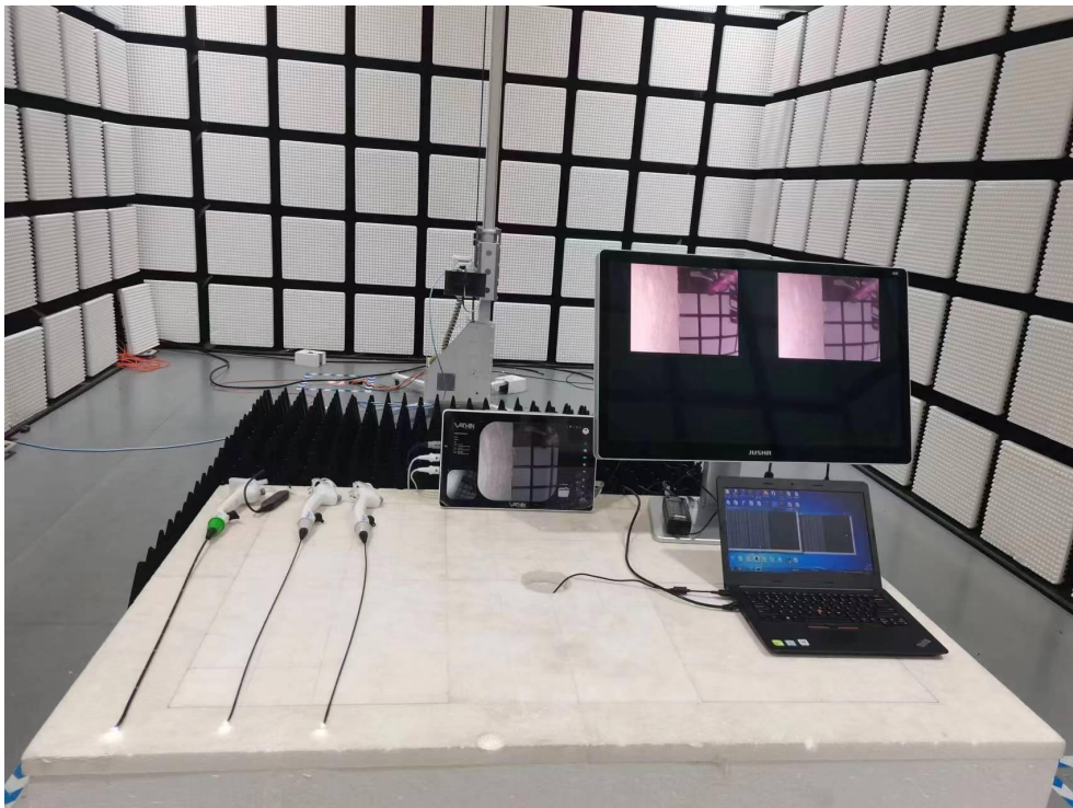
Fig. 2 Radiated emission setup photo(Above 1GHz)
