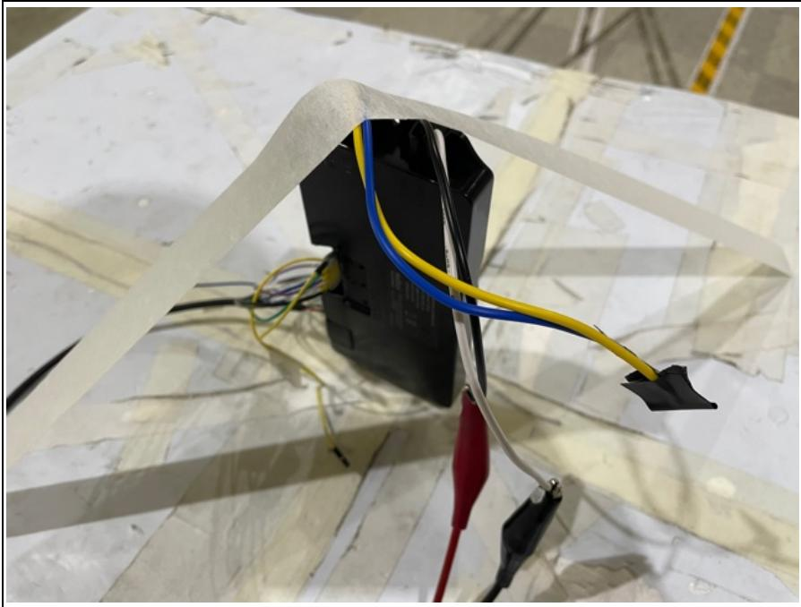
**2. Photo of Radiated Spurious Emission Test (Below 1 GHz)**
