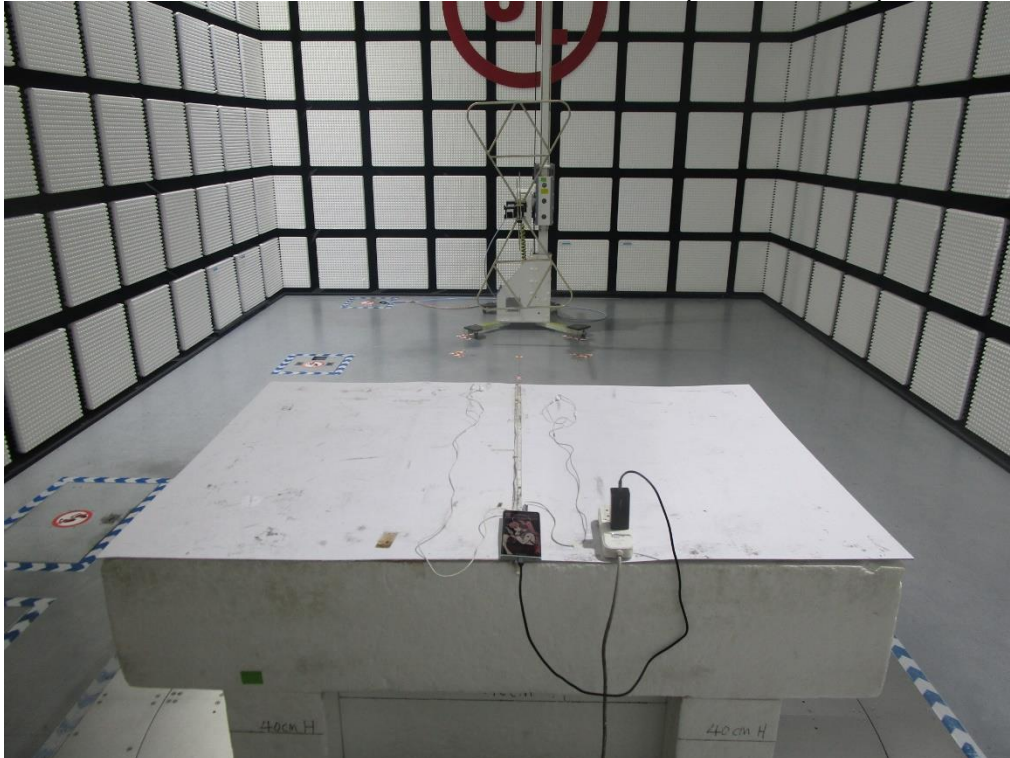
RADIATED RF MEASUREMENT SETUP (30MHz~1GHz)
