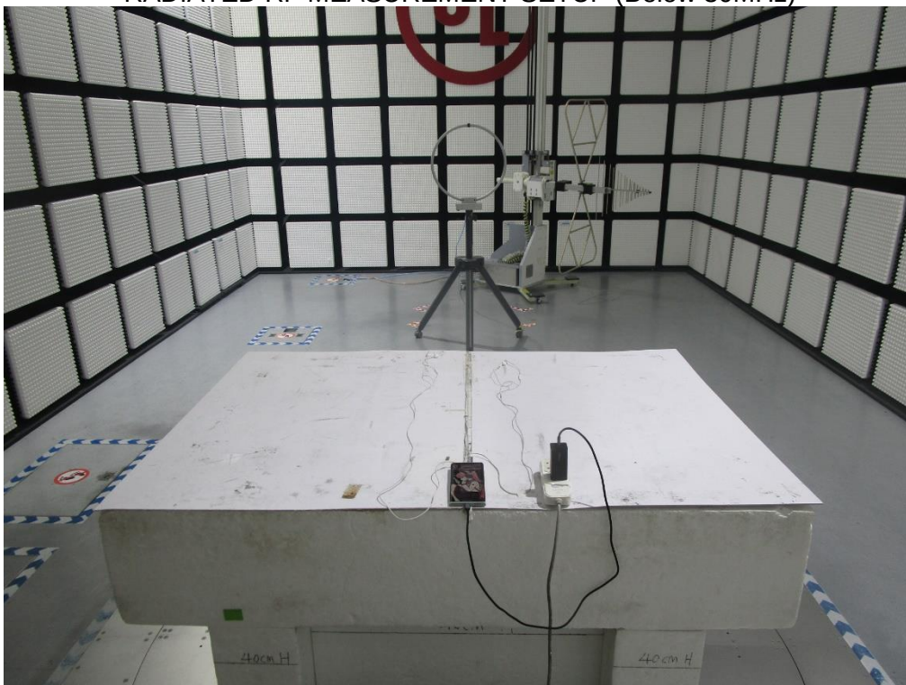
RADIATED RF MEASUREMENT SETUP (Below 30MHz)
