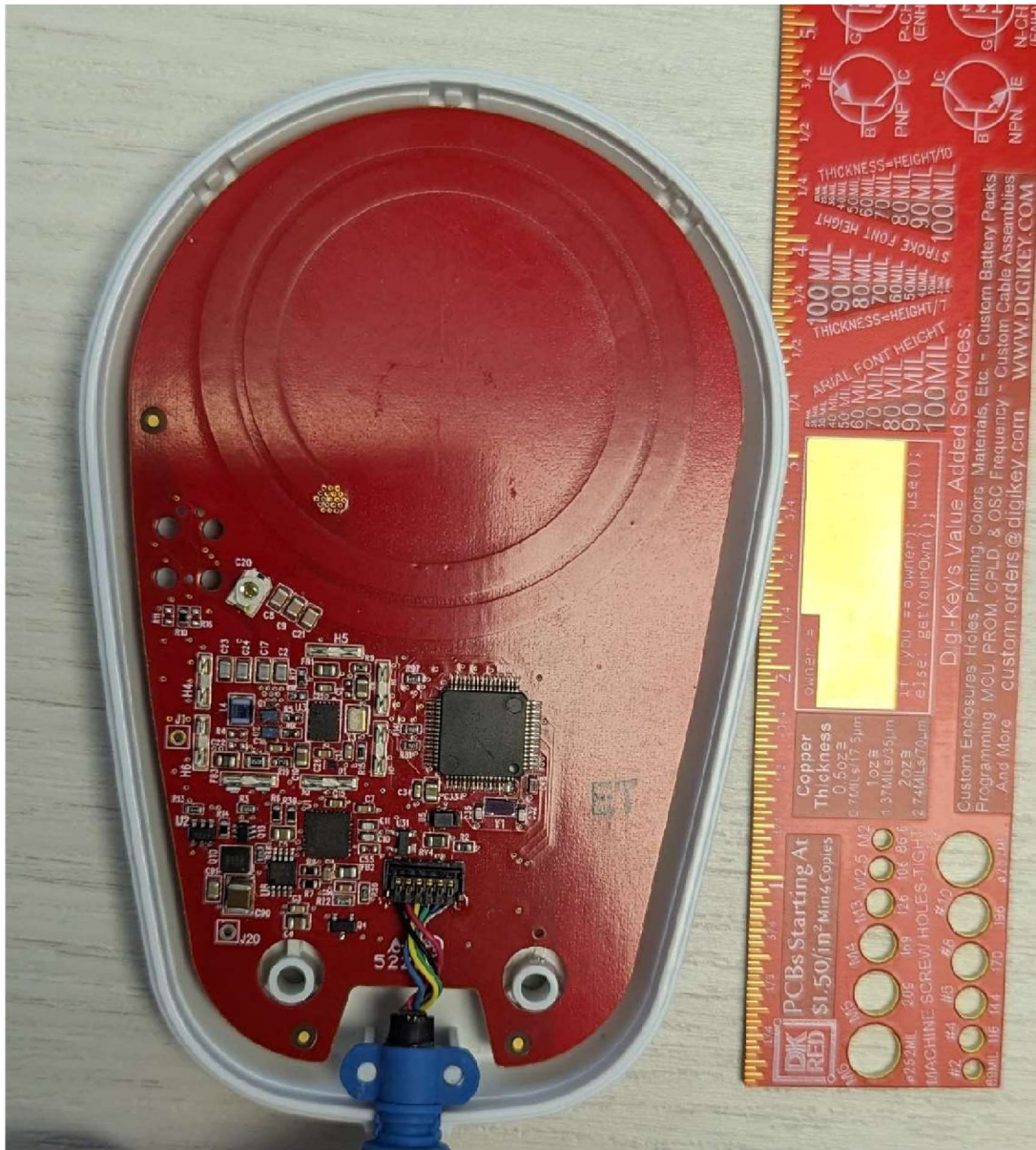
Internal Picture 1: Bottom PCB layout of the Intelio Programming Wand. 13.56MHz antenna is a PCB trace 2-turn coil.
