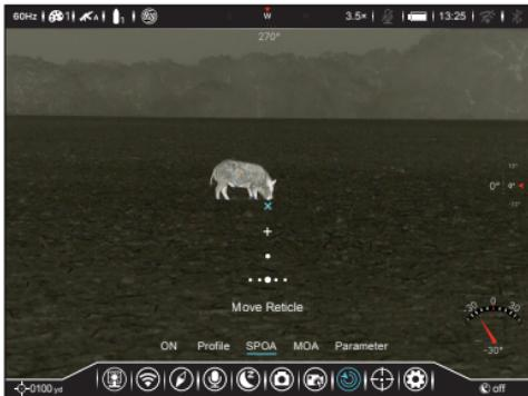
**NOTE:** When SPOA is set to Move Reticle, the HYBRID COMPACT will automatically move the original reticle to the suggested point of aim.
