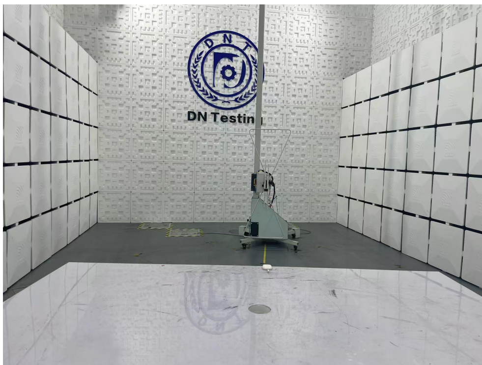
Radiated Emission Test View|(Below 1G)
