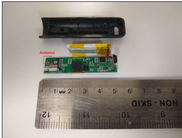
Internal Photo – EUT Antenna Placement
