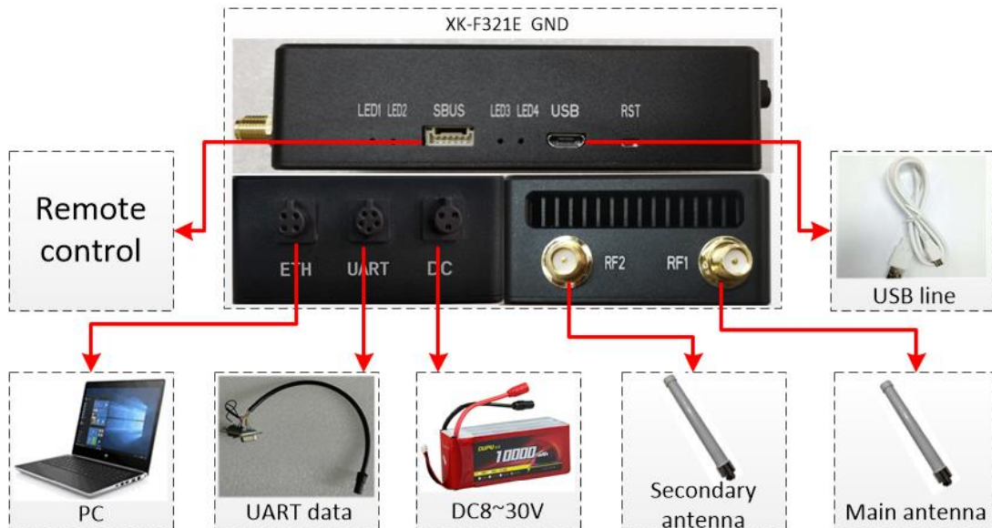
Figure 5.2 ground unit installation and connection diagram
