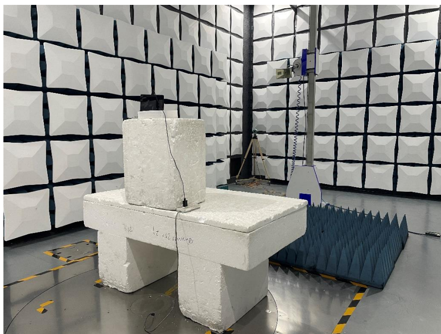
Radiated Emissions View (1GHz-18GHz)
