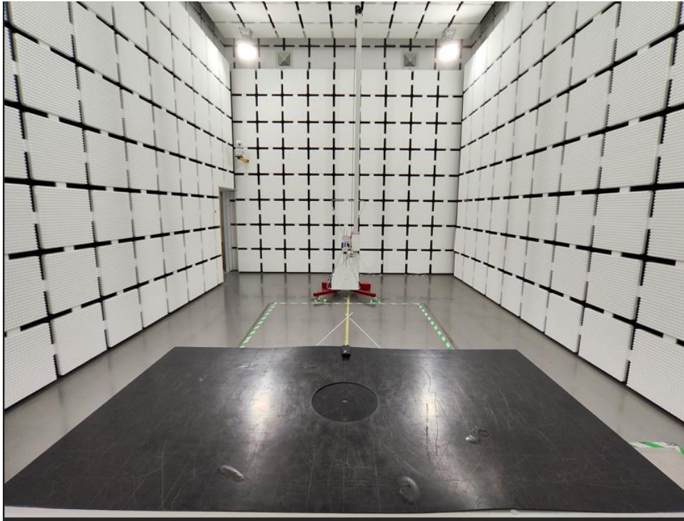
Spurious Radiation Emissions Test (<1G)
