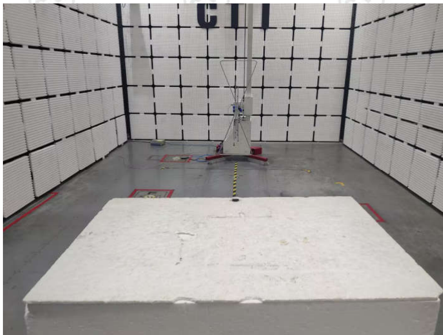
Radiated spurious emission Test Setup-1(Below 1GHz)
