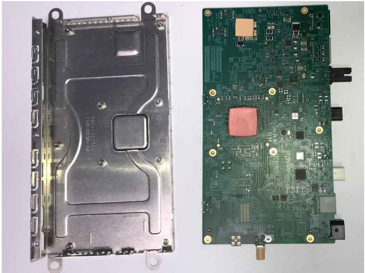
PCB Bottom & Inside Bottom Cover
