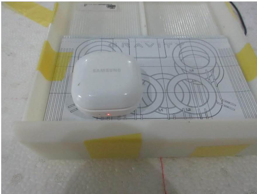
Operating Mode with charging case on Coil 6
