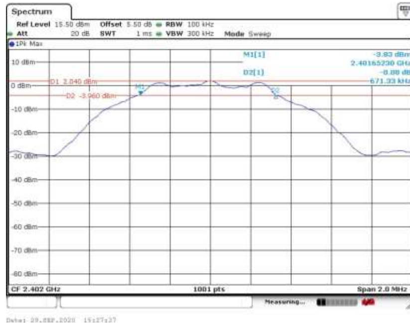
6 dB Bandwidth Plot on Channel 00
