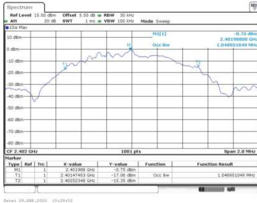
99% Bandwidth Plot on Channel 00
