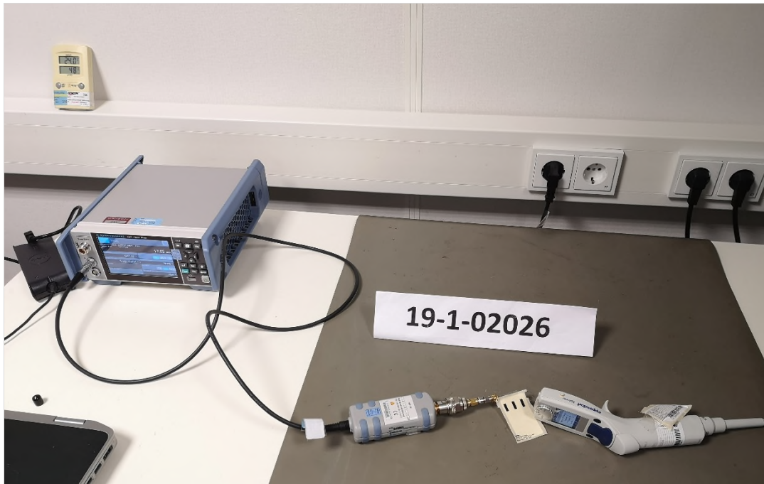
Photograph 7: Conducted Test Setup in the Radio Lab
