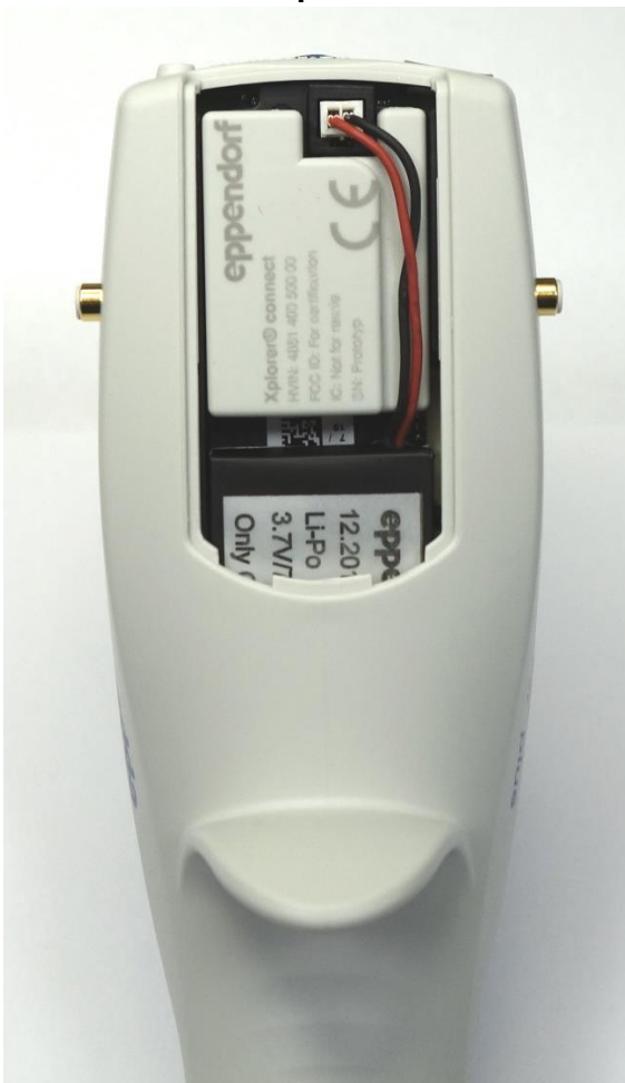
Position of Xplorer connect module in the Xplorer pipette
