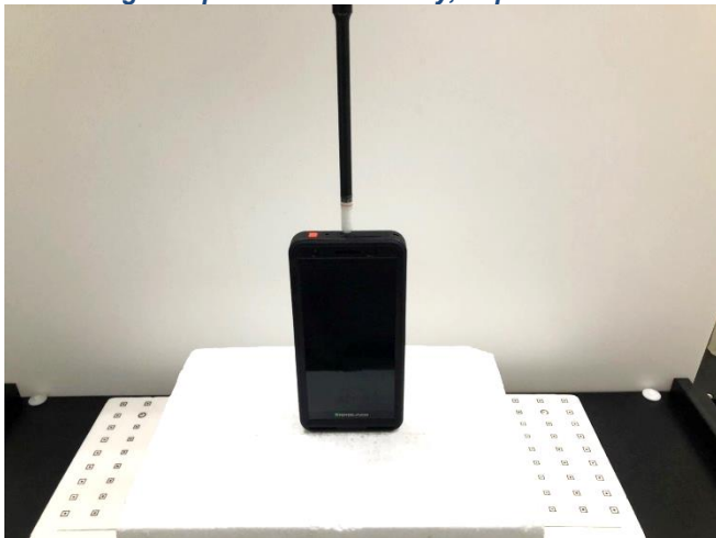
Testing Setup for Power Density, Top Side at 0 mm
