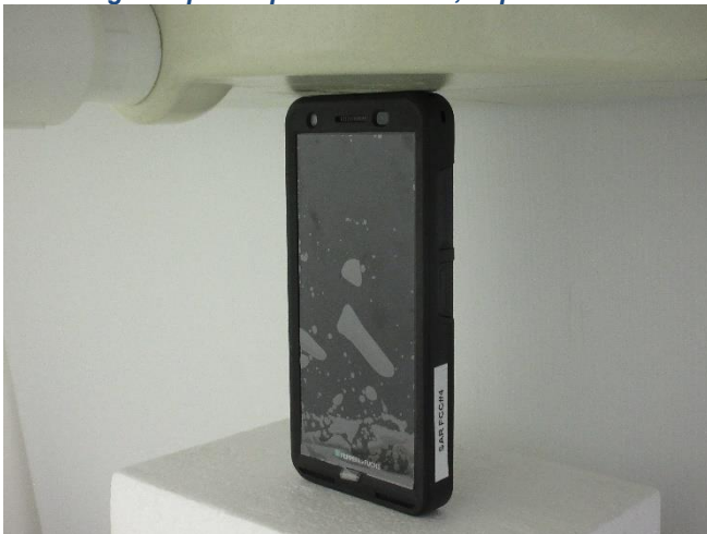
Testing Setup for Specific Phablet, Top Side at 0 mm
