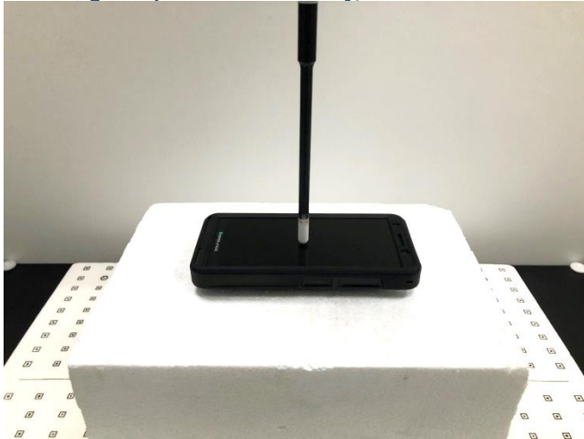
Testing Setup for Power Density, Front Face at 0 mm
