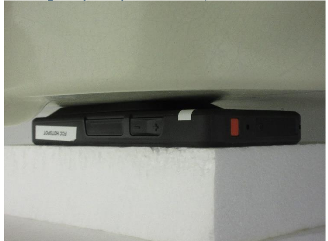
Testing Setup for Specific Phablet, Rear Face at 0 mm
