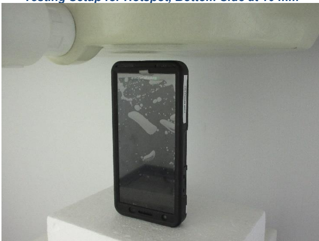
Testing Setup for Hotspot, Bottom Side at 10 mm
