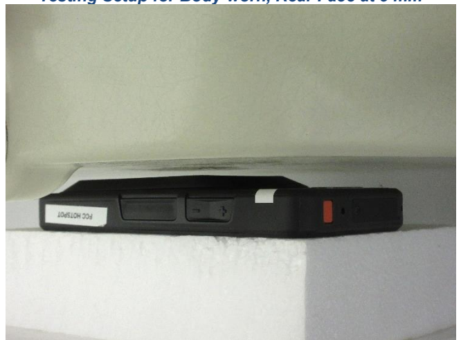
Testing Setup for Body-worn, Rear Face at 5 mm
