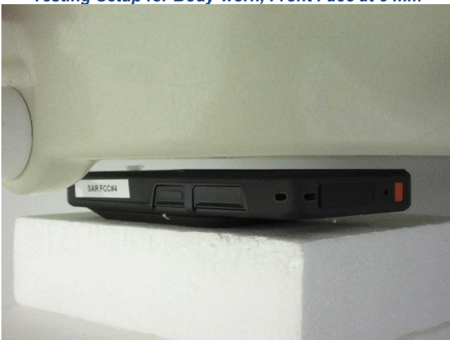
Testing Setup for Body-worn, Front Face at 5 mm
