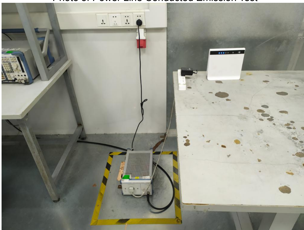
FCC ID: 2AXZ3-EAGLE Photo of Power Line Conducted Emission Test
