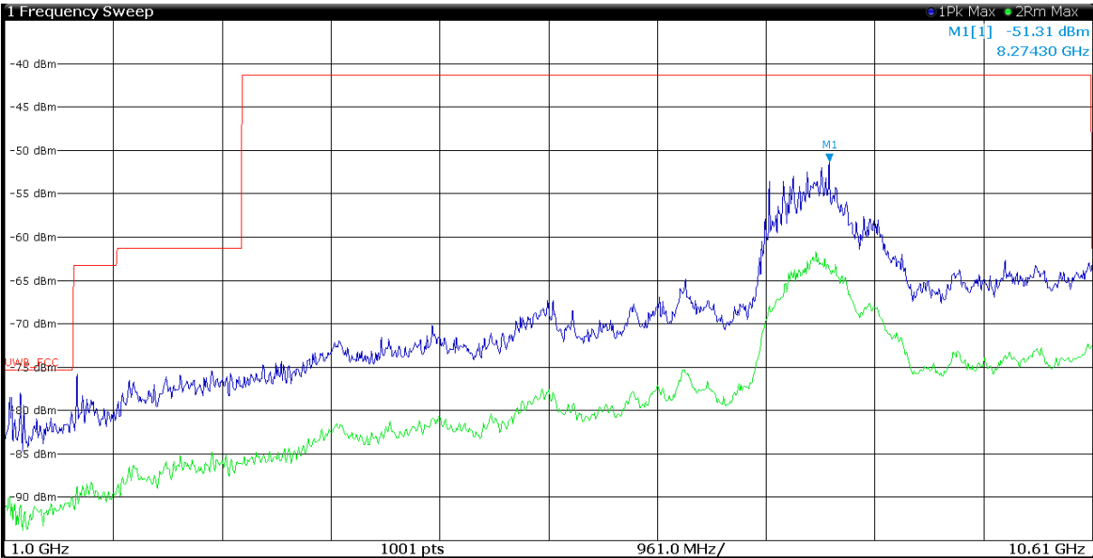
Figure 7.5-5: Radiated spurious emissions 1 to 10.61 GHz (FCC limits), with antenna in horizontal polarization
