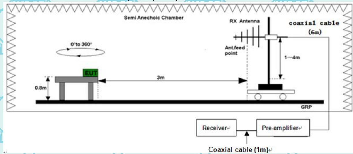
**(B) Radiated Emission Test-Up Frequency Above 1GHz**
