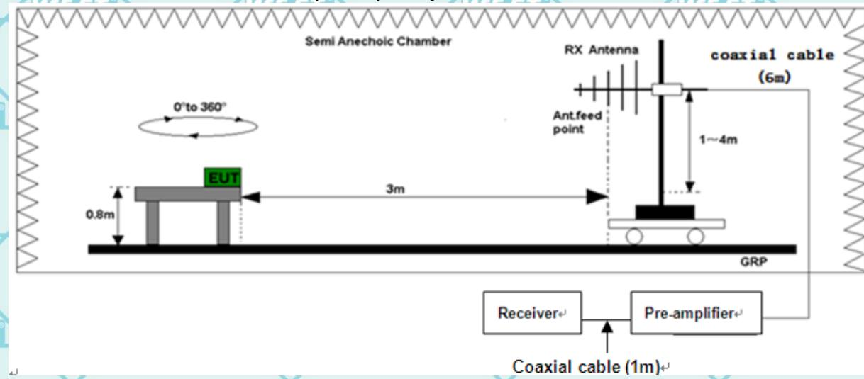
**(B) Radiated Emission Test-Up Frequency Above 1GHz**
