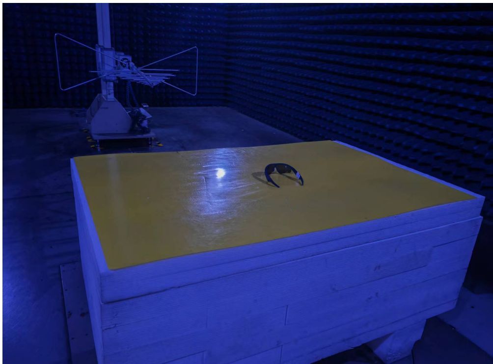
Photo of Radiated Emission Measurement (Above 1G)
