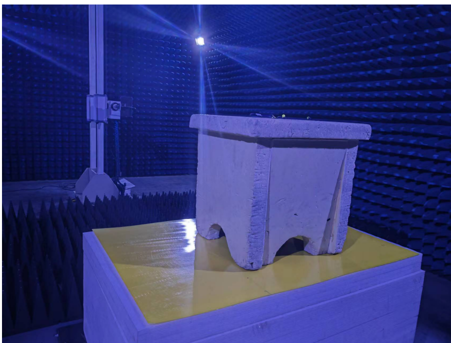
Photo of Radiated Emission Measurement (Above 1G)
